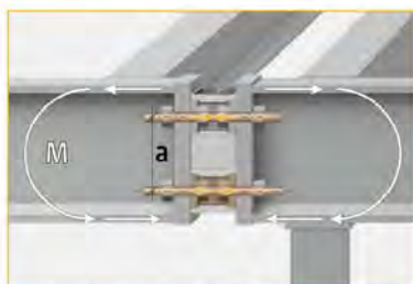
Schöck Isokorb® type S22: simplified diagram of moment load resistance
