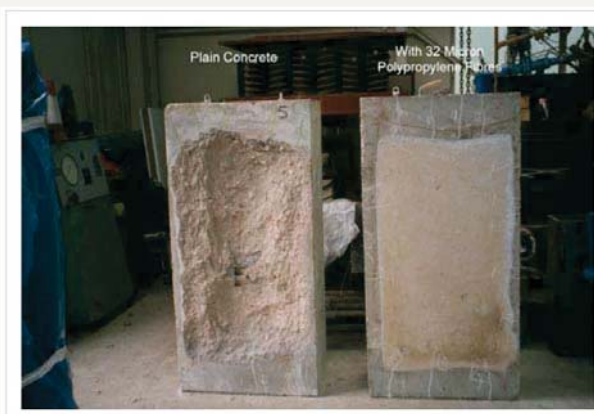
Fig. 9: Segment with 0 kg/m 3 PP-fibres (photo: MFPA Leipzig/D)
