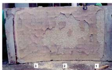
Fig. 10: Segment with 2.0 kg/m 3 PP-fibres (photo: MFPA Leipzig/D)
