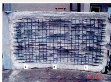
Fig. 9: Segment with 0 kg/m 3 PP-fibres (photo: MFPA Leipzig/D)
