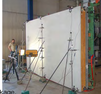
Air-pillow test setup for structural in-pane stiffness testing and front plate cracking
