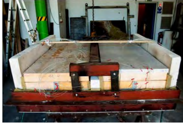
Specimens to be tested Left: insulation and structural rib Right: insulation, structural rib and front plate
