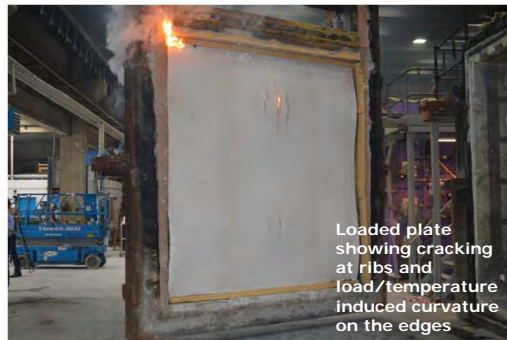
Full scale sandwich panel loaded to 50t throughout the test
