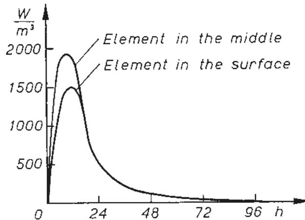
Fig. 2 The theoretical rates of heat generation per unit volume for elements being in the middle and upper surface.
