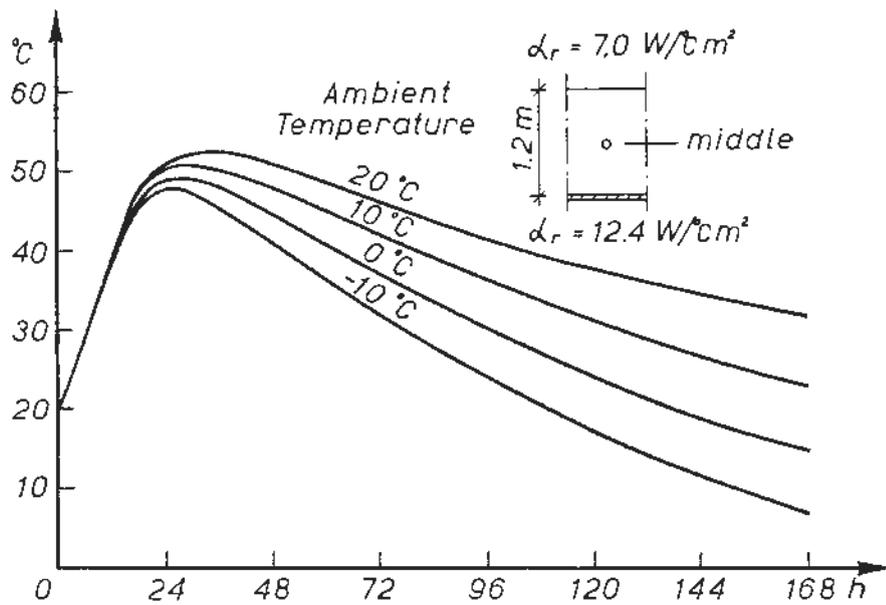
Fig. 4 Effect of outdoor temperature on the mid-point temperatures of the cross section.
