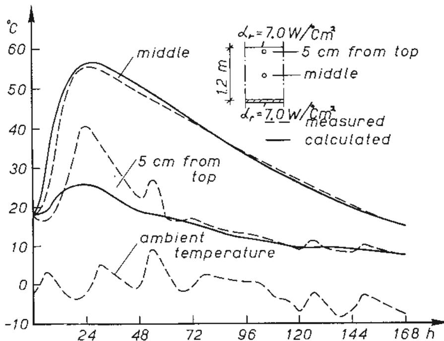
Fig. 1. Time-temperature curves measured and calculated for the 1.2 m thick bridge slab.
