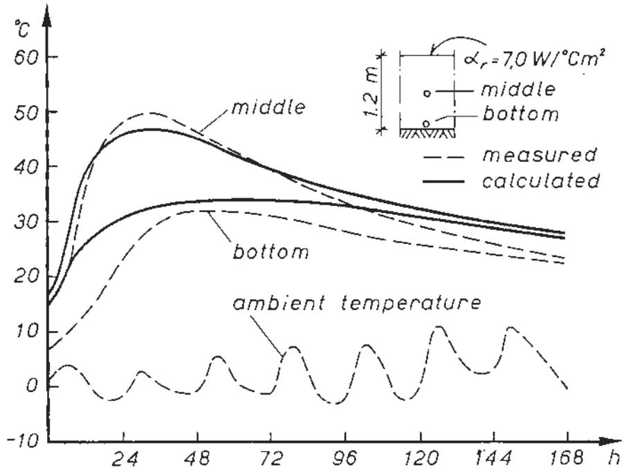
Fig. 3 Time-temperature curves measured and calculated for the 1.2 m thick base of foundation.
