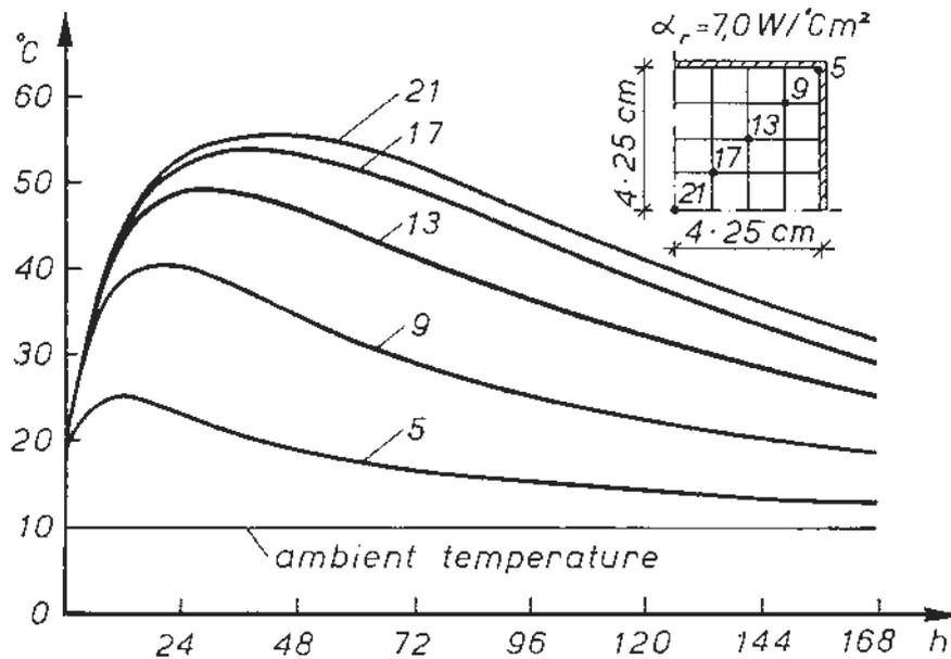
Fig. 5. The effect of two-dimensional heat flow on the temperatures at the points between the corner and mid-point of a concrete block.
