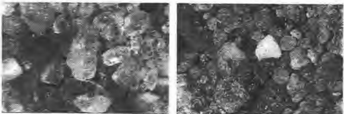
Figure 2: Photographs of artificial sand (left) and natural sand (right) of grading 4. magnification app. 4 times
