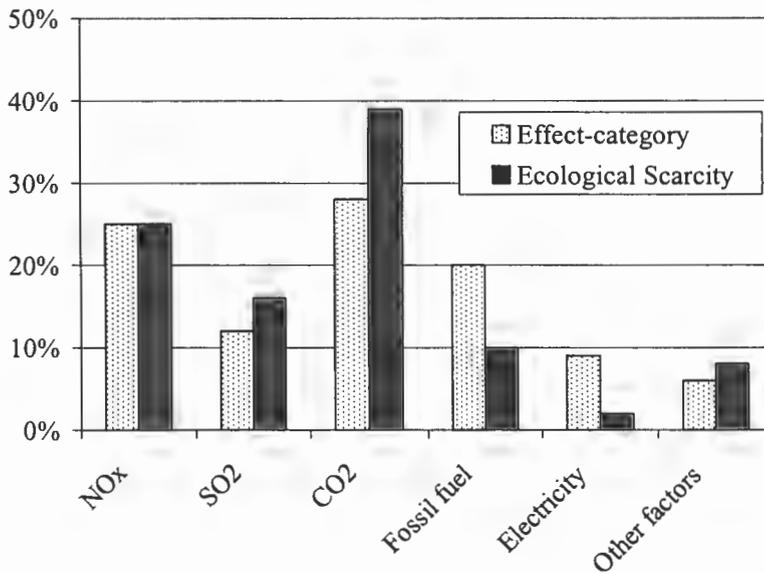
Diagram 1: Distribution of environmental loads for a hollow core slab, according to two different weighting models. Other factors include, for instance, emissions of CO, HC, heavy metals and waste.
