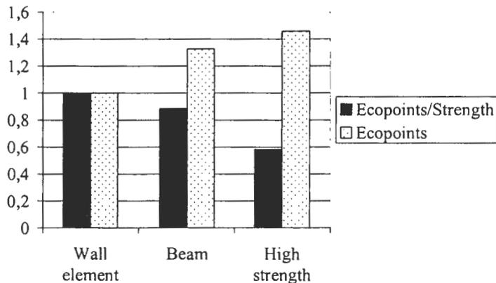
Diagram 2: Environmental load, according to the Effect-category weighting model, of three element types with and without relation to technical function.
