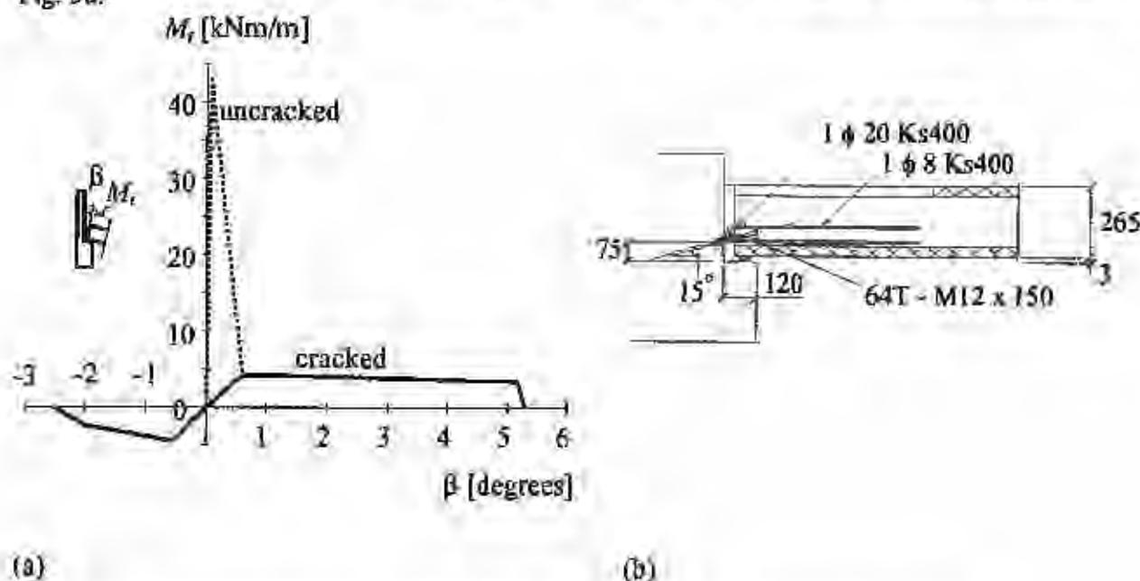
Figure 5 (a) Assumed behaviour of the beam-floor connection of ordinary type;
