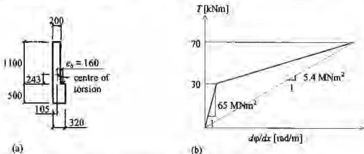
Figure 4 (a) Cross-section of the spandrel beams; (b) Assumed torsional response of the spandrel beams loaded in torsion, bending and shear.
