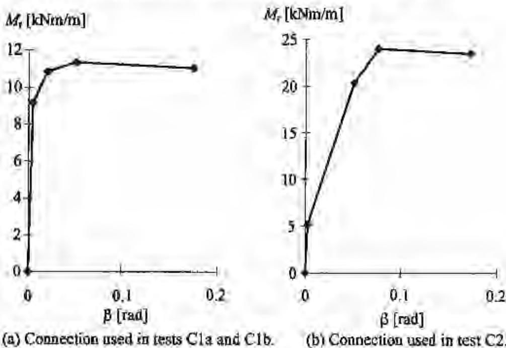
Figure 17 Estimated relationships between transferred moment  $M_r$  and rotation  $\beta$  used in the analyses.
