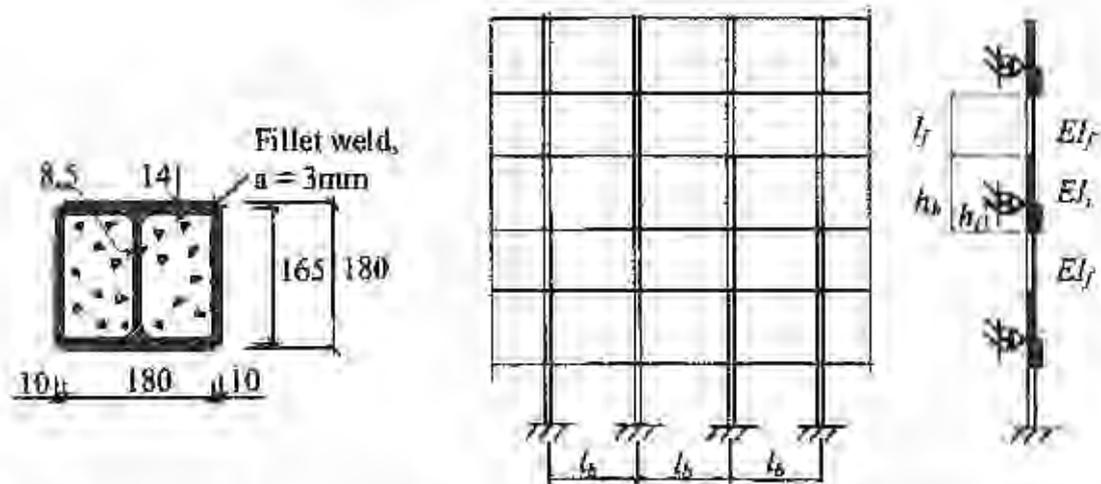
Figure 2 (a) Cross-section of columns; (b) Geometry and boundary of the façade columns.
