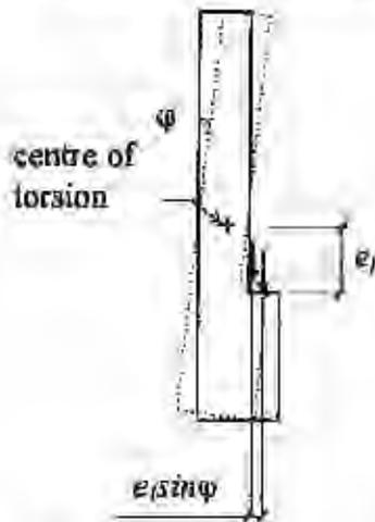
Figure 9 Reduction of the eccentricity of the vertical load from the floor, due to rotation of the beam.
