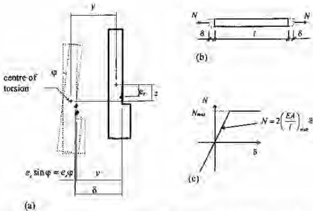
Figure 10 (a) Rotation and displacement of the cross-section; (b) Deformation of the floor; and (c) Relationship between horizontal force  $N$  and horizontal deformation  $\delta$  ( $N_{max}$  is the upper limit of the connection).
