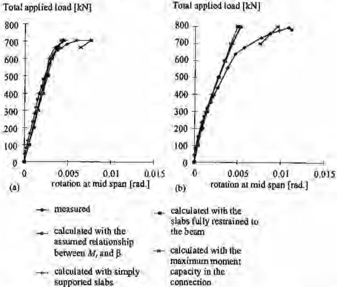
Figure 18 Total applied load versus sectional rotation at mid span in (a) test C1a; (b) test C1b.
