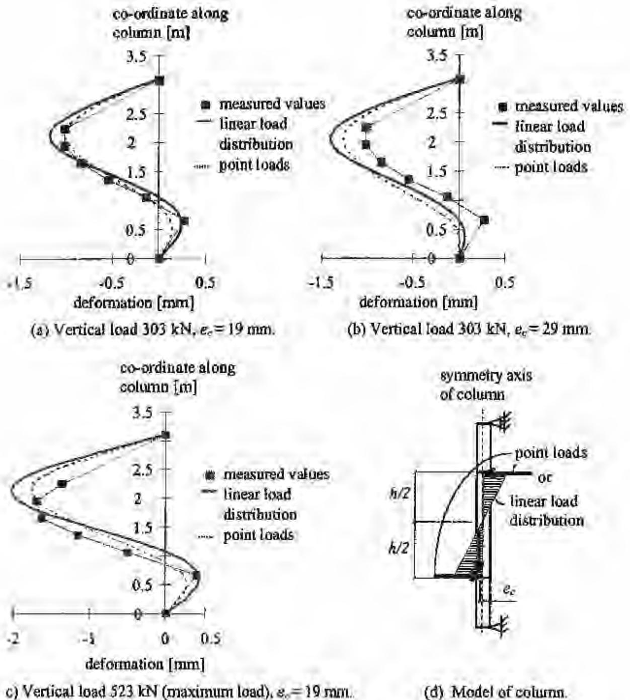
Figure 14 (a), (b) and (c) Comparison of measured and calculated deflections; (d) Model of column. Two different ways for transferring the torsional moment from the beam to the column were checked: linear load distribution and point loads.
