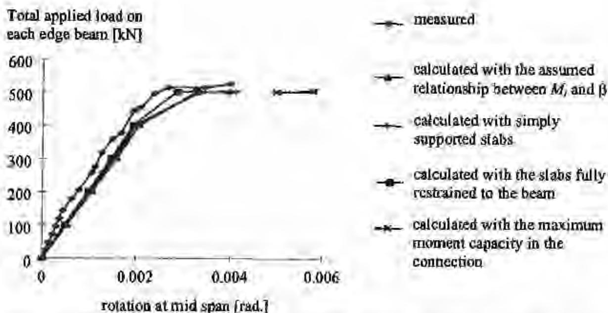
Figure 19 Total applied load on each edge beam versus sectional rotation at mid span in test CZ.
