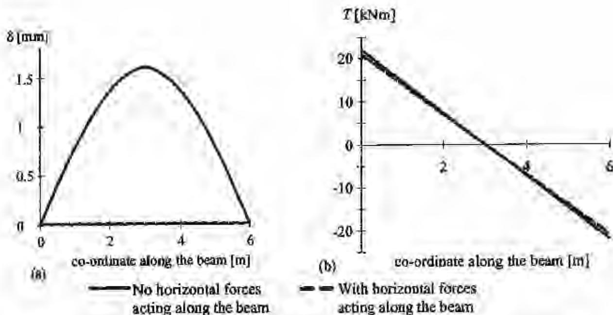
Figure 12 (a) Calculated horizontal deflection of the beam where the floor elements are connected,  $\delta$ , versus a co-ordinate along the beam (The connection is cracked); (b) Torsional moment along the beam,  $T$ , versus a co-ordinate along the beam (The connection is cracked).
