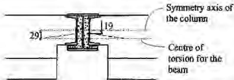
Figure 15 The centre of torsion tends to move towards the symmetry axis of the column, at the edge of the beam.
