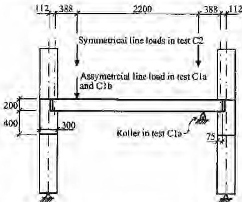
Figure 16 Principle of the test arrangement, Ref. /6/.
