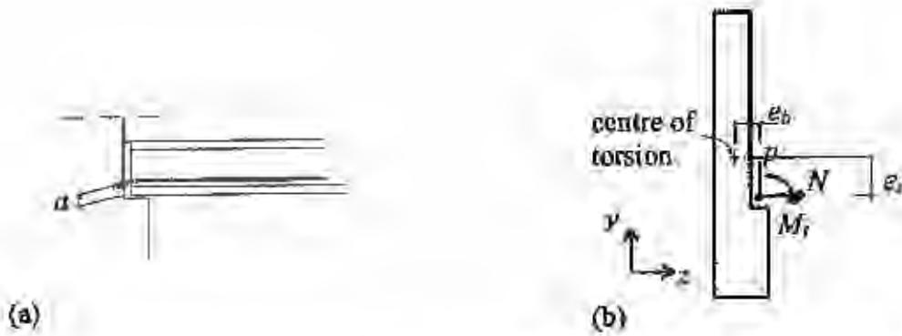
Figure 11 (a) Inner lever arm  $a$  in the connection; (b) Torsional load on the beam.
