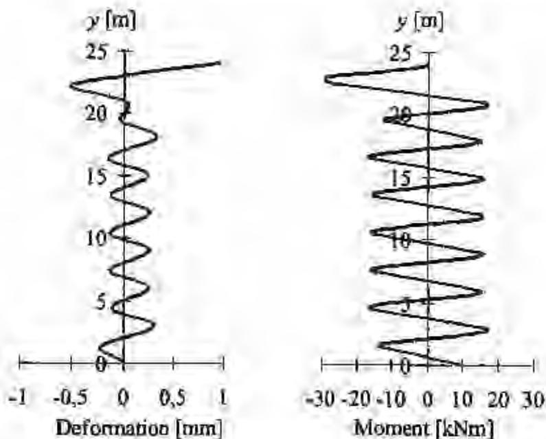
Figure 8 Deformation and bending moment along the column. In this example,  $1 \text{ kN/m}^2$  was applied on all floors, the beam-floor connections were assumed to be uncracked, and the basic input data were used for the columns. The thicker lines indicate the zones where the beams were connected.
