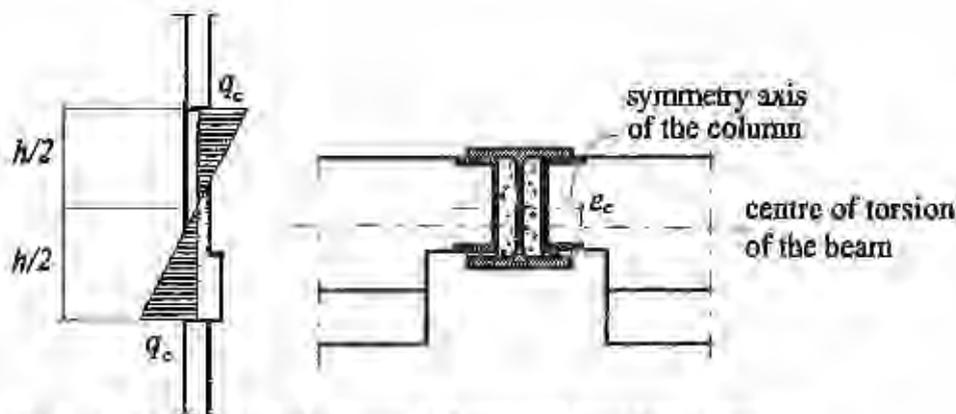
Figure 3 Connections between column and spandrel beams.
