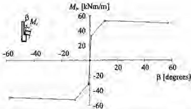
Figure 7 Assumed characteristic behaviour of the improved beam-floor connection with high deformability and ductility.
