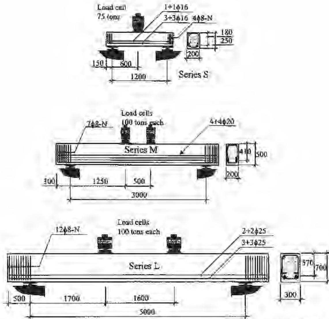
Figure 1. Load setup and geometrical configurations of test specimens in series S, M and L.
