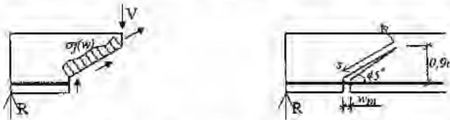
Figure 7. Basic principles for estimating the contribution of fiber concrete to the shear capacity according to Casanova [6].
