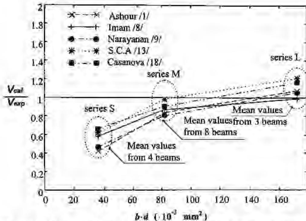
Figure 8. Ratio of calculated,  $V_{cal}$ , over experimental,  $V_{exp}$ , shear force as a function of the effective shear area,  $b \cdot d$ , for some design formulations.
