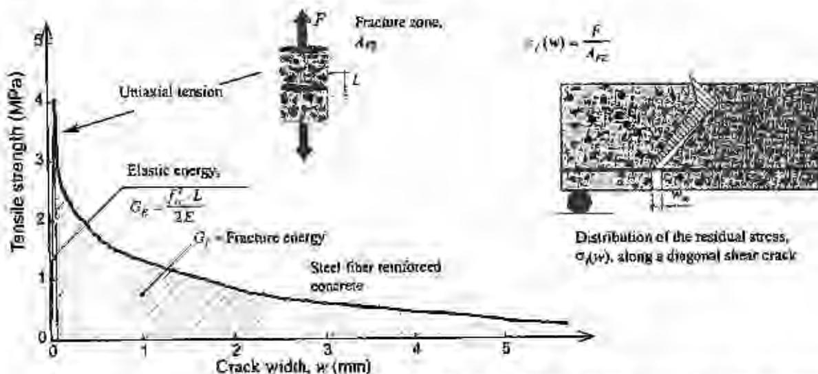
Figure 6. Comparison of stress - strain relationship for plain and fiber reinforced concrete in tension. Also, some fracture mechanical properties are shown.  $G_E$  equals the stored energy per unit area and  $G_f$  is the fracture energy per unit area.
