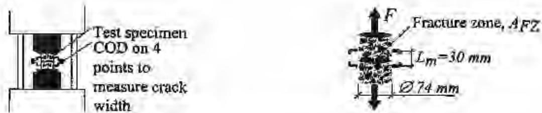
**Figure 2. Illustration of the testing device for the uniaxial tensile tests and a specimen for the uniaxial tensile tests.**
