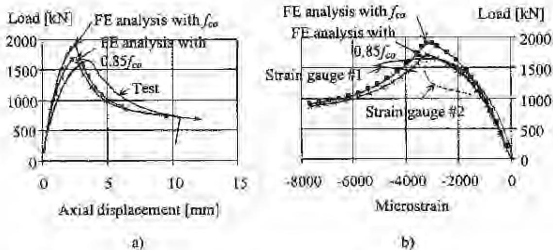
Figure 6 Column no. 2, test results and results of FE analyses: a) Load versus axial displacement curves, and b) Load-vertical strain relations. The figure includes two curves from the FE analysis, one using the cylinder strength and the other  $0.85f_{co}$ .
