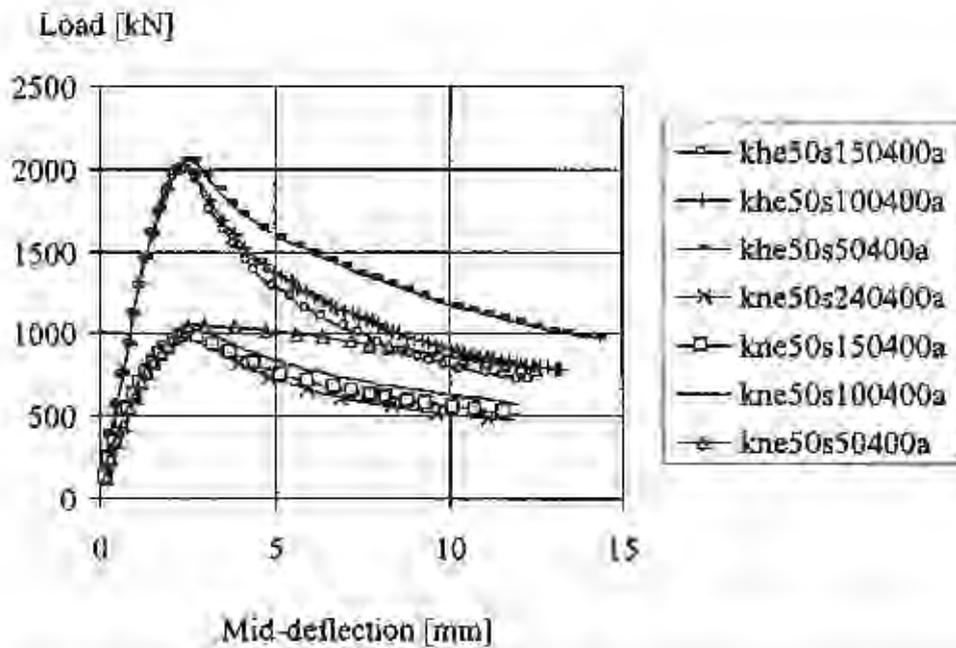
Figure 12 Load deflection relations for cross-sections with reinforcement configuration A and constant stirrup yield strength (400 MPa) subjected to eccentric loading. The stirrup spacing is varied.
