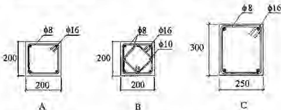
Figure 1 Concrete columns: geometry and details of configurations A, B and C.
