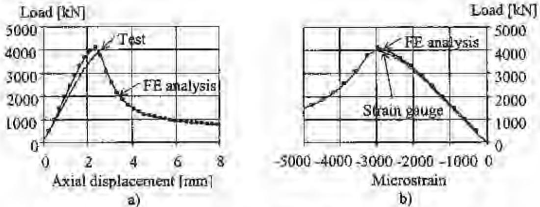
Figure 5 Column no. 1, test results and results of FE analyses: a) Load versus axial displacement curves, and b) Load-vertical strain relations.
