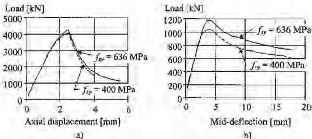
Figure 8 Load-displacement relations for cross-sections with reinforcement configuration A subjected to: a) pure compression, and b) a load eccentricity of 90 mm.
