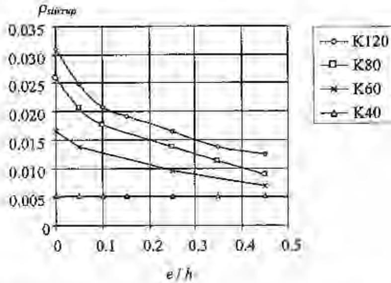
Figure 17 Required volumetric stirrup ratio versus eccentricity-to-width ratio for four different concrete strengths.
