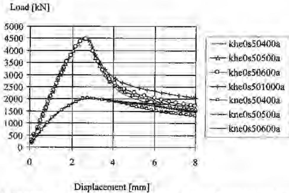
Figure 9 Load displacement relations for cross-sections with reinforcement configuration A and stirrup spacings of 50 mm subjected to pure compression. The yield strength of the stirrups is varied.
