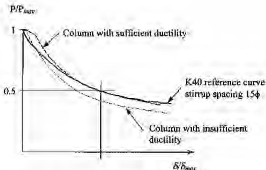
Figure 16 Illustration of a method to determine whether the column of higher strength concrete has sufficient ductility; the reference curve strength is of grade K40 and the stirrup spacing is  $15\phi$ .
