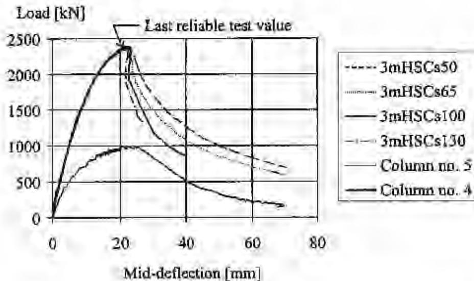
Figure 15 Load deflection relations for a 3 m high-strength concrete column with different stirrup spacings.
