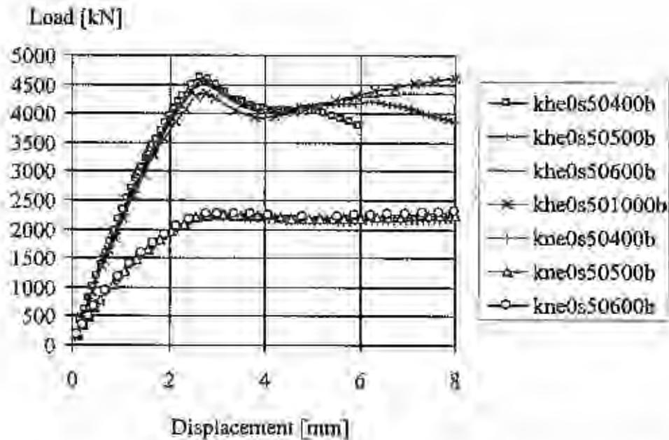
Figure 10 Load displacement relations for cross-sections with reinforcement configuration B and constant stirrup spacings of 50 mm subjected to pure compression. The yield strength of the stirrups is varied.
