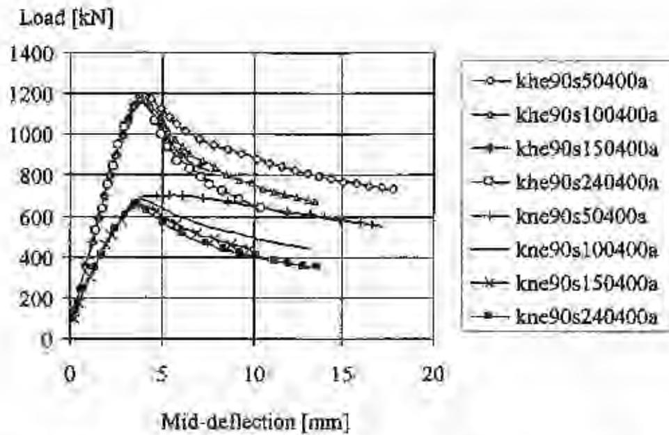
Figure 13 Load deflection relations for cross-sections with reinforcement configuration A and constant stirrup yield strength (400 MPa) subjected to eccentric loading. The stirrup spacing is varied.
