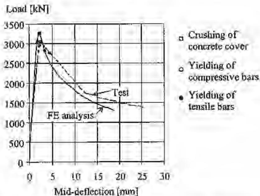
Figure 7 Load versus mid-deflection for high-strength concrete column no. 3 subjected to a load eccentricity of 90 mm.
