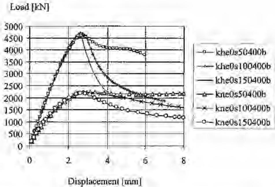
Figure 11 Load displacement relations for cross-sections with reinforcement configuration B and constant stirrup yield strength (400 MPa) subjected to pure compression. The stirrup spacing is varied.
