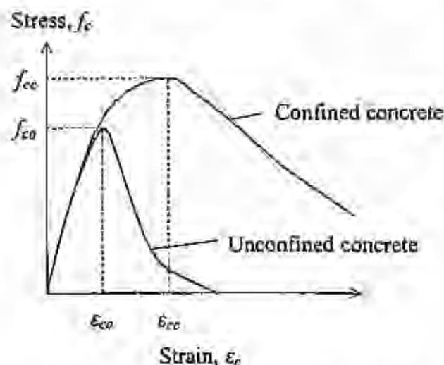
Figure 2 Stress-strain curves for confined and unconfined concrete
