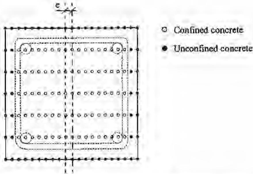
Figure 4 Confined and unconfined integration points in a beam cross-section
