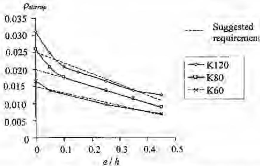
Figure 18 Suggested stirrup volume requirement for different concrete strengths.
