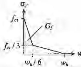
Figure 3 Stress-crack opening relation for the fracture zone.
