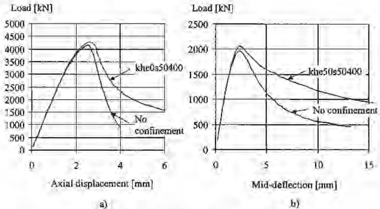
Figure 14 Effect of confinement: a) pure compression, b) eccentricity 50 mm.
