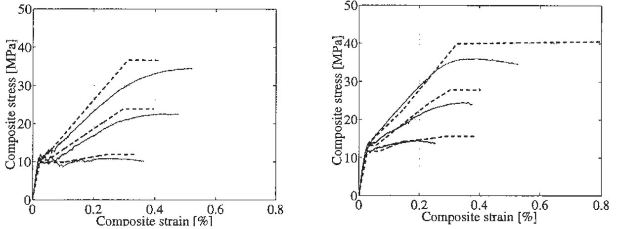
**Figure 10:** Measured (—), and simulated (---) responses for  $V_f = 3\%$  (left) and  $V_f = 6\%$  (right).
