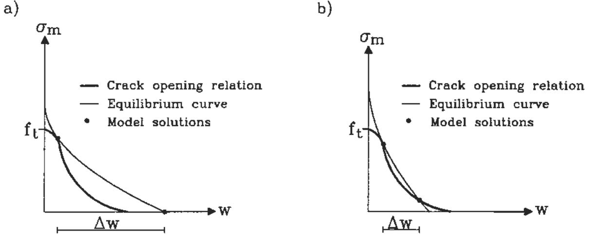
**Figure 6:** *Illustration of uncontrolled crack development for the case of 6.a: a weak reinforcement and 6.b: a relatively strong reinforcement.*
