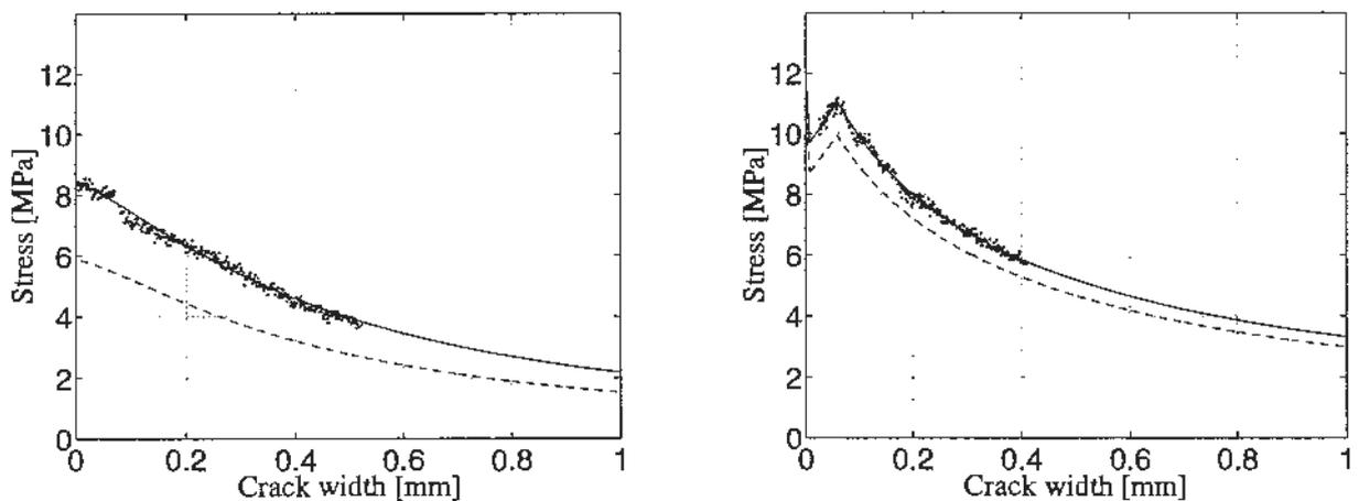
Figure 9: Measured (· · ·), estimated (—) and simulated (---) crack opening relations for  $V_f = 3\%$  (left) and  $V_f = 6\%$  (right).
