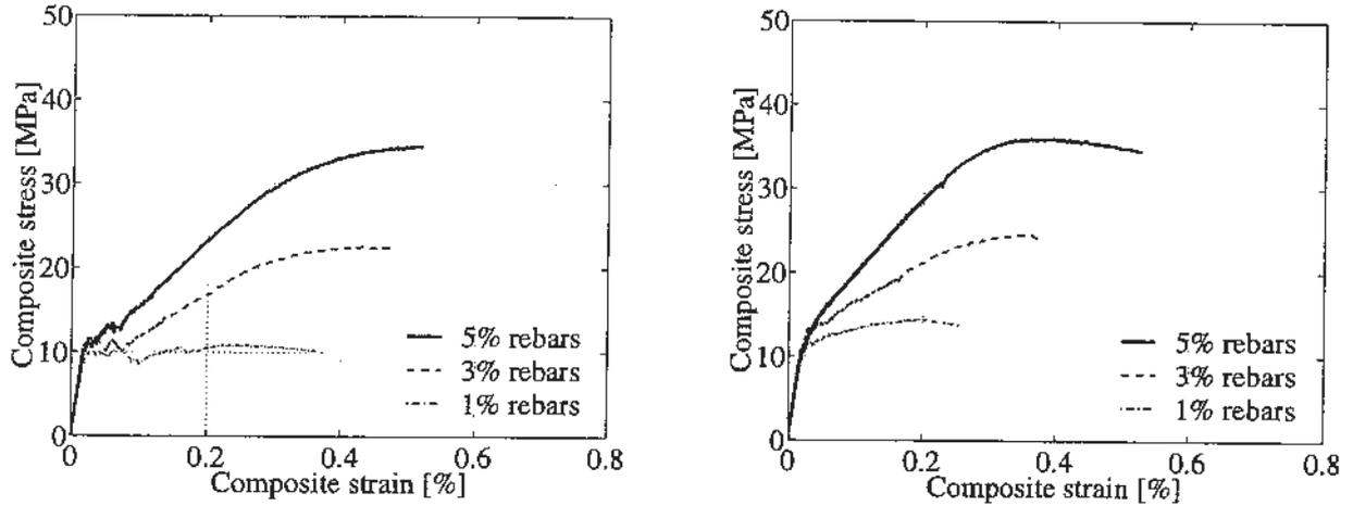
Figure 4: Measured responses in uniaxial tension for  $V_f = 3\%$  (left) and  $V_f = 6\%$  (right).
