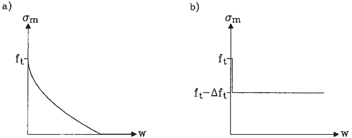
**Figure 7:** *Idealized crack opening relations. 7.a: Parabolic crack opening relation. 7.b: Constant crack opening relation with an initial spike due to the sub-matrix contribution*
