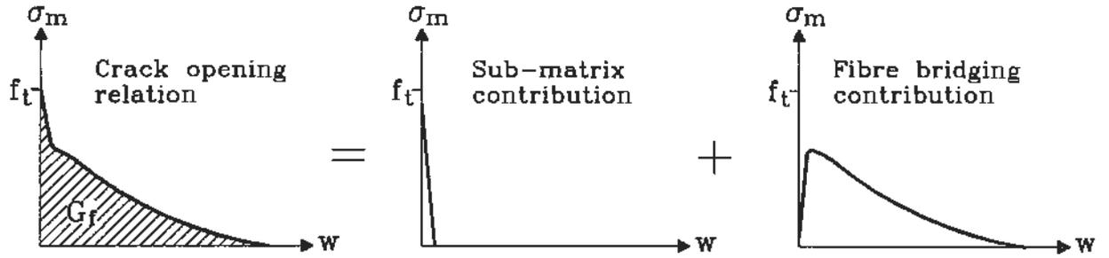
**Figure 1:** *Illustration of typical crack opening relation for a fibre reinforced matrix.*
