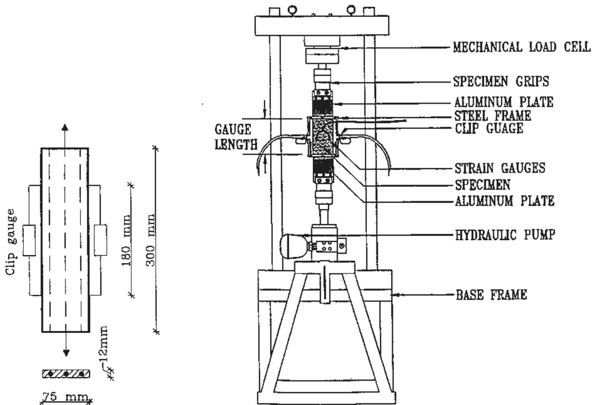
Figure 2: Specimen and test setup.
