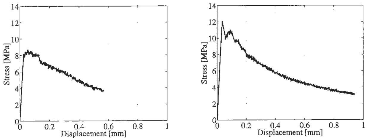
**Figure 3:** Measured responses in uniaxial tension for the matrix materials. Left: Response for  $V_f = 3\%$ . Right: Response for  $V_f = 6\%$ .
