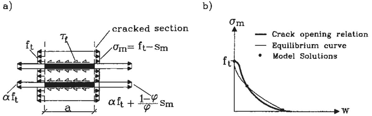
**Figure 5:** Illustration of 5.a: the stress distribution at initial cracking and 5.b: the model solutions at initial cracking.
