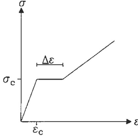
Figure 8: Definition of plastic strain  $\Delta\epsilon$  due to initial yielding.
