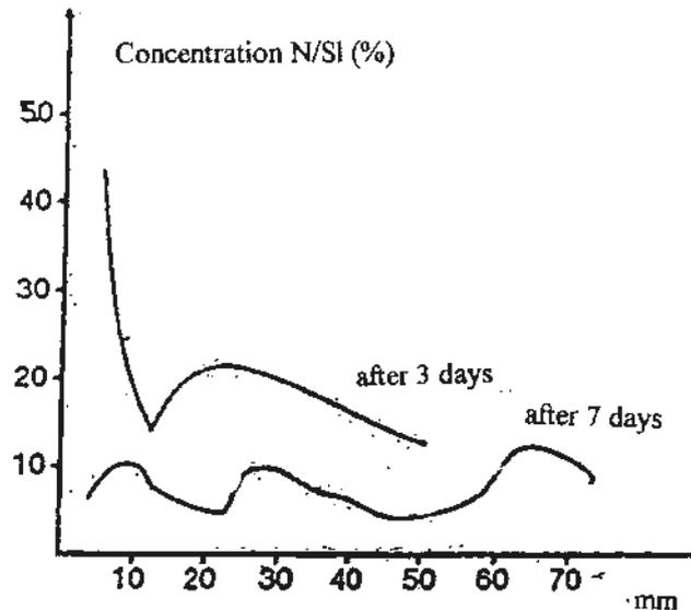
**Figure 5.** Transport studies of inhibitor in concrete blocks (application face at top)
