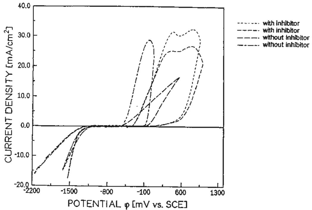
Figure 3. Potentiodynamic polarisation of mild steel /4/
