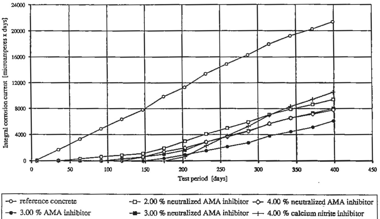
**Figure 4.** Integral corrosion currents /7/
