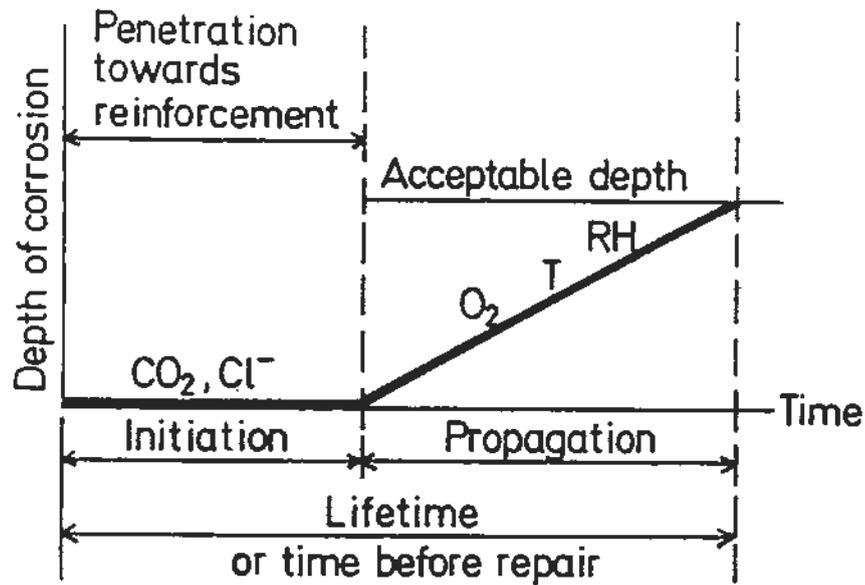
**Figure 1.** Illustration of steel corrosion in concrete /1/
