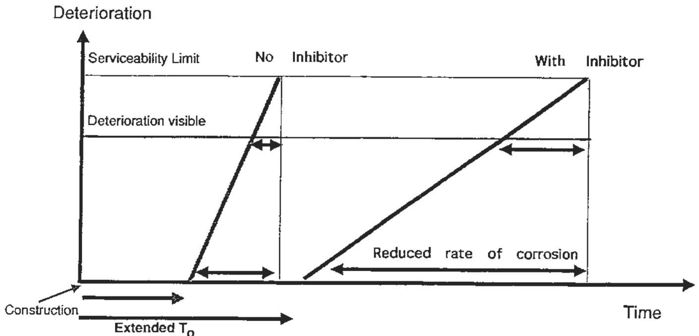
**Figure 2.** Extension of the service life of a concrete structure with corrosion inhibitor /5/
