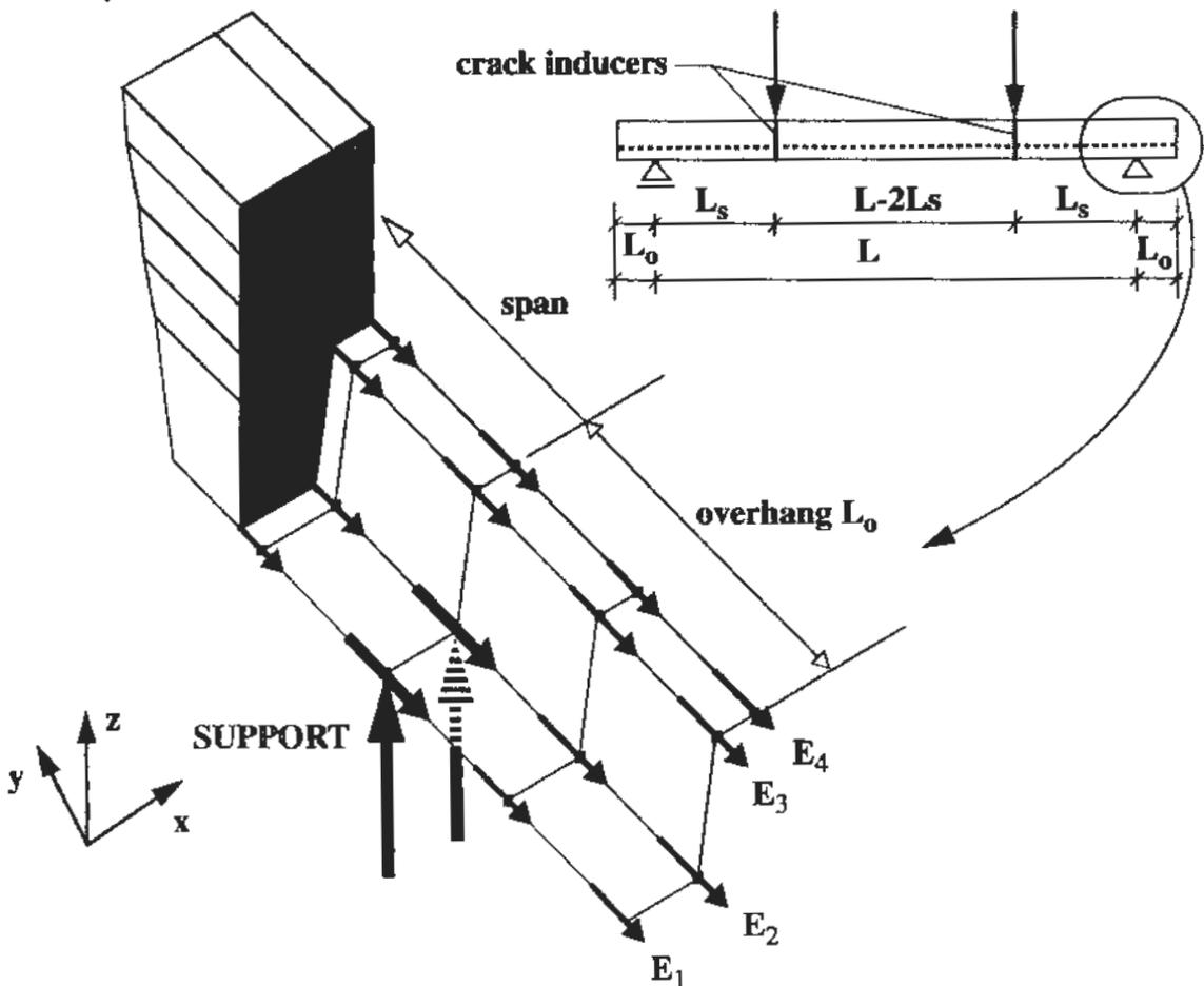
Figure 6. Model of the longitudinal interaction between sheeting and concrete
