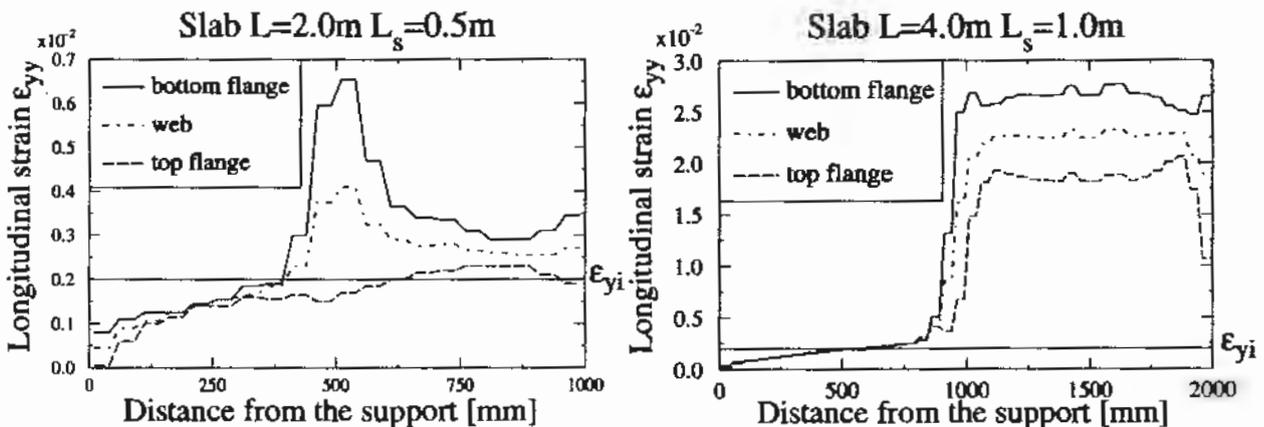
Figure 14. Strain distribution in the sheeting at maximum load
