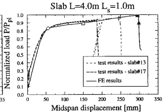
Figure 10. Load-displacement diagram for slab failing in flexure
