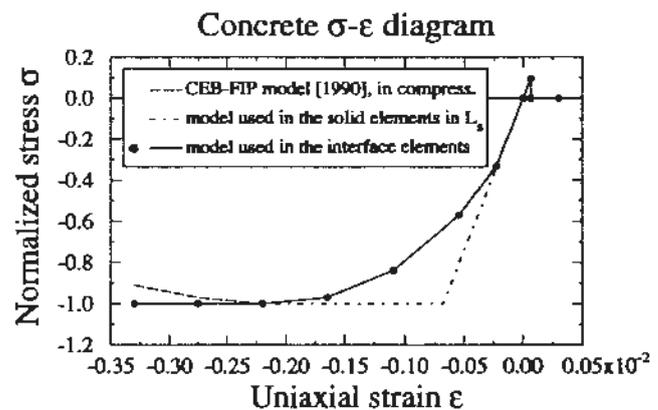
Figure 8. Basic uniaxial  $\sigma$ - $\epsilon$  relation for concrete
