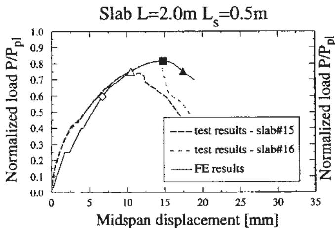
Figure 9. Load-displacement diagram for slab failing in longitudinal shear
