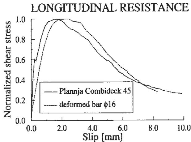
Figure 1. Comparison of push test for sheeting /6/ and the pull-out test of reinforcement /16/, /17/
