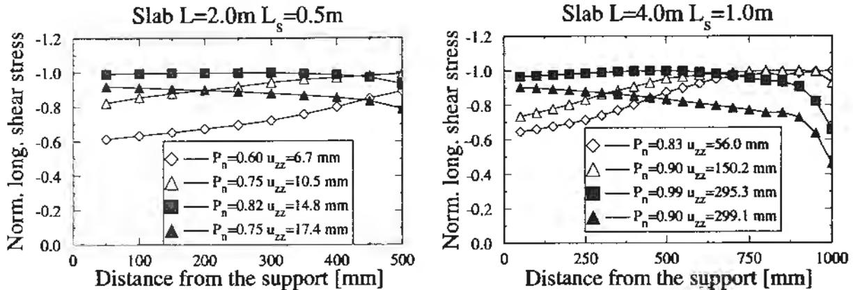
Figure 12. Longitudinal shear stress distribution at the bottom flange in the shear spans for slabs failing in longitudinal shear and flexure
