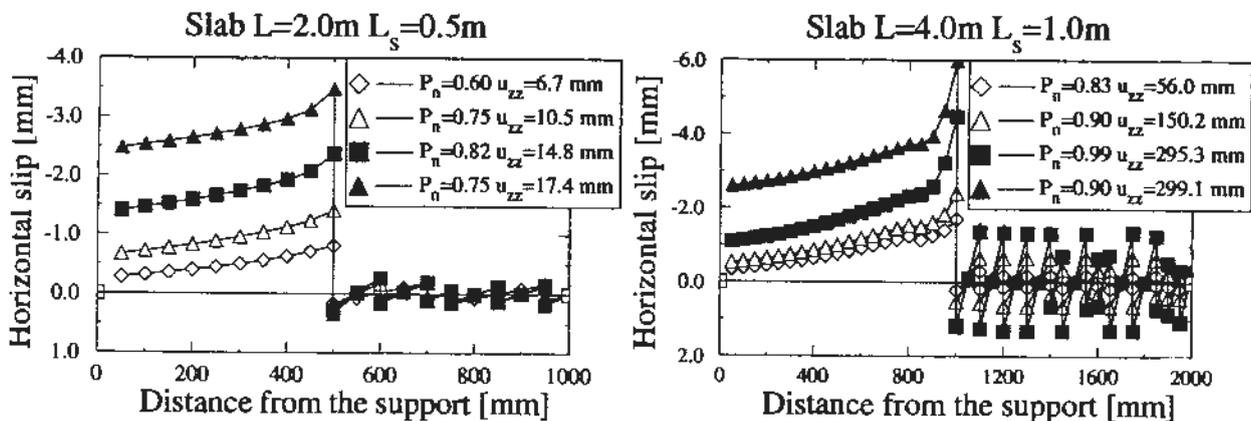
Figure 11. Slip between the concrete deck and the sheeting at different load levels
