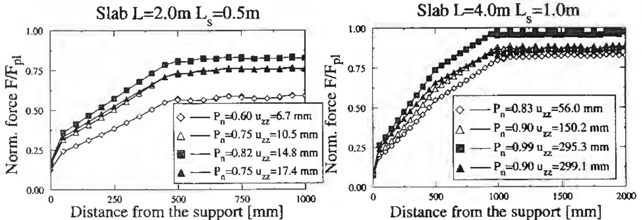
Figure 13. Cumulative force in the sheeting at the maximum load
