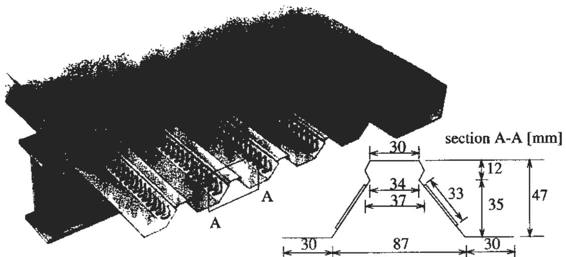
Figure 2. Plannja Combideck composite floor, courtesy of Plannja AB Luleå
