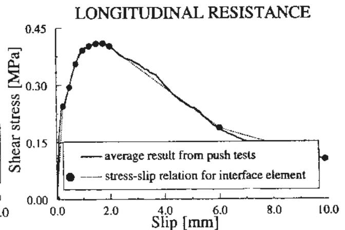
Figure 5. Sheeting shear stress-slip diagram
