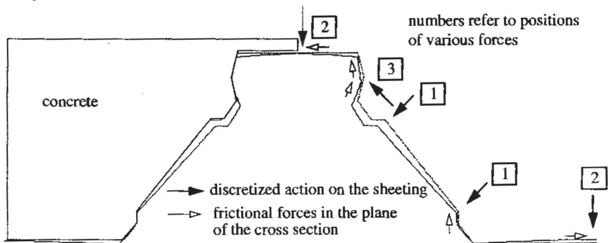
Figure 3. Bending of sheeting during concrete overriding. The original and the deformed shape of the sheeting are shown.
