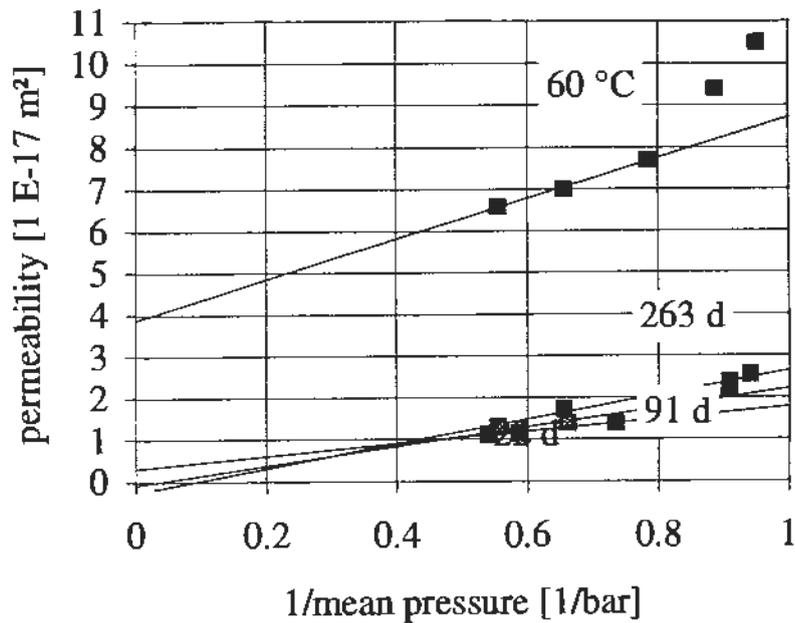
Figure: Permeability as function of the reciprocal mean gas pressure.
