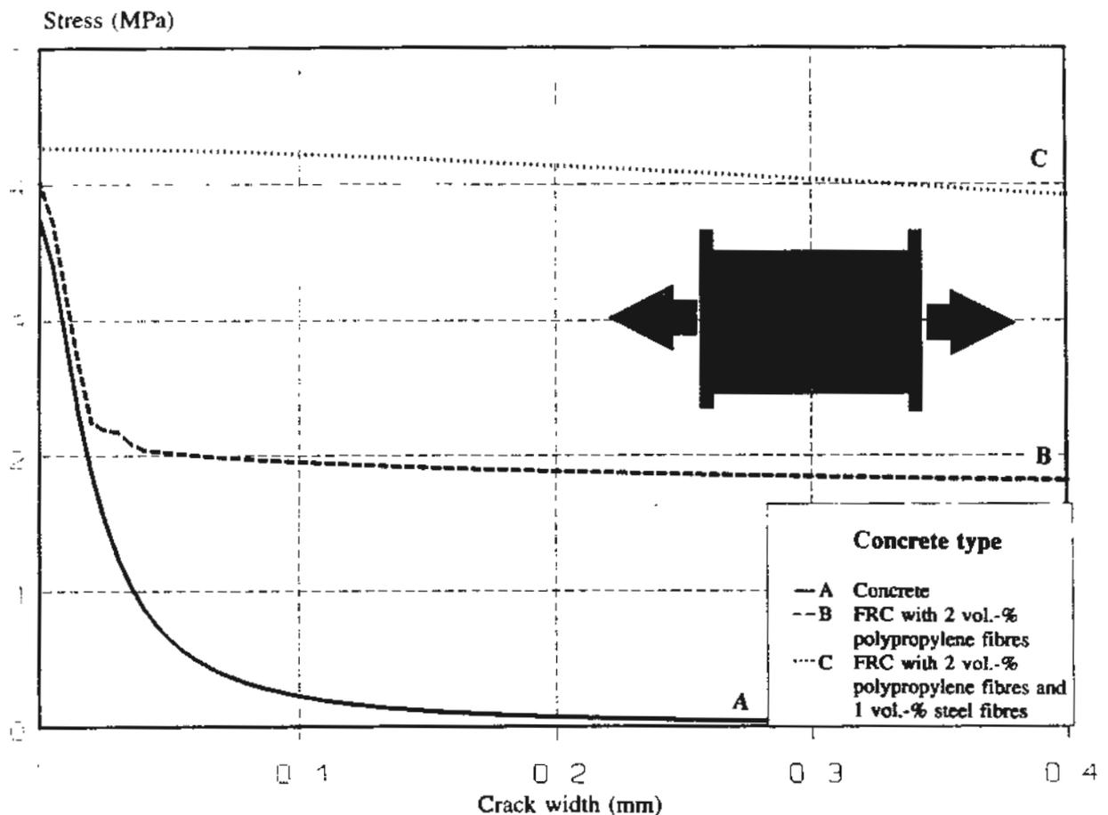
FIG. 3. Stress-crack width curves
