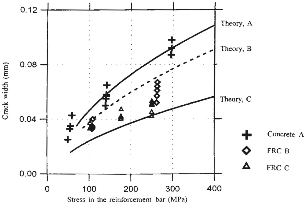
FIG. 4. Experimental and theoretical results for crack widths in the prisms.
