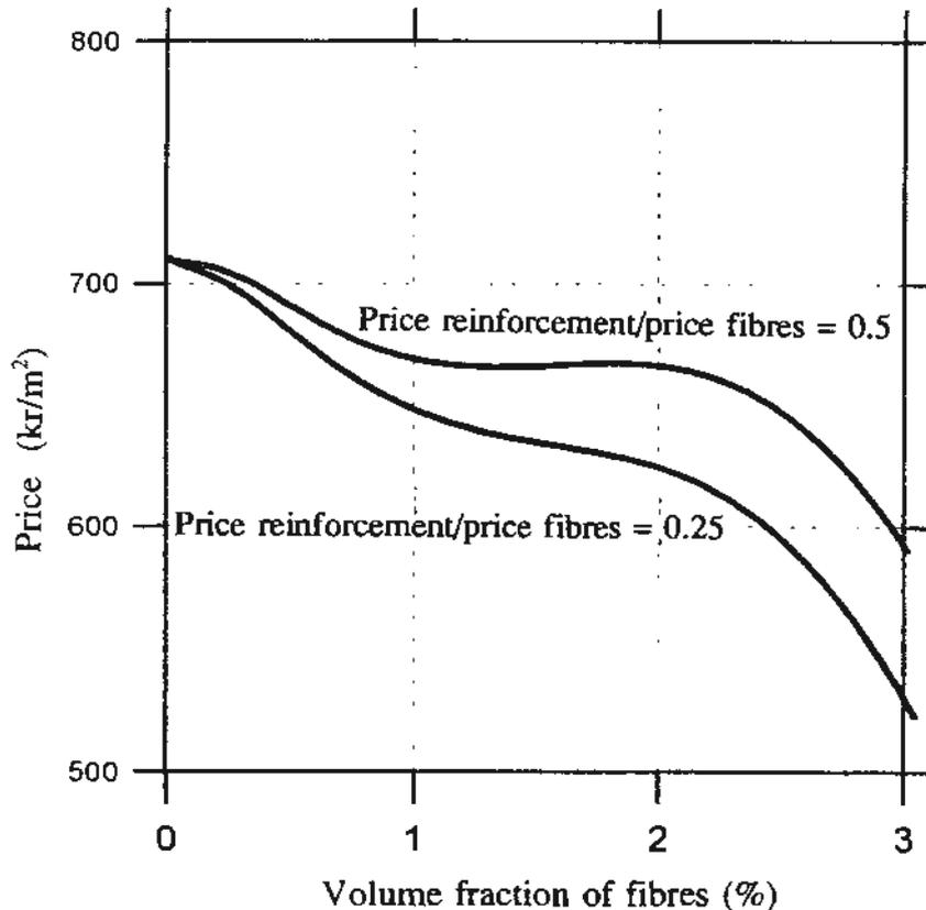
FIG. 6. Material costs (fibres and conventional reinforcement) for different volume fractions of fibres and for  $M/b=200$  kNm/m.
