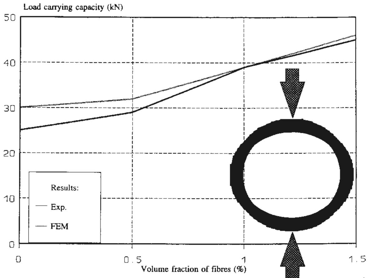
FIG. 7. Comparison between FEM calculations of - and experiments with - FRC pipes.
