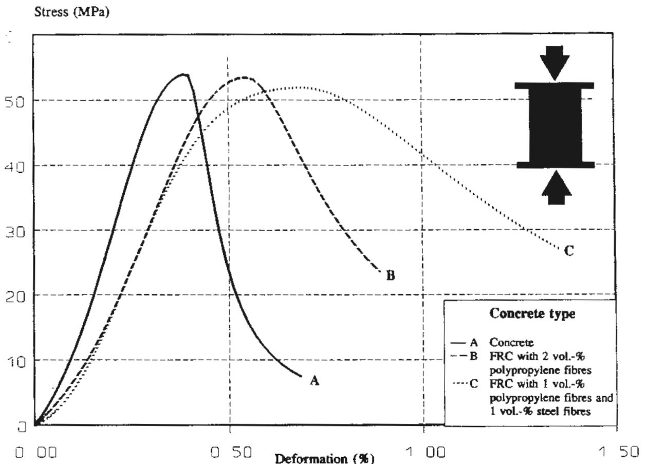
FIG.2. Compressive stress-strain curves
