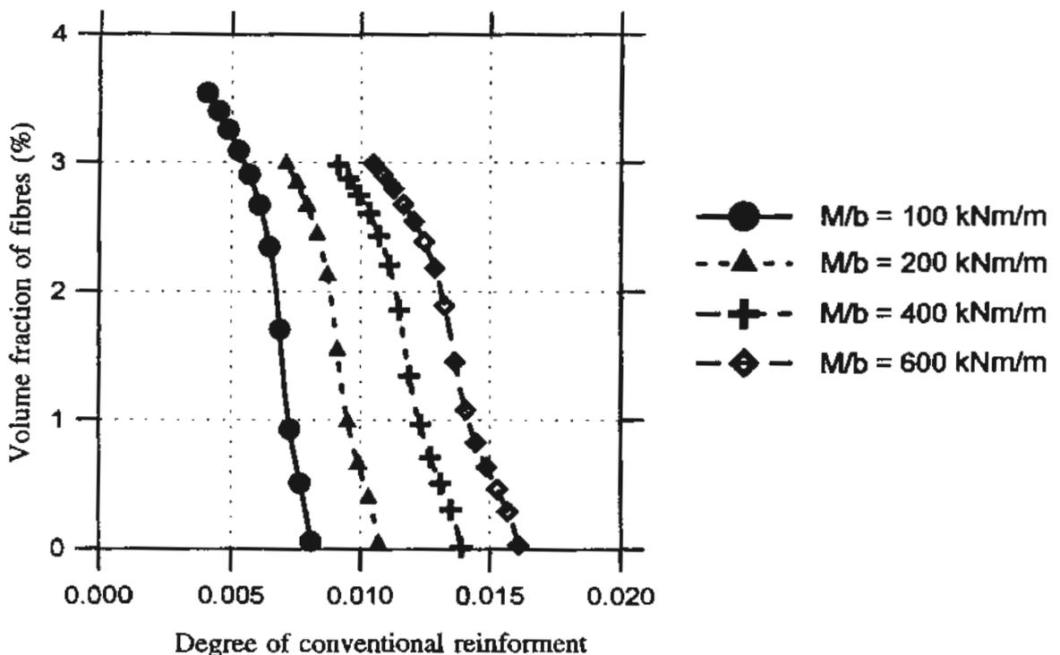
FIG. 5. Corresponding values of the volume fraction of fibres and the degree of reinforcement for a beam loaded in bending.
