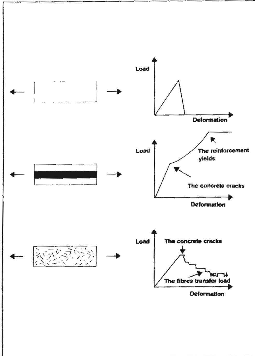
FIG. 1. *Material behaviour of unreinforced concrete, conventionally reinforced concrete and FRC*
