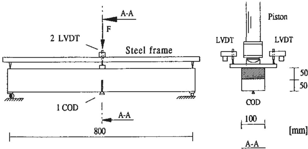
Figure 2: Test setup for the monotonic and the fatigue tests.
