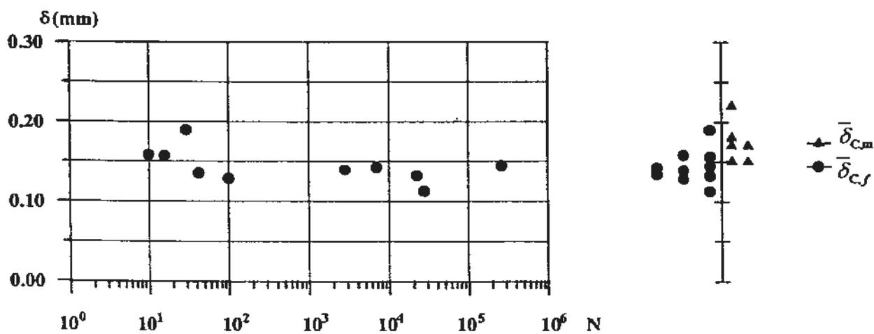
Figure 5: (left) Points representing the end of the linear section of the creep curves. (right) Distribution of deformation of the fatigue and the monotonic tests.
