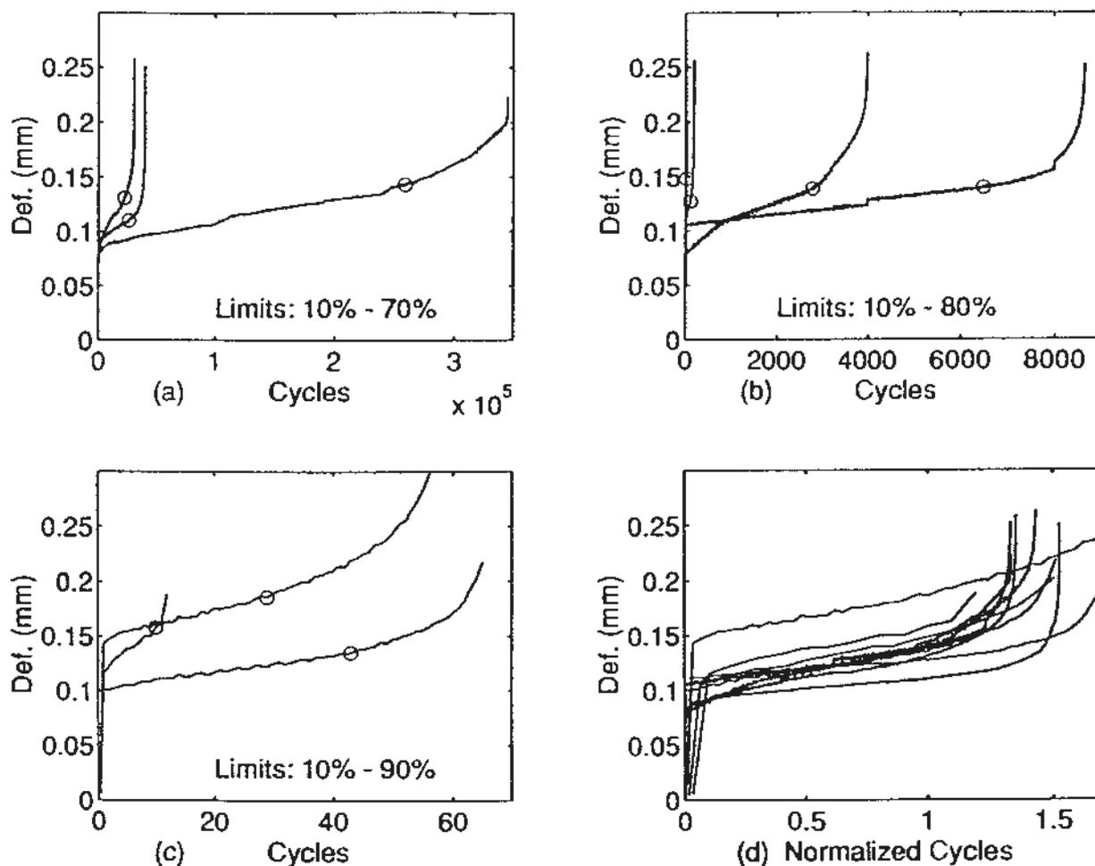
Figure 4: (a)-(c) Fatigue creep curves for the different load levels, (d) Normalized fatigue creep curves, with respect to point C, for all tests.
