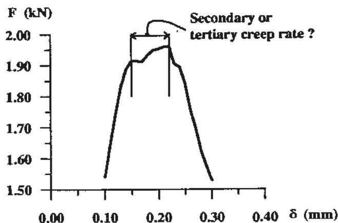
Figure 6:  $F - \delta$  curve of beam No. 5 with a plateau at the peak.
