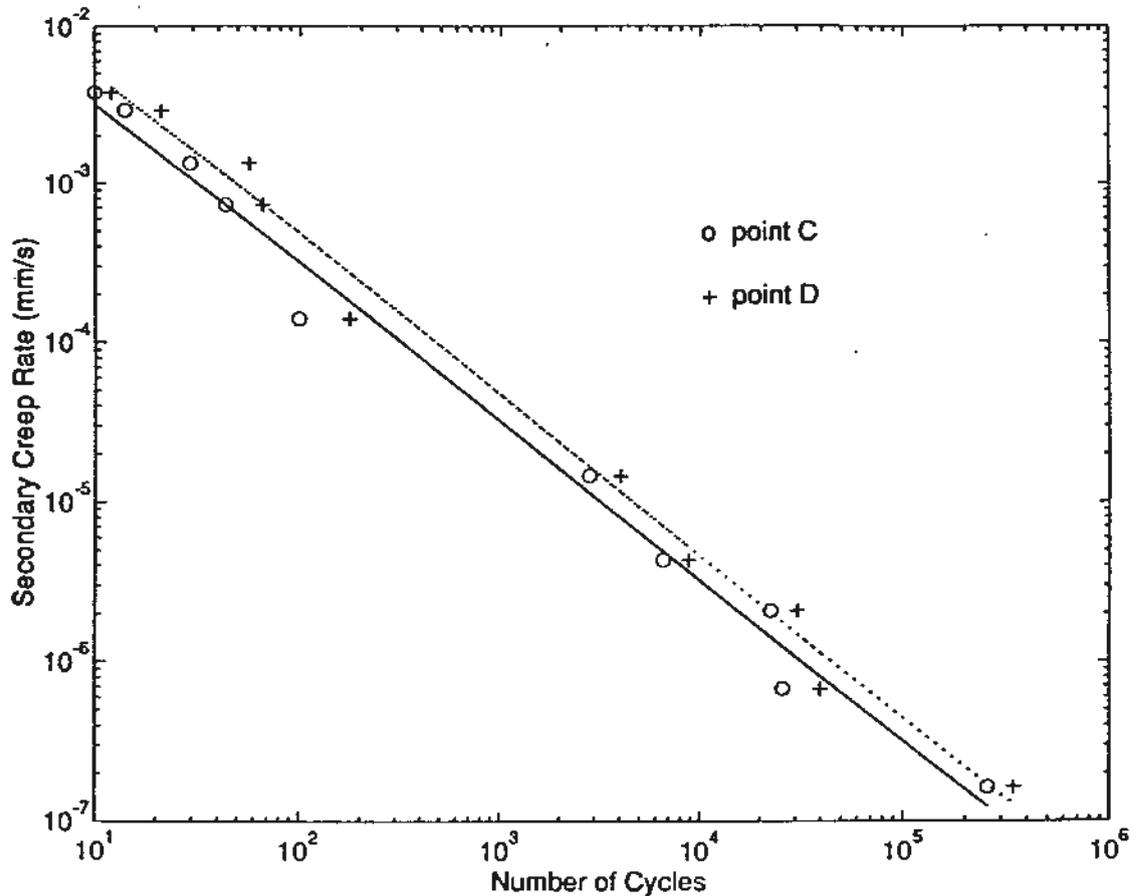
Figure 7 : Relation between fatigue creep rate  $\dot{\delta}_{sec}$  and fatigue life, defined as  $N_C$  and  $N_D$ .
