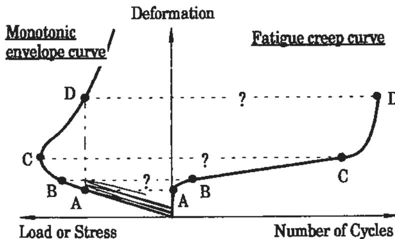
Figure 1: Schematic description of the fatigue failure hypothesis.
