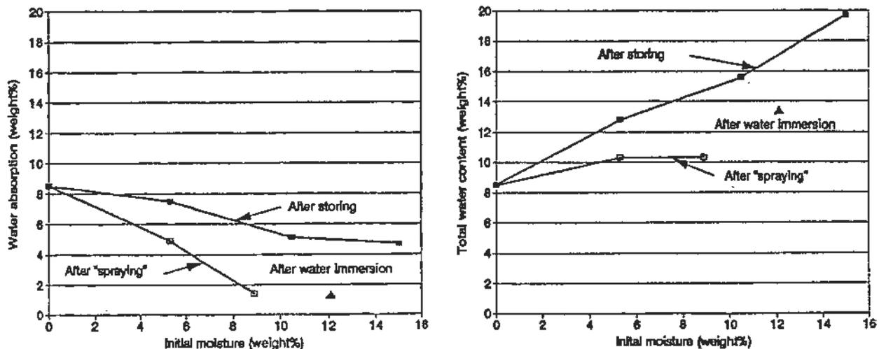
Figure 1. Effect of the initial LWA moisture on the mix water absorption (example)
