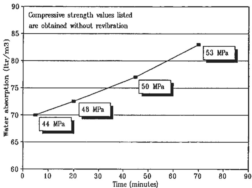
Figure 2. The mix water absorption and compressive strength as a function of time after mix water addition (example)
