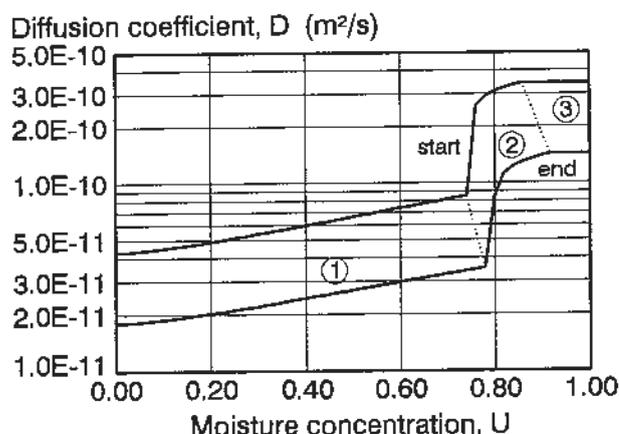
Figure 2 Example on curves showing the diffusion coefficient versus moisture concentration at the start of the 5 day, and at the end of the drying process. Mortar with  $w_0/C = 0.55$ .
