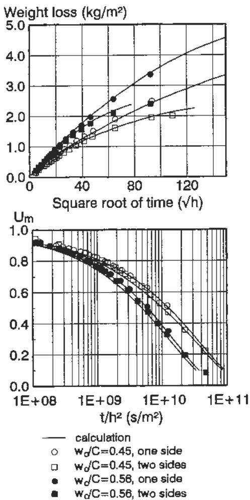
Figure 7 Influence of  $w_0/C$  ratio on drying of mortar
