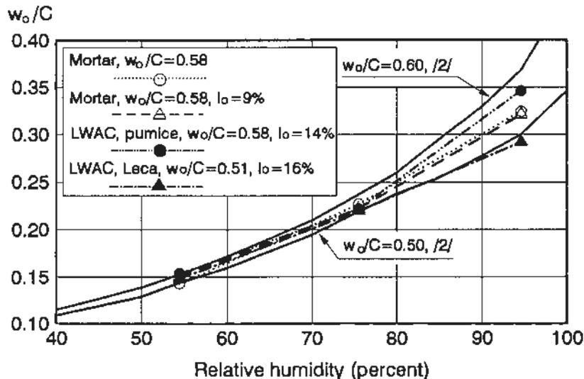
Figure 4 Desorption isotherms for 4 different types of concrete compared to curves based on literature /2/.  $l_o$ =air content
