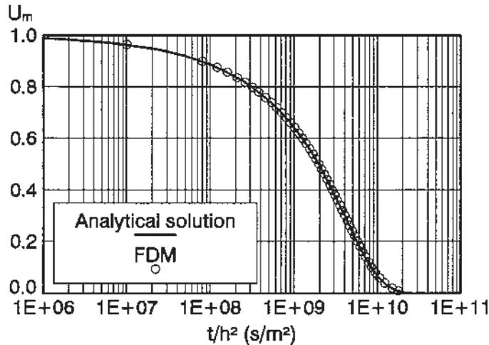
Figure 5 Drying course with constant diffusion coefficient. Comparison between analytical and FDM method.  $D=10^{-10} \text{ m}^2/\text{s}$
