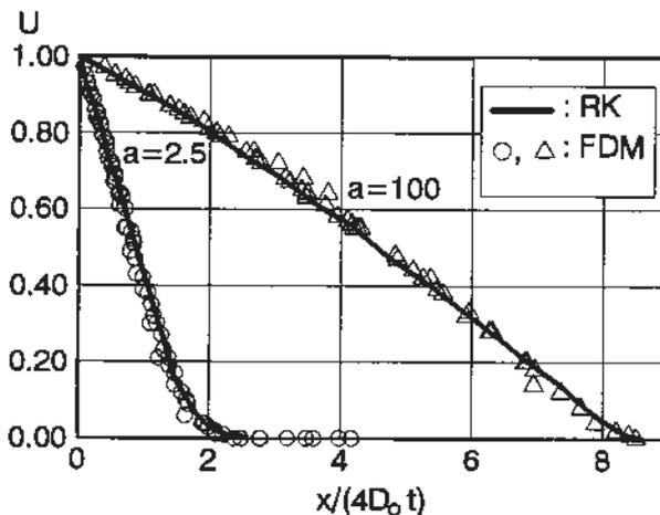
Figure 6 Concentration-distance curves according to equation (10). Numbers on curves are values of  $a$ . Comparison between FDM and Runge-Kutta (RK).
