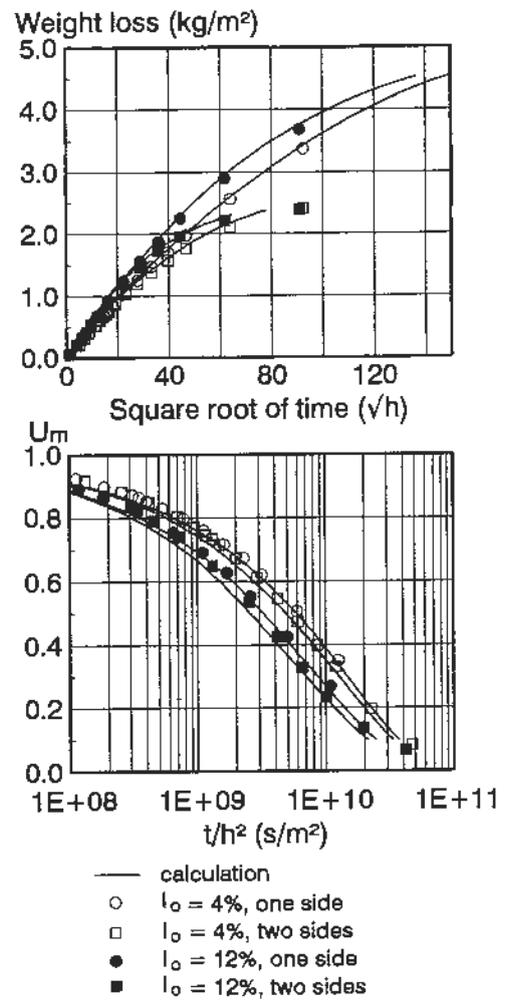
Figure 8 Influence of air content ( $l_0$ ) on drying of mortar
