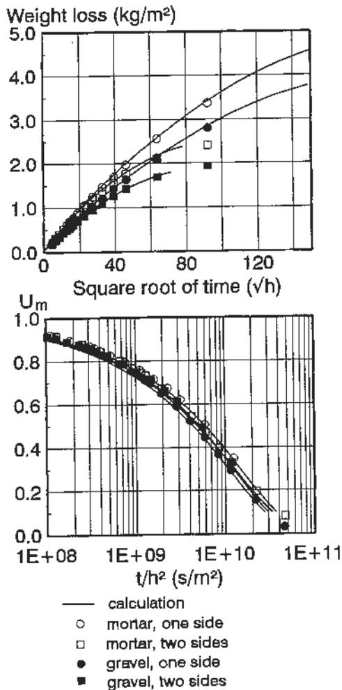
Figure 9 Influence of gravel, 26 vol-%, on drying of mortar.
