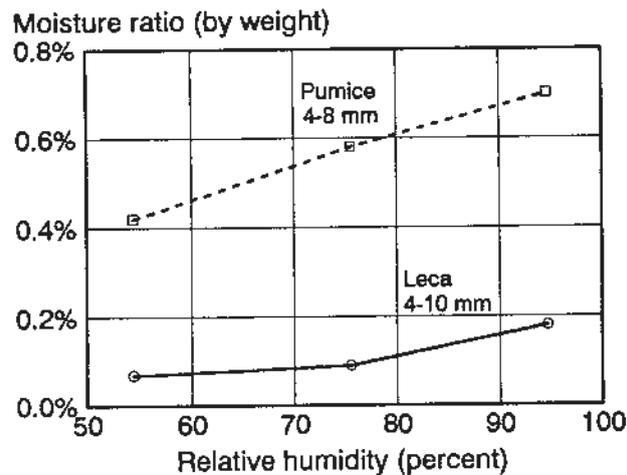
Figure 3 Desorption isotherms for lightweight aggregates used in the experiments.
