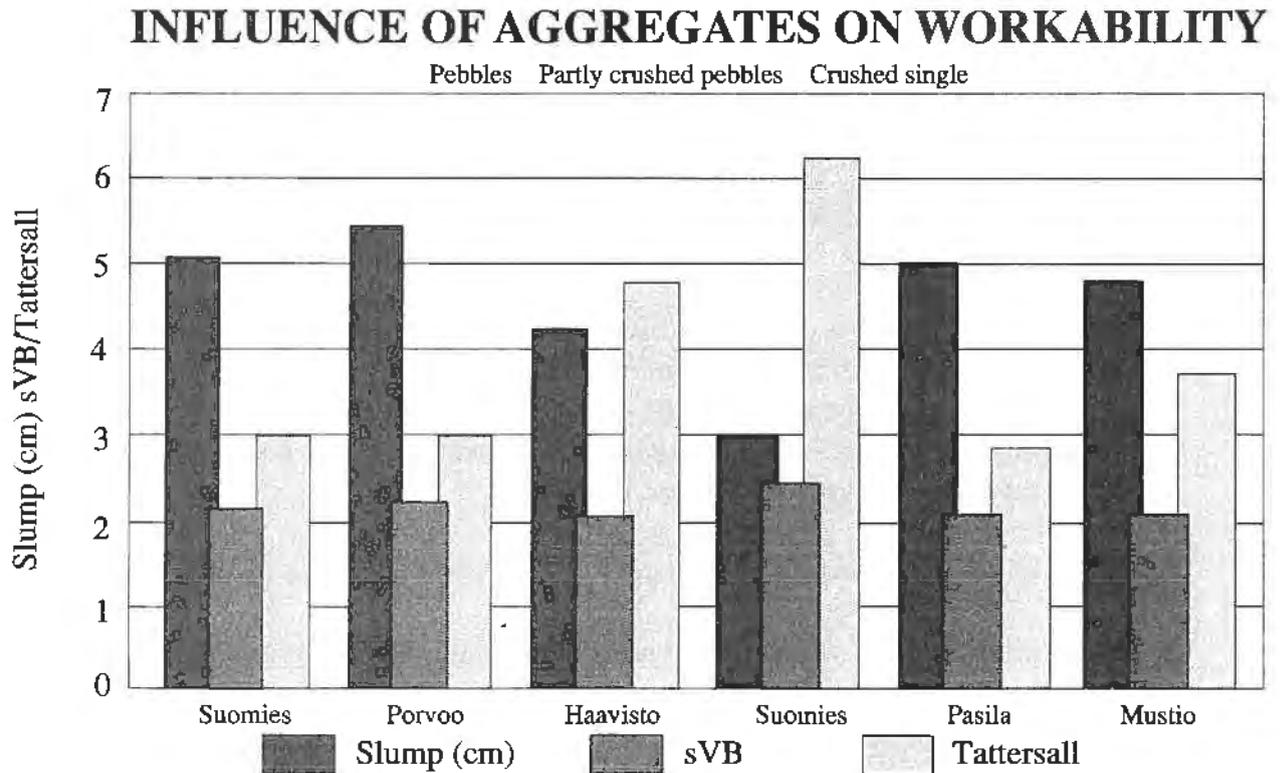
For the coarse aggregate shape of crushed stone strongly affects workability.
