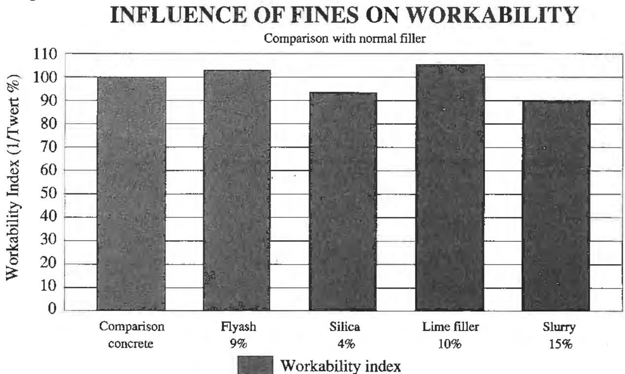
For the fines good-quality flyash and lime filler improve workability whereas silica and slurry make it much worse.
