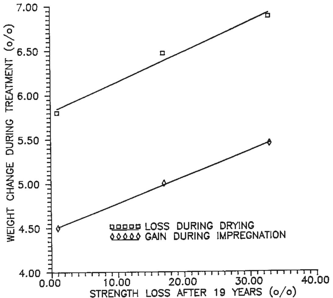
Fig. 5. The linear relation between weight loss during drying and polymer loading with strength loss of PIC curbstones during 19 years outdoor weathering.
