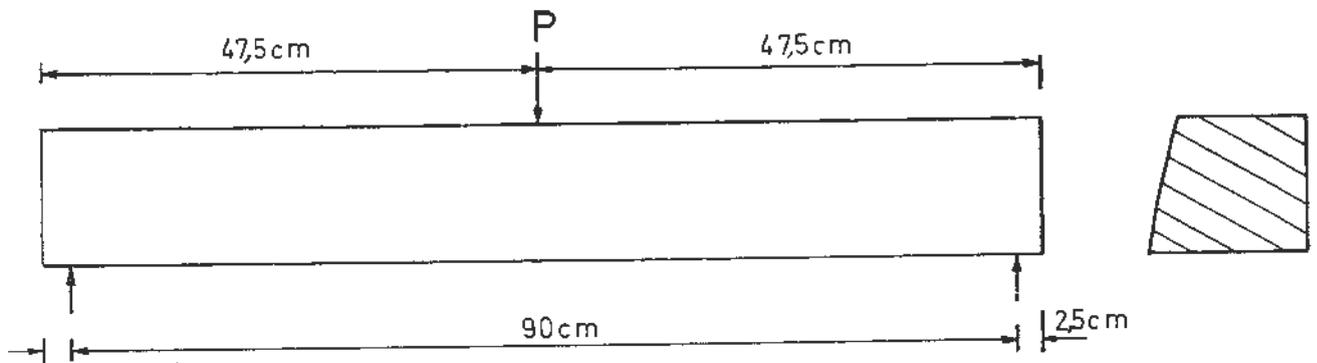
Fig. 2. Dimensions of the curbstones and set up for the testing of load capacity.
