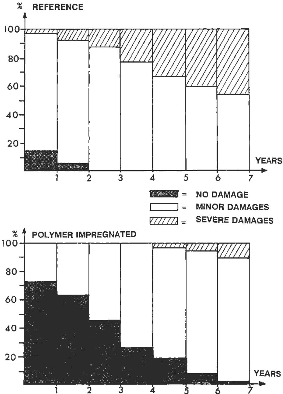
Fig. 1 An evaluation of the performance of untreated concrete curbstones (upper figure) and PIC curbstones (lower figure) during 7 years of field exposure with heavy traffic.
