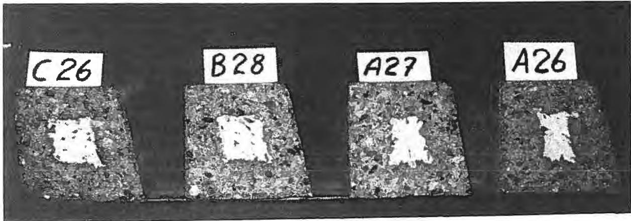
*Fig. 4. A close up of the fracture surface of the curbstones after the load capacity experiment.*
