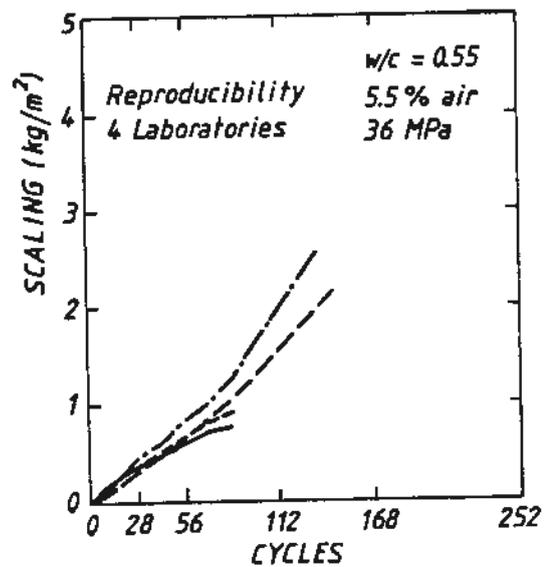
Fig. 2 b      Scaling for concrete B1. Mean values with one specimen excluded at one laboratory
