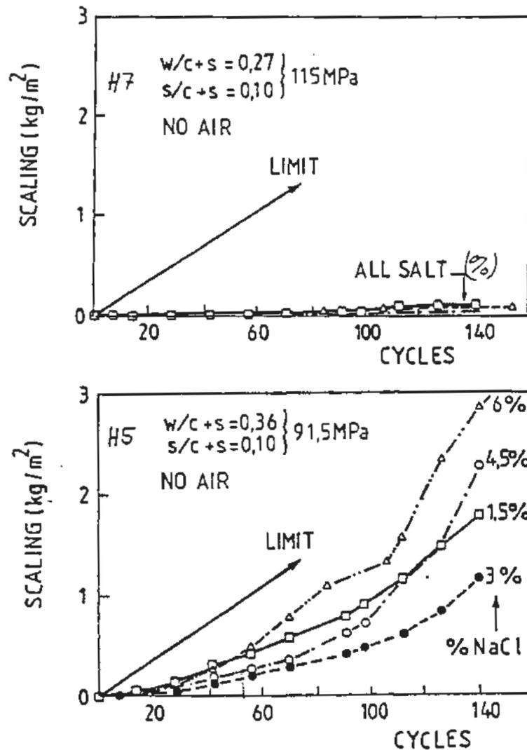
Fig. 6 Scaling of two high strength concretes made with high strength cement P30-4A
