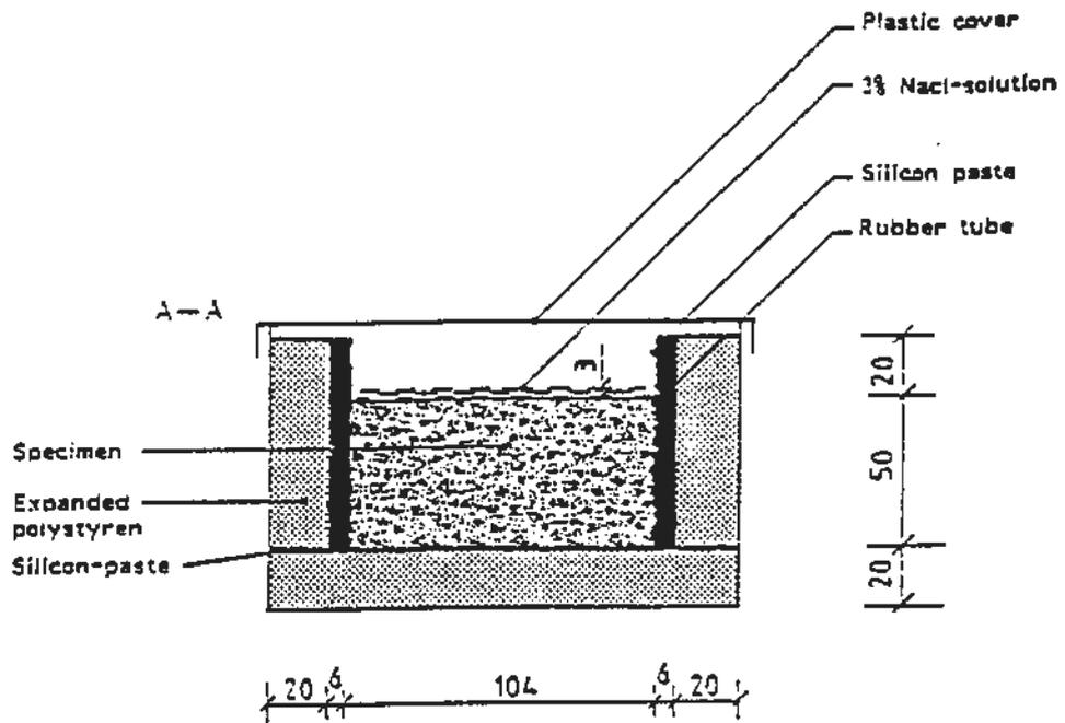
Specimens prepared for SS 13 72 44 freeze/thaw test
