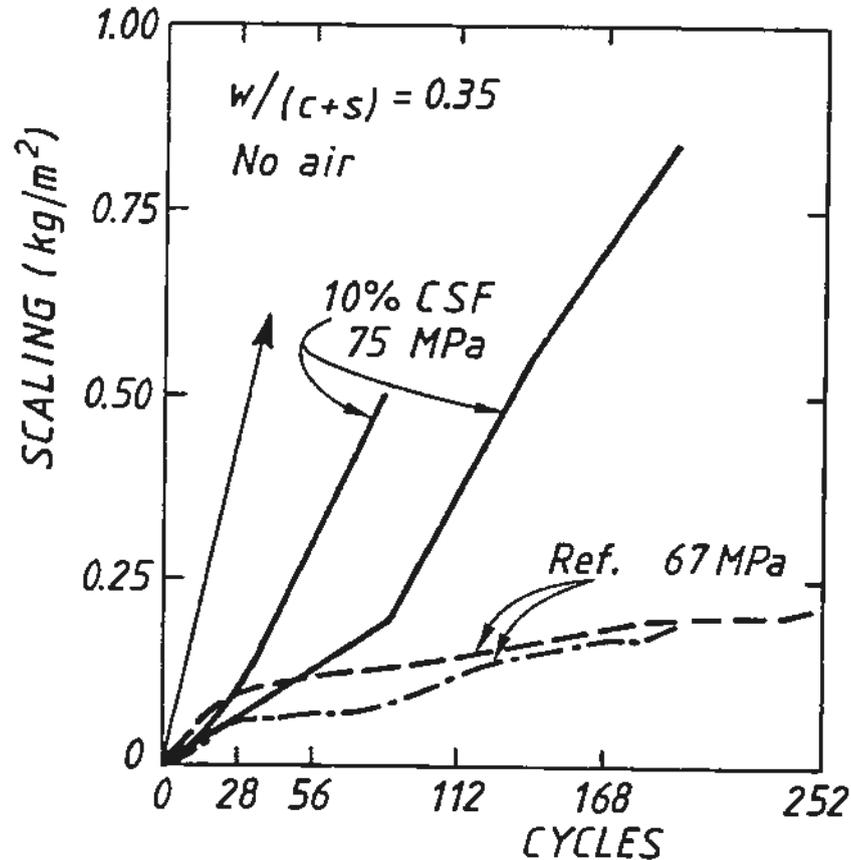
Fig. 9 Scaling of two high strength concretes, each tested at two laboratories
