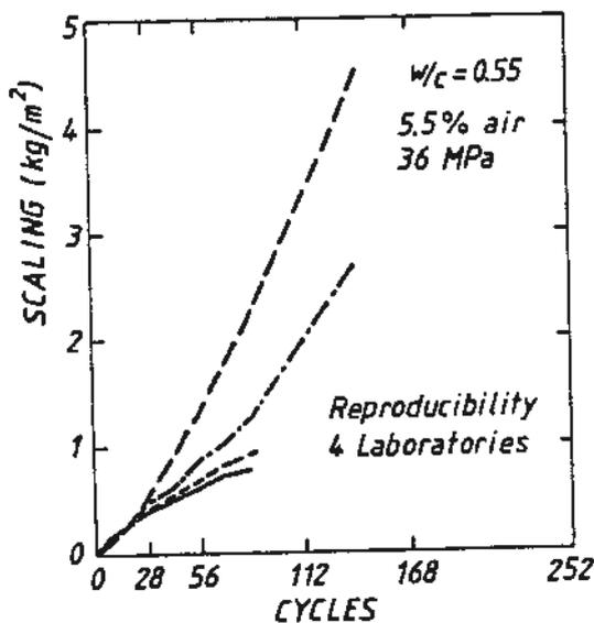
Fig. 2 a      Scaling for concrete B1. Mean values including all test specimens
