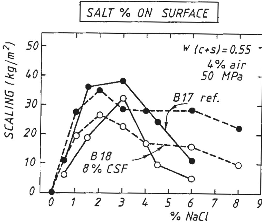
Fig. 5 Scaling with different salt concentrations on the test surface
