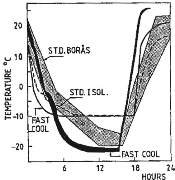
Fig. 4 Achieved temperature cycles in normal freezer ( $-20^{\circ}\text{C}$ ) and more powerful freezer ( $-10^{\circ}\text{C}$ ). Fast cool refers to specimens with less insulation (plastic foil in contact with salt solution)
