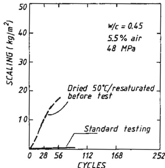
Fig. 3 Scaling with and without drying/resaturation treatment
