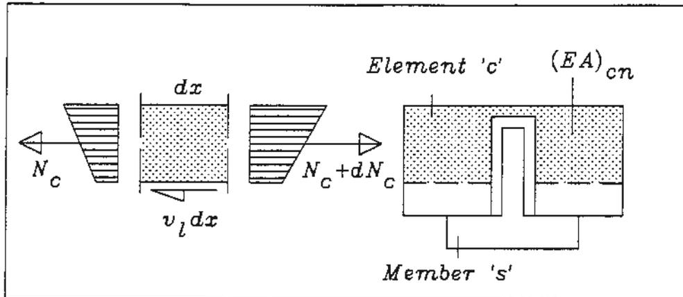
FIG. 4. Horizontal equilibrium must always be maintained between the change in the normal stress resultant and the longitudinal shear force  $v_l dx$  in the element 'c'.
