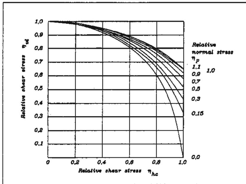
FIG. 6. Shear failure curves for different values of normal stress  $\sigma_{11}$ . Relative normal stress is calculated with respect to the tensile strength of concrete,  $\eta_P = \sigma_{11}/f_{ct}$ .
