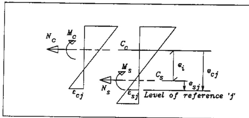
FIG. 3. Strain diagrams for the members 'c' and 's'. The stress resultants are shown to act in their positive directions.
