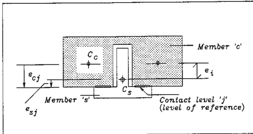
FIG. 2. Composite cross-section of a flexural member where structural parts 'c' and 's' are in contact only on level 'j'.
