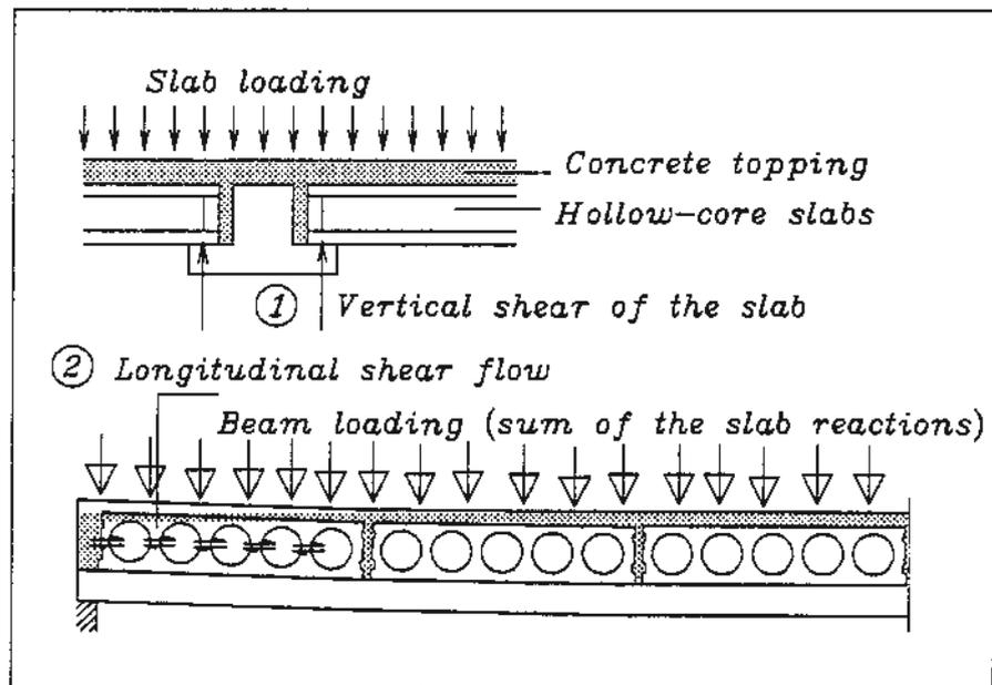
FIG. 1. Shear forces acting on hollow-core sections when slabs are supported by beams: 1) vertical shear due to slab loading, 2) longitudinal shear flow due to composite beam behaviour.
