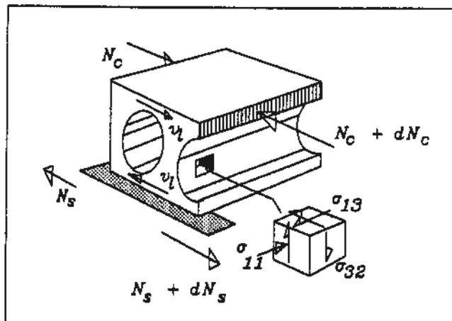
FIG. 5. Stress components for the failure consideration.
