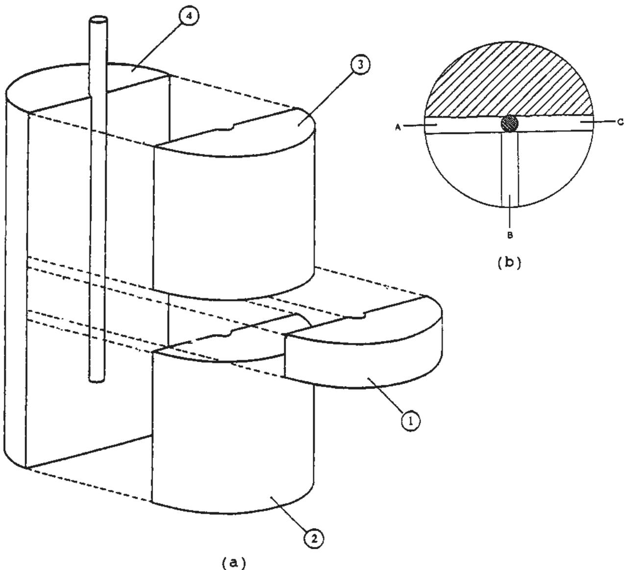
FIG. 1. (a) Location of the different samples for chloride measurements in a cylinder. (b) Position of the radials cut from sample no. 1.
