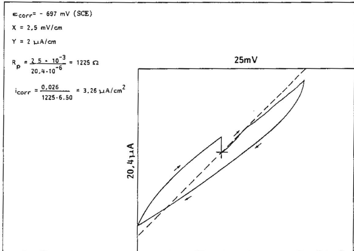
Fig. 3. An example of a polarization curve with the determination of  $i_{\text{corr}}$ .
