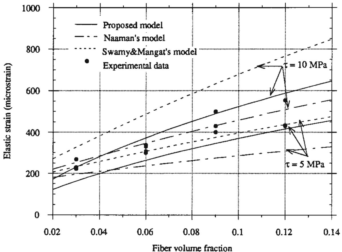
Figure 6. Comparison between experimental data and the proposed model, and the models by Naaman and Swamy&Mangat for fiber reinforced DSP
