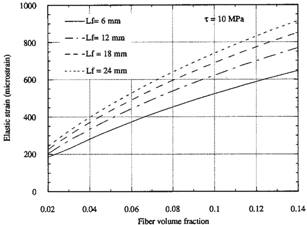
Figure 7 The effect of fiber length on elastic strain for DSP reinforced with small diameter (0.15 mm) steel fibers.
