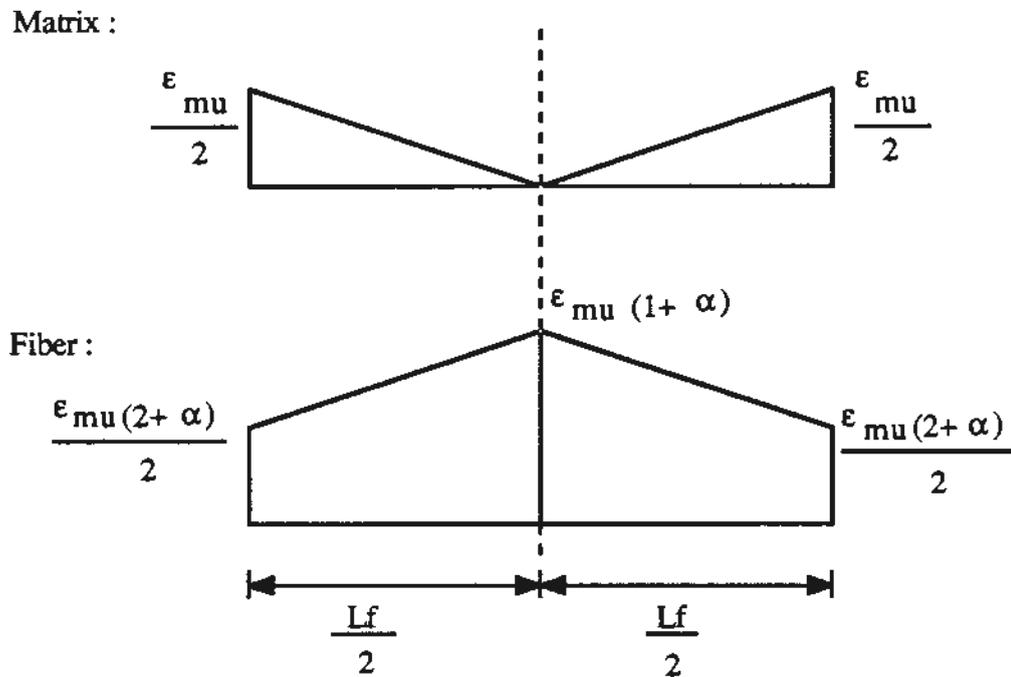
Figure 5 Matrix and fiber strain assumptions used in the model derivation
