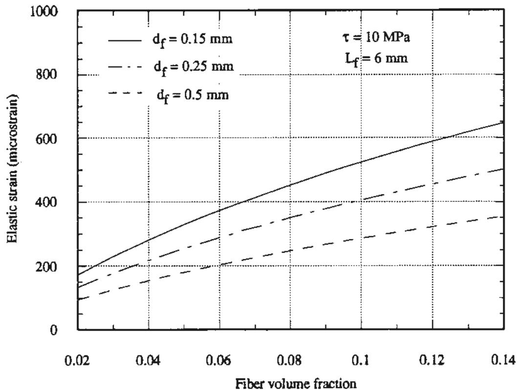
Figure 8. The effect of fiber diameter on elastic strain for fiber reinforced DSP
