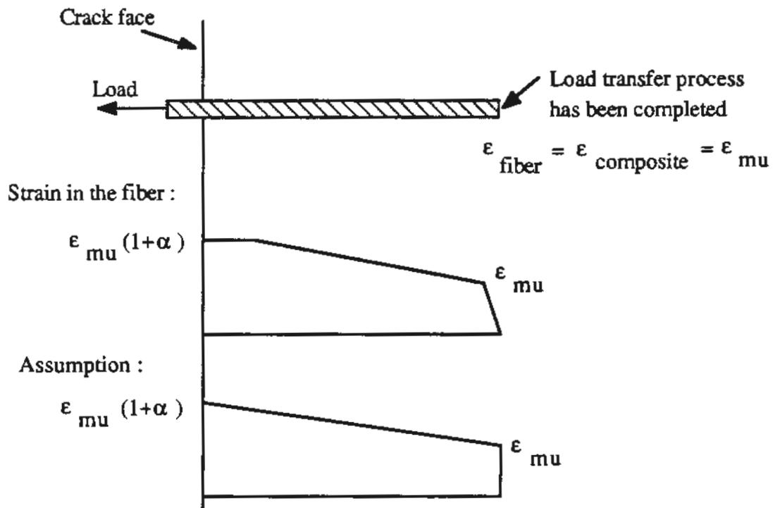
Figure 4 Strain in the fiber just after cracking
