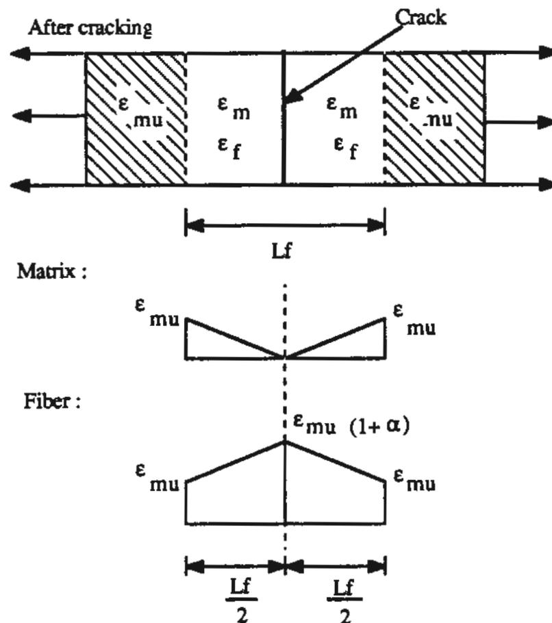
Figure 3 Strain in the composite, matrix, and fiber after the occurrence of the first crack
