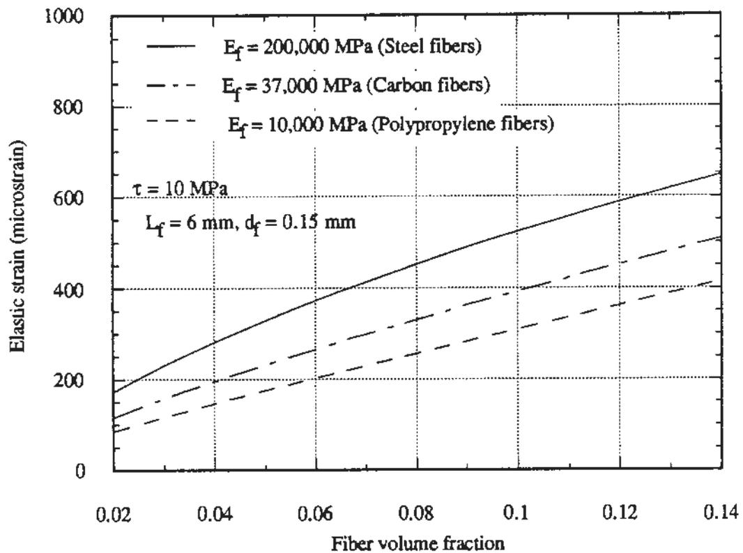
Figure 9. The effect of modulus elasticity of fiber on elastic strain for fiber reinforced DSP
