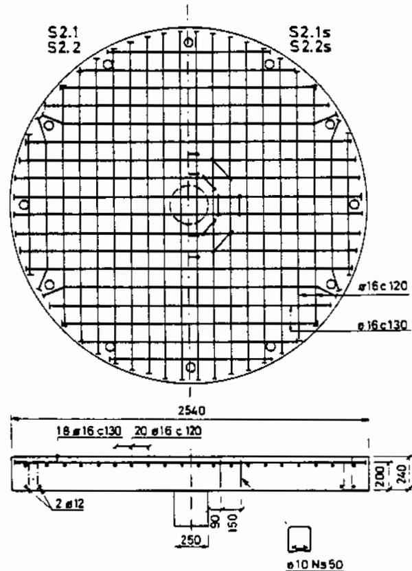
FIG. 2 Reinforcement and nominal dimensions of the test slabs. The left part of the figure shows the slabs without shear reinforcement and the right part shows the slabs with shear reinforcement, tested by Tolf /5/.
