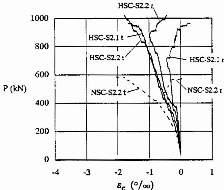
FIG. 4. Concrete strains,  $\epsilon_c$ , at the bottom of the slab 60 mm from the column face in relation to the load,  $P$ .
