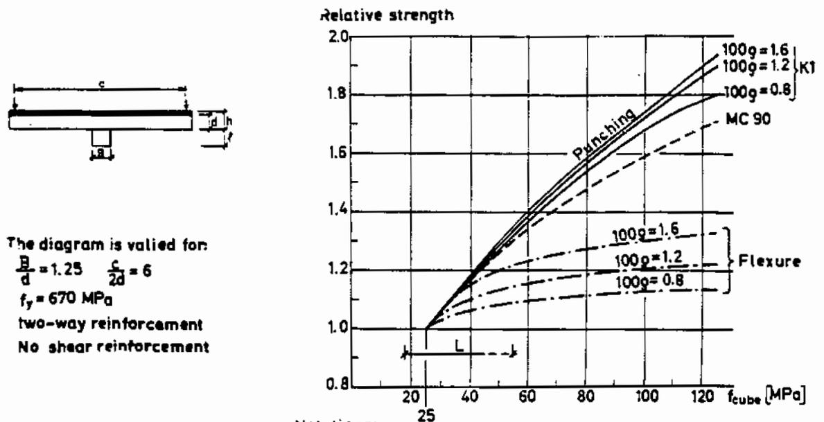
FIG.1 Effect of concrete strength and ratio of reinforcement on load carrying capacity of circular slab on central column.
