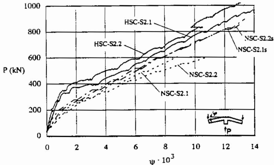
FIG. 6. Angle of rotation,  $\psi$ , of the slab portion outside the shear crack in relation to the load,  $P$ .
