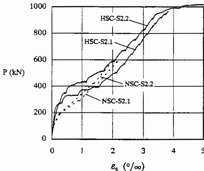
FIG. 5. Observed tensile strains in the flexural reinforcement,  $\epsilon_s$ , above the column in relation to the load, P. The strain was measured at a distance of 65 mm from the centre of the slab.
