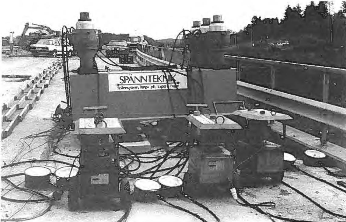
Fig. 6. Loading equipment on top of the prestressed bridge
