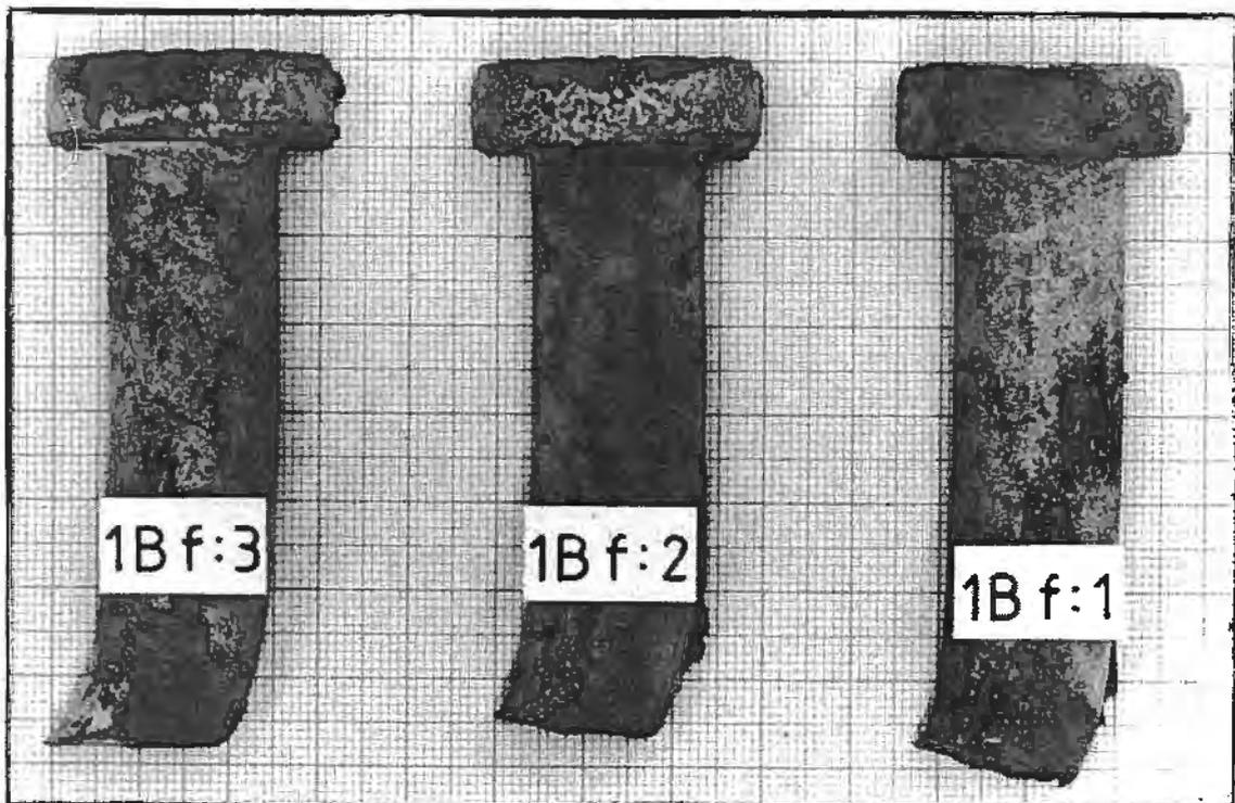
FIG. 8 Fractured studs in 1BF
