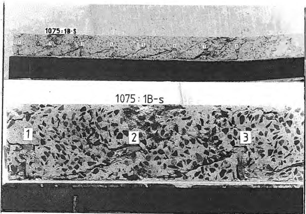
FIG. 6 Crack Distribution in 1BS
