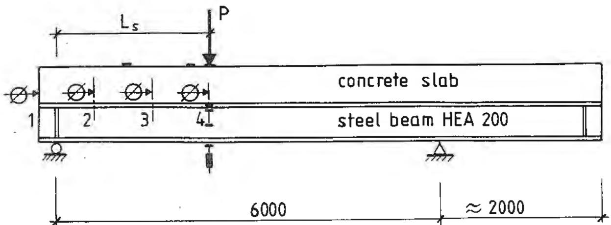
FIG. 2 Test Set-up and Instrumentation
