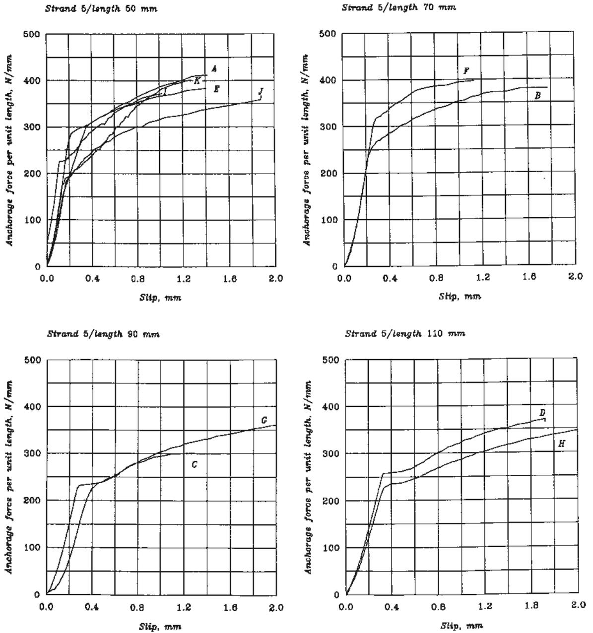
FIG. 9. Load-slip curves for tests A - K: strand 5
