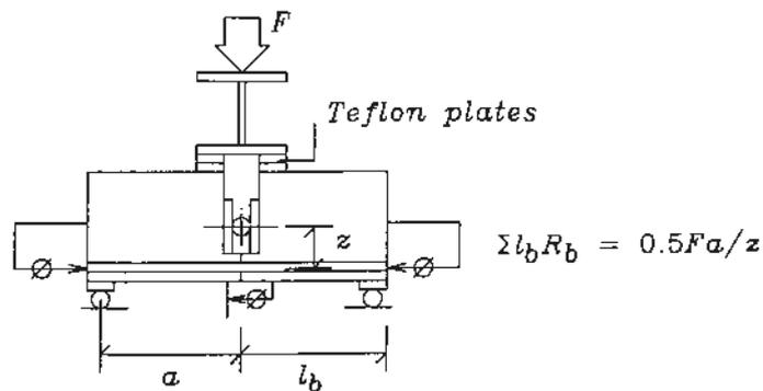
FIG. 4. The flexural pull-out test applied to a hollow-core slab
