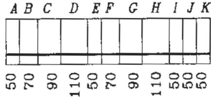
FIG. 7. Series of slices of a V6 hollow-core slab used to study the effect of embedment length on bond strength. The cross-section of the slab contains 5 strands having a nominal diameter of 9.3 mm.
