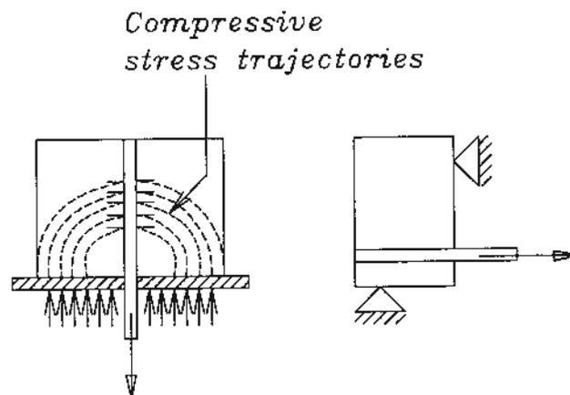
FIG. 2. Pull-out set ups for anchorage tests
