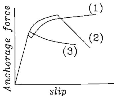
FIG. 5. Types of load-slip curves found in push-out tests
