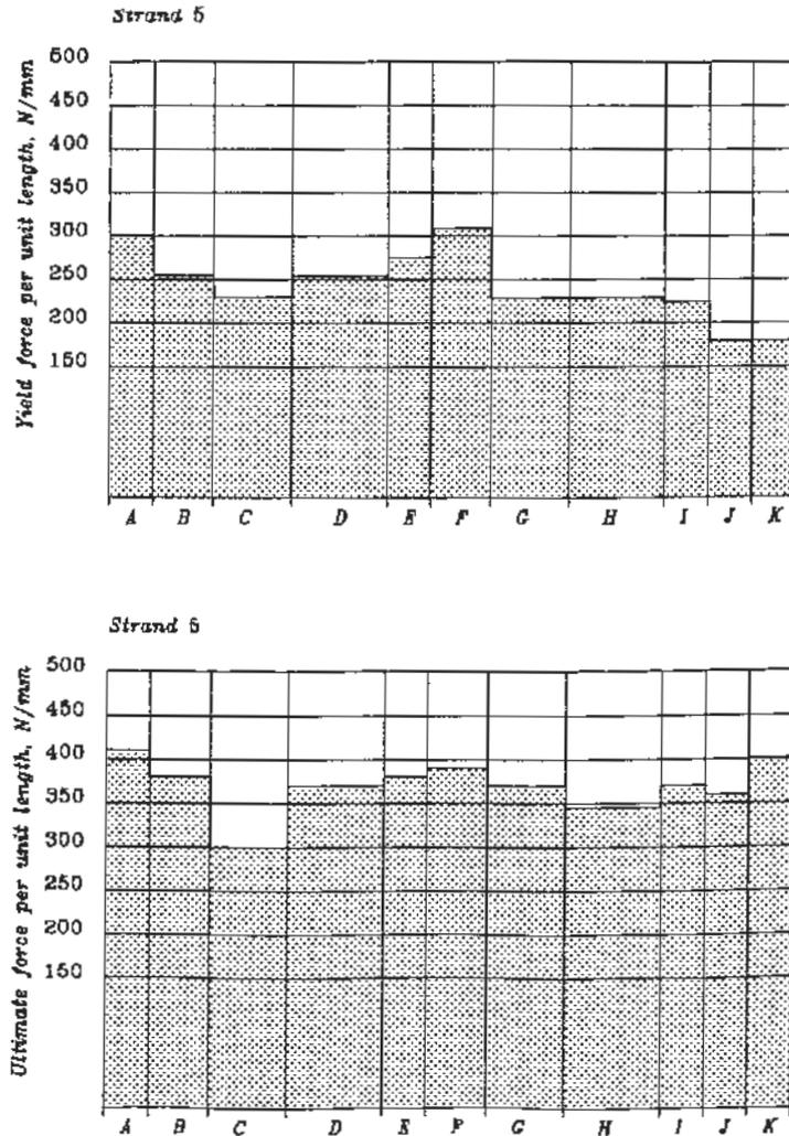
FIG. 8. Profiles of test results concerning the effect of embedment length: strand 5. Since the peak values are situated randomly in all strands, it can be assumed that the lengths used give similar results. It is not possible to use greater lengths because of yielding in the indenter and strand head.
