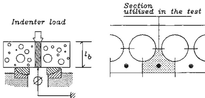
FIG. 3. Principle of the push-out test on hollow-core slabs
