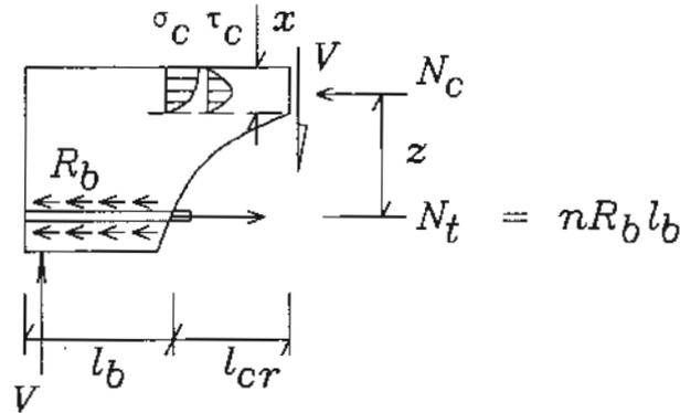
FIG. 1. The equilibrium mechanism involved in the shear-bond failure
