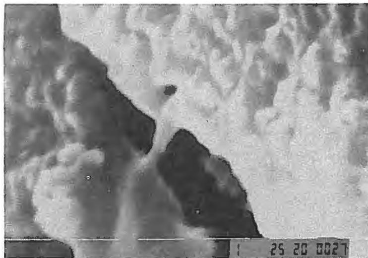
Fig 6. Fracture surface of a PCC with 10 vol% SBR showing the crack bridging ability of the polymer (12000X SEM)
