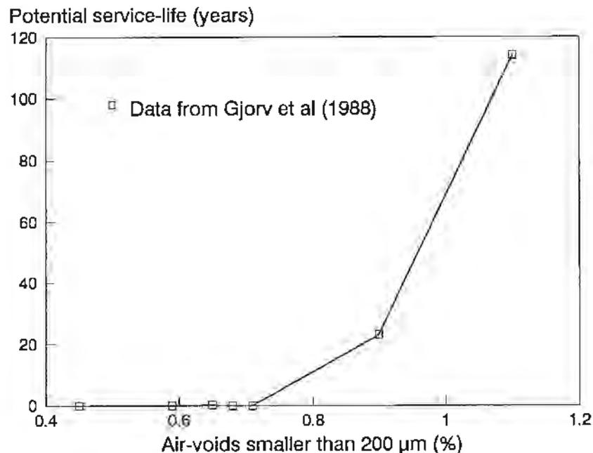
Fig 1 Potential service-life vs air-voids smaller than 200  $\mu\text{m}$
