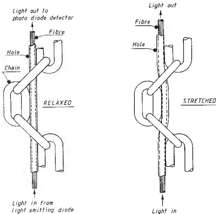
Fig 3. The chain in relaxed and stretched conditions /5/
