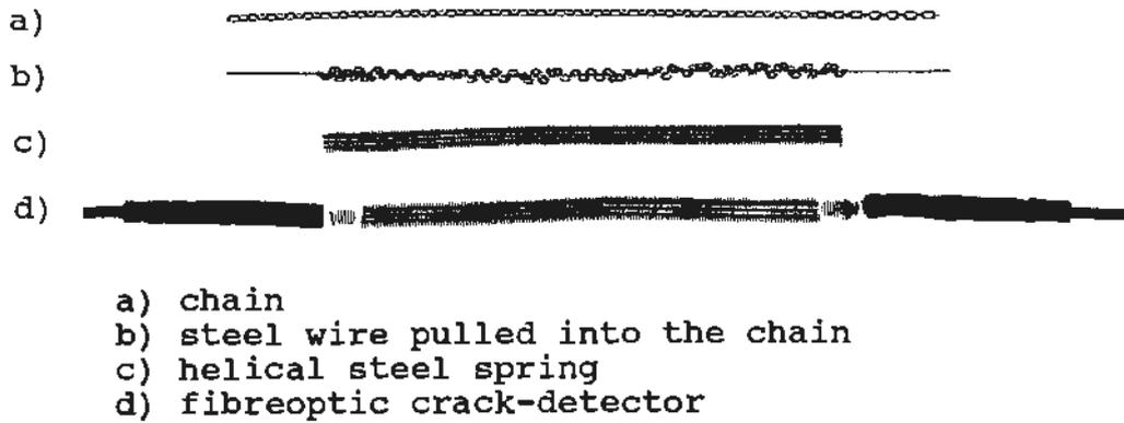
Fig 5. The different parts of the detector
