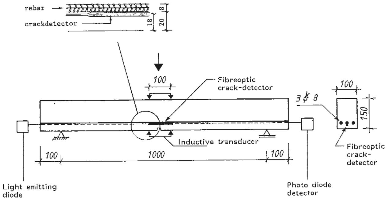
Fig 6. A beam undergoing three-point-bending, measurement in millimetres
