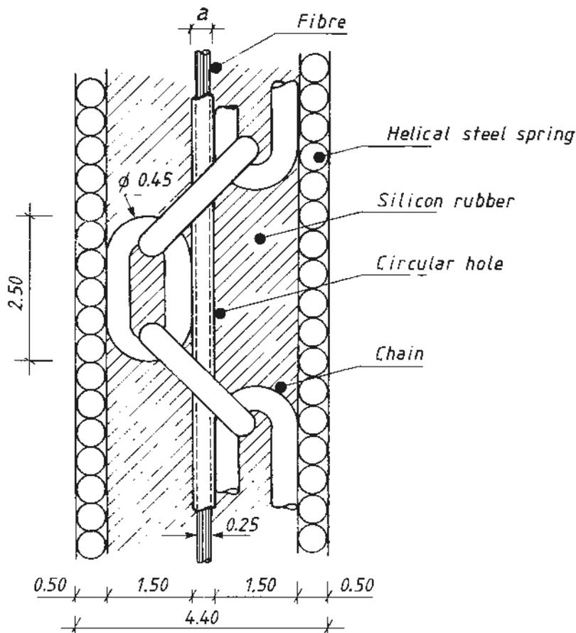
Fig 4. Construction of the fibreoptic crack-detector, measured in millimetres
