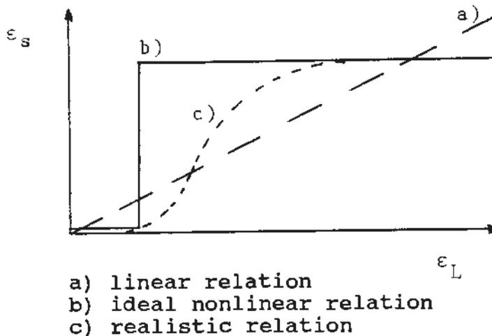
Fig 2. Elongation of the detector ( $\epsilon_s$ ) as a function of the elongation in the concrete ( $\epsilon_L$ ) /5/
