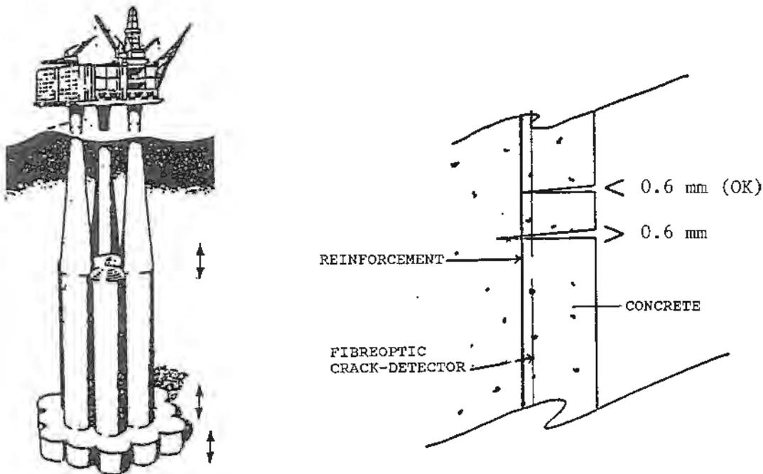
Fig 1. Location of the fibreoptic crack-detector and a sketch showing the principle /4/
