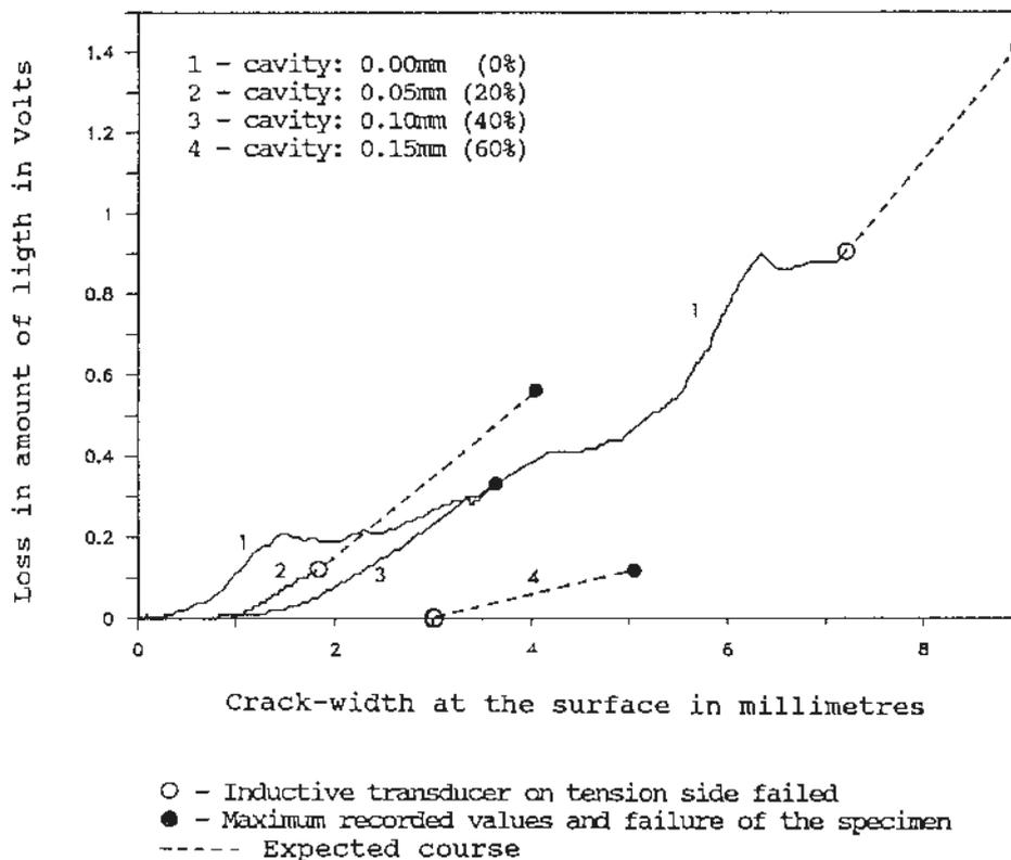
Fig 7. The loss in the amount of light through the fiberoptic crack-detector shown together with the corresponding crack-widths
