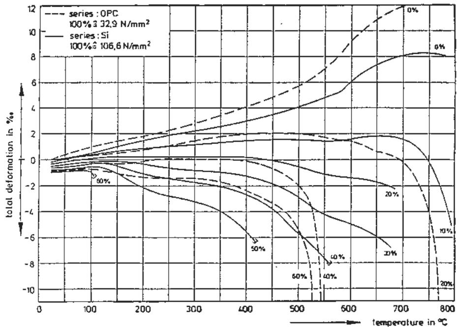
Fig. 6. Total deformation of loaded Si-concrete and normal strength OPC-concrete during heating.
