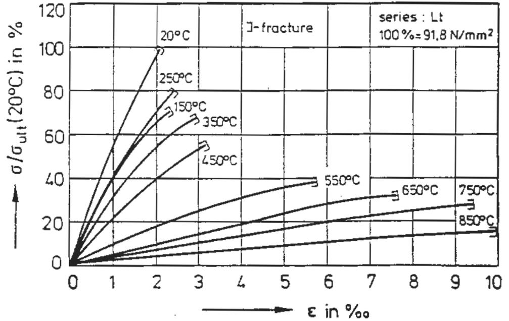
Fig. 3. Stress-strain relationships of Lt-concrete tested at high temperatures.
