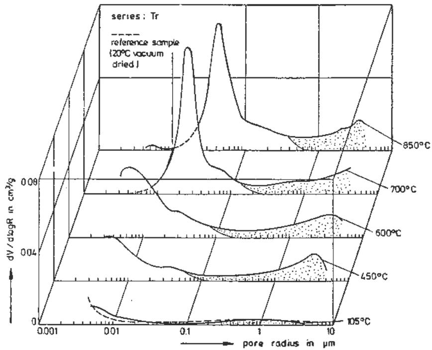
Fig. 2. Differential pore size distribution of heated Tr-concrete.
