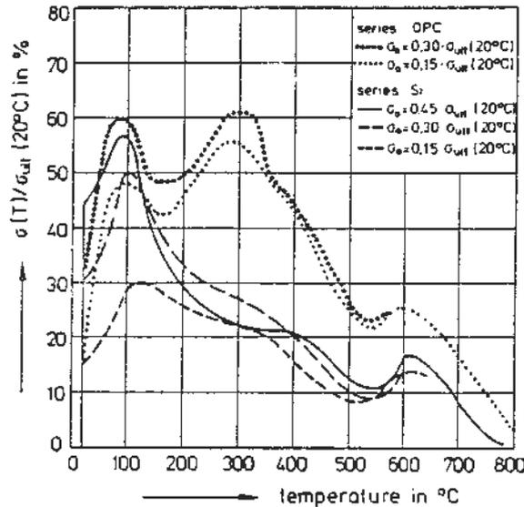
Fig. 8. Restraint forces of Si- and OPC-concretes.
