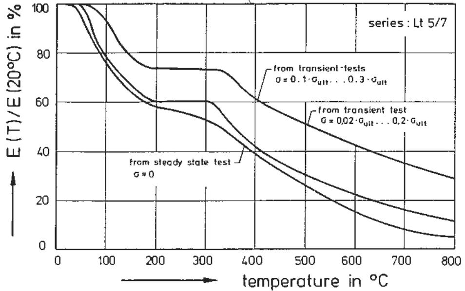
Fig. 7. Modulus of elasticity of Lt-concrete.
