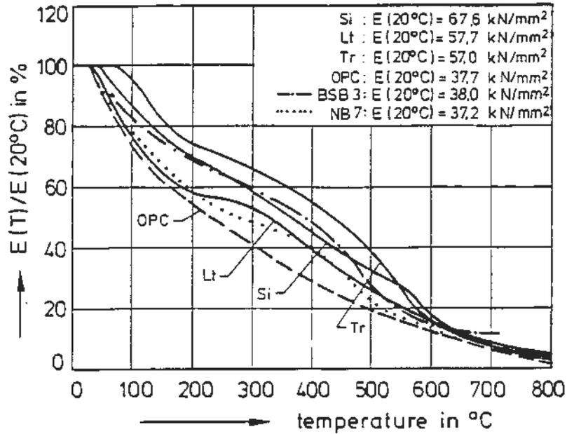
Fig.5. Modulus of elasticity of various high strength and normal strength concretes.
