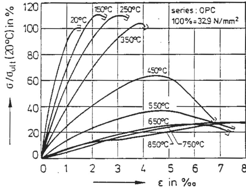
Fig. 4. Stress-strain relationships of OPC-concrete tested at high temperatures.
