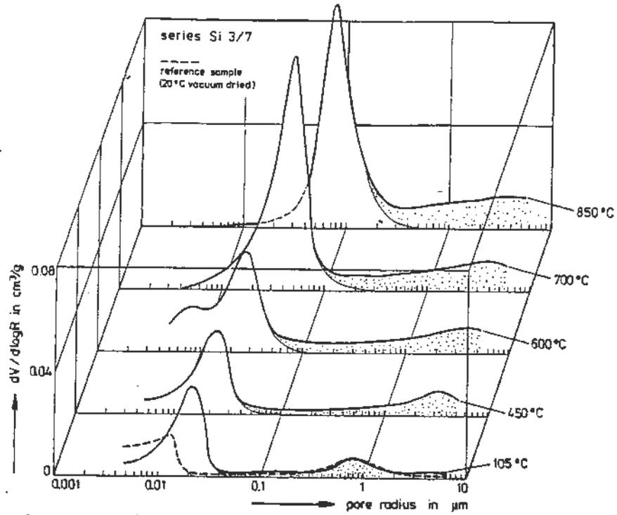
Fig. 1. Differential pore size distribution of heated Si-concrete.
