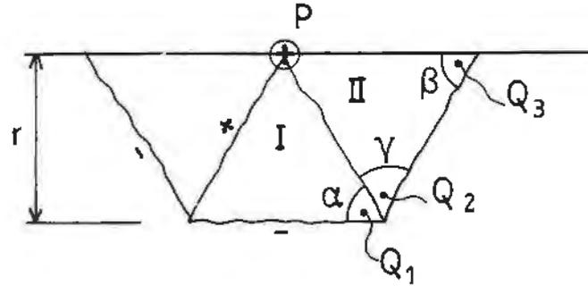
FIG. 2. The yield-line pattern for the case of a point-load on the free edge of a cantilever slab.
