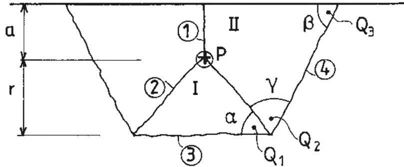
FIG. 3. The yield-line pattern for the case of a point-load at a distance  $a$  from the free edge of a cantilever slab.
