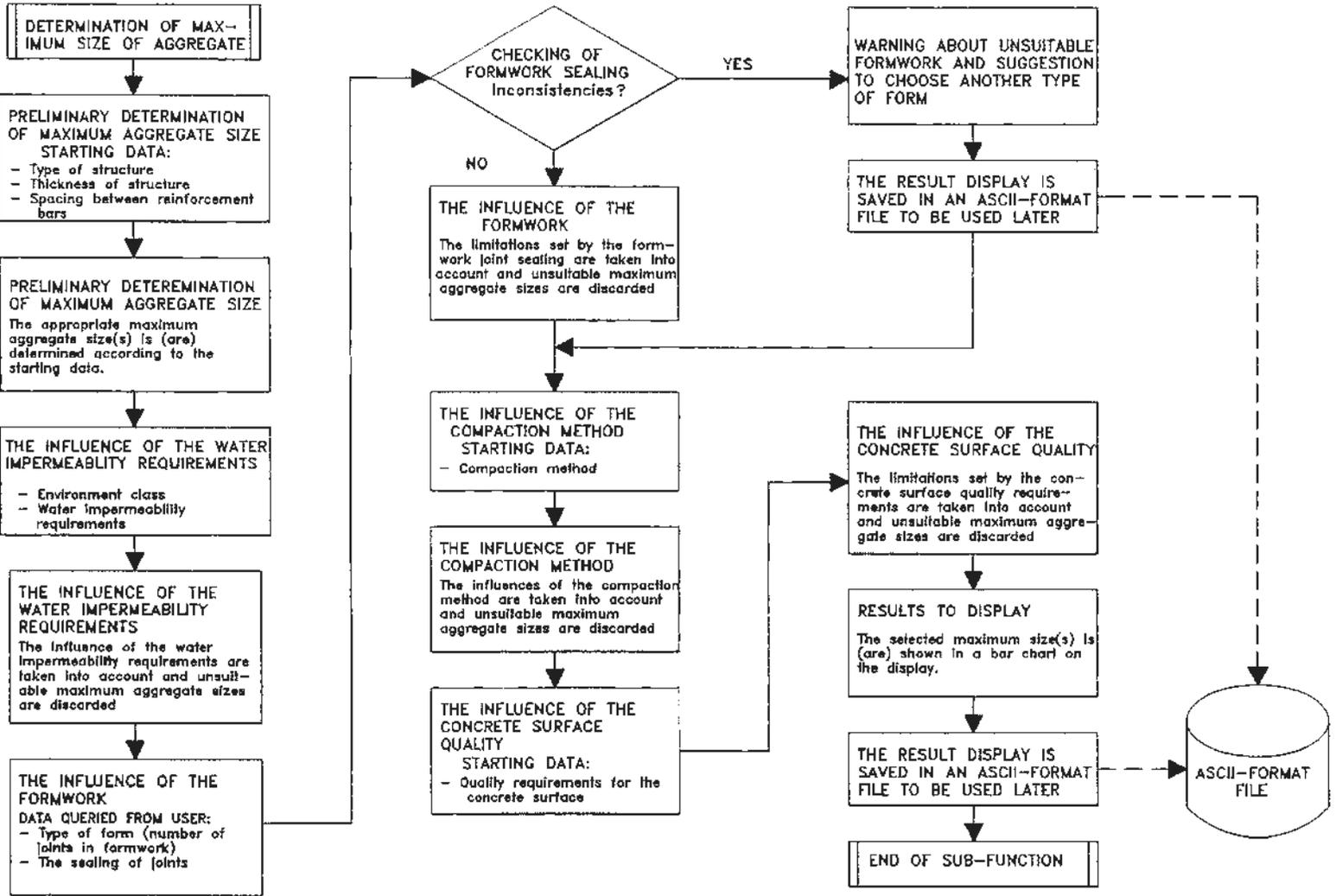
Fig. 8. The course of inference in the context for determining the maximum size of aggregate.
