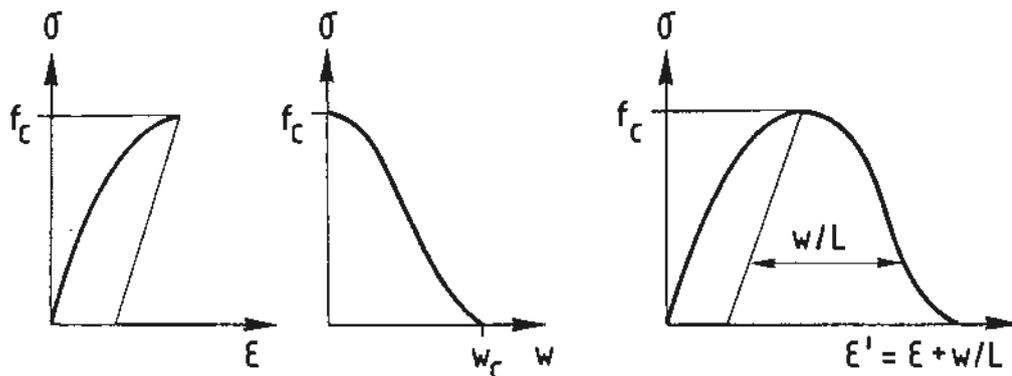
Fig. 1. The description of the stress-deformation relation by means of two diagrams.
