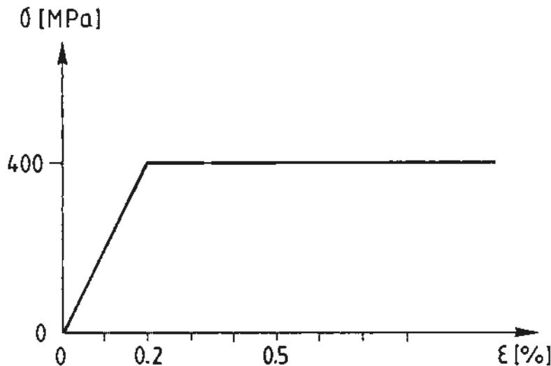
Fig. 4. Elastic-perfectly plastic stress-strain curve for the reinforcing steel.
