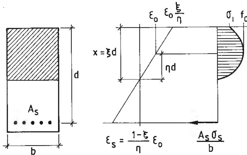
Fig. 3. Assumed strains and stresses in a rectangular beam section.
