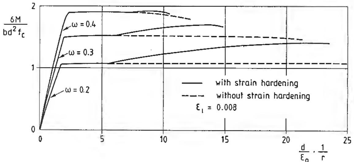
Fig. 7. Examples of theoretical moment-curvature relations with an assumed curve according to Fig. 6.
