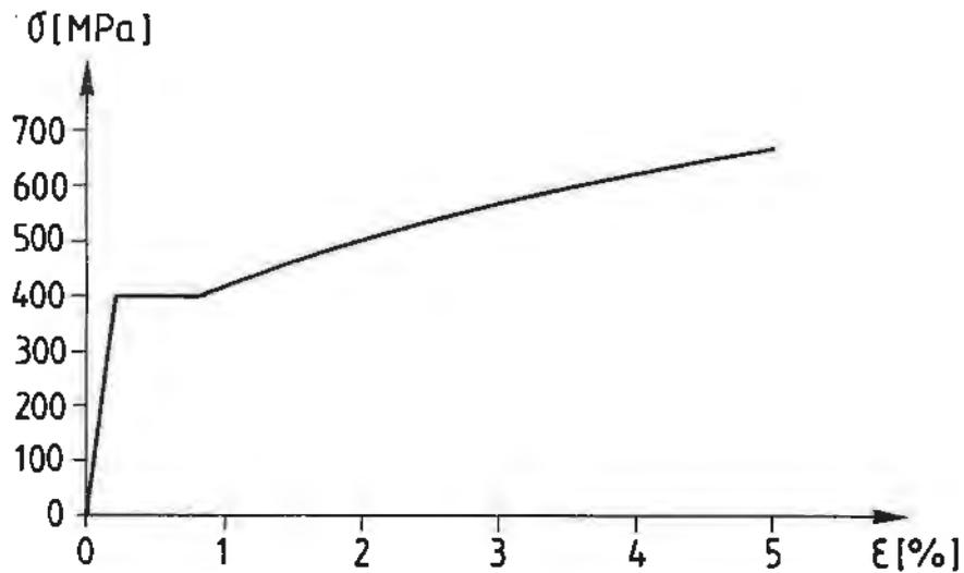
Fig. 6. Strain-hardening stress-strain curve for the reinforcing steel.
