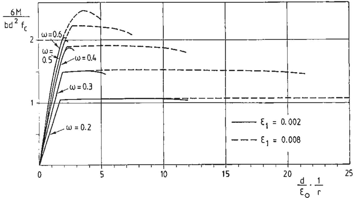
Fig. 5. Examples of theoretical moment-curvature relations with assumptions according to Figs. 2-4.
