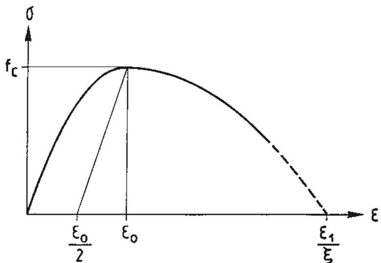
Fig. 2. Assumed parabolic shape of the formal stress-strain relation on length  $L$ , used in the numerical analysis.
