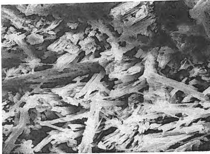
Figure 4. a) Air pores filled with ettringite
