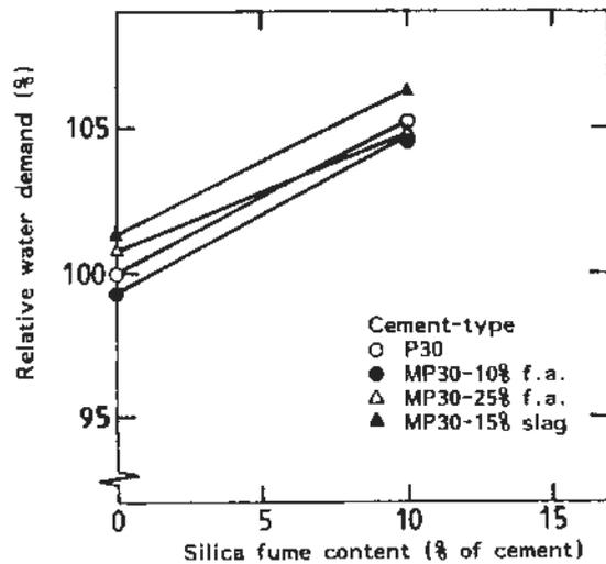
Fig 1. Mean water demand for concrete strength grades C25 and C45 with different cement types as a function of silica fume content /2/
