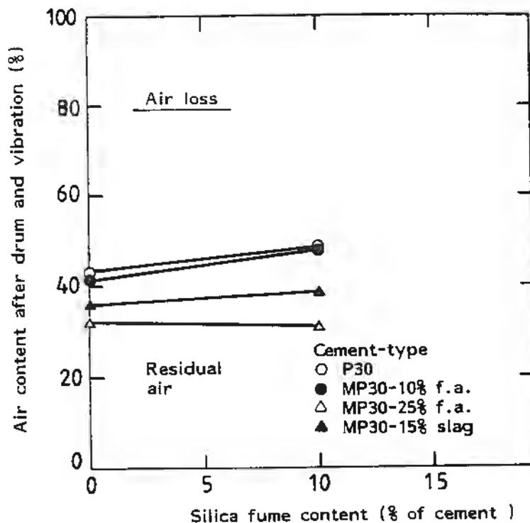
Fig 3. Air content in concrete after 60 min drum testing and then in the vibration test for 3 min in % of air content before testing depending on cement type and silica fume content /2/
