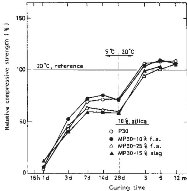
Fig 8. Compressive strength development of concrete cured in water at 5°C the first 28 days and then in water at 20°C in % of strengths for comparable mixes cured at 20°C continuously. 10 % silica fume by weight of cement was used /3/
