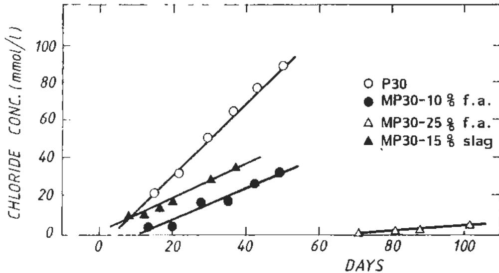
Fig 12. Chloride diffusion through disks of cement paste of different cement types with w/c ratio equal to 0.5. No silica fume was added /8/
