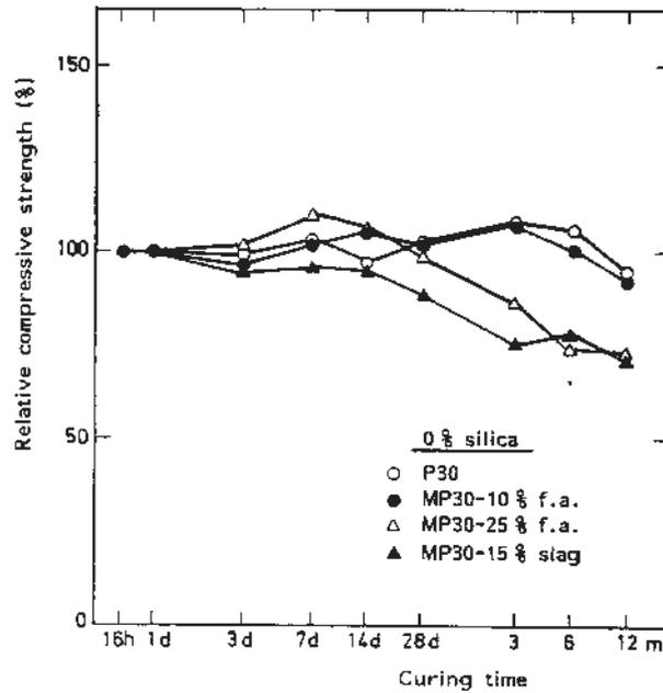
Fig 5. Relative compressive strength of concrete cured in air at 20°C and 50 % RH in % of strength of the same mixes cured in water at 20°C. No silica fume was used /3/
