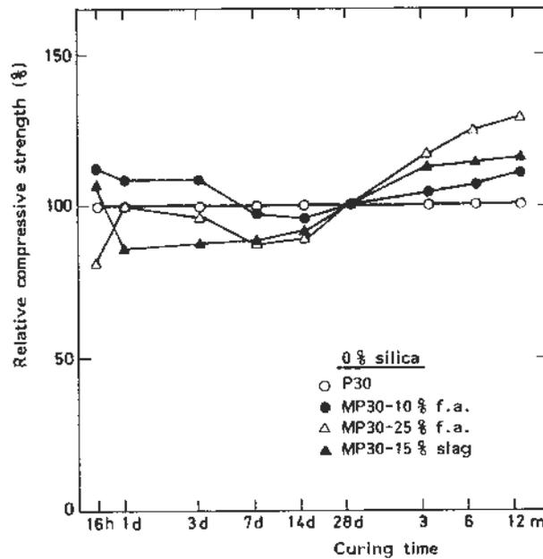
Fig 4. Relative compressive strength of concrete cured in water at 20°C depending on cement type and curing time. Concrete of P30 cement is 100% at any time. No silica fume was used /3/
