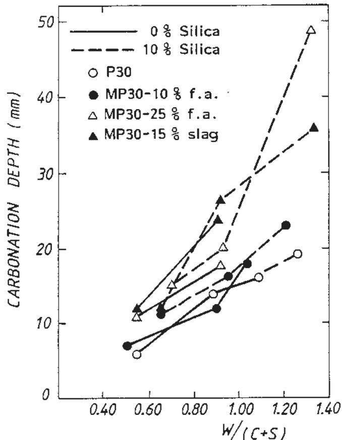
Fig 11. Absolute carbonation depths for samples stored in air at 20°C and 50 % RH for three years as a function of cement type, silica fume and w/(c+s) ratio /11/
