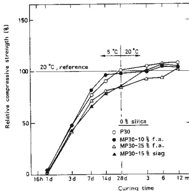
Fig 7. Compressive strength development of concrete cured in water at 5°C the first 28 days and then in water at 20°C in % of strengths for comparable mixes cured at 20°C continuously. No silica fume was used /3/
