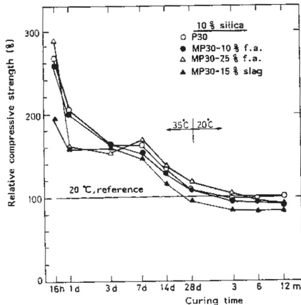
Fig 10. Compressive strength development of concrete cured in water at 35°C the first 28 days and then in water at 20°C in % of strengths for comparable mixes cured at 20°C continuously. 10 % silica fume by weight of cement was used /3/
