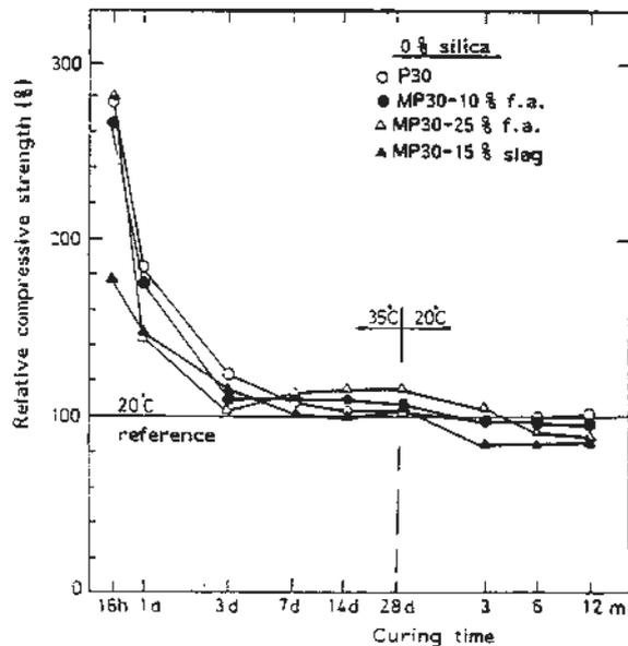
Fig 9. Compressive strength development of concrete cured in water at 35°C the first 28 days and then in water at 20°C in % of strengths for comparable mixes cured at 20°C continuously. No silica fume was used /3/
