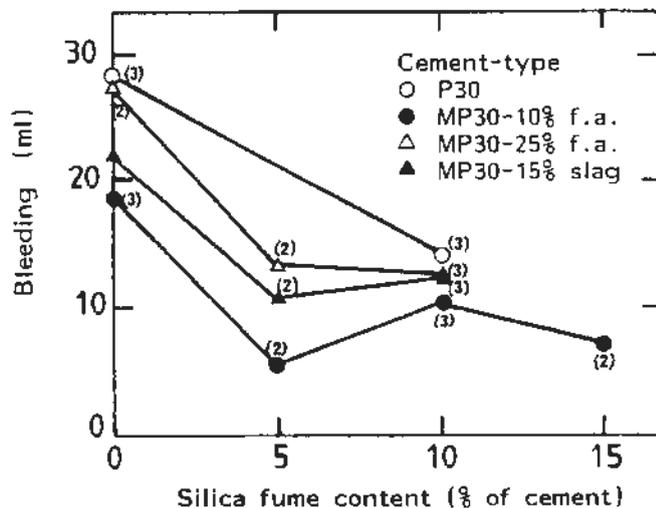
Fig 2. Mean bleeding in concretes with different cement types as a function of silica fume content /2/
