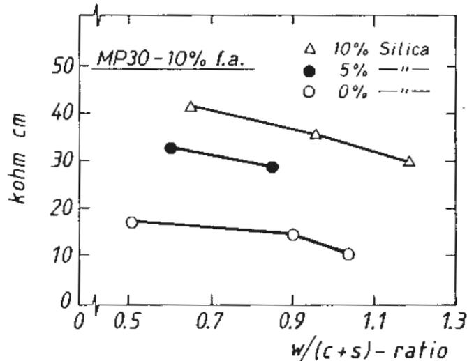
Fig 14. Specific electrical resistivity in concrete as a function of silica fume dosage and w/c+s ratio in saturated samples /8/
