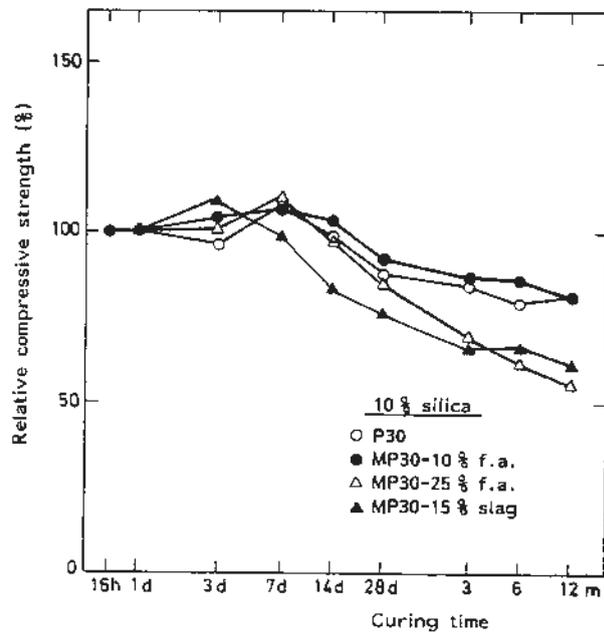
Fig 6. Relative compressive strength of concrete cured in air at 20°C and 50 % RH in % of strength of the same mixes cured in water at 20°C. 10 % silica fume by weight of cement was used /3/
