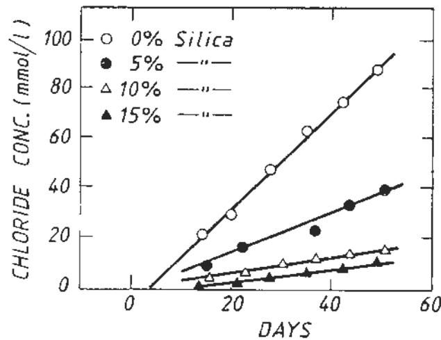
Fig 13. Chloride diffusion through disks of P30 cement with different silica fume dosages with w/c+s ratio equal to 0,5 /8/
