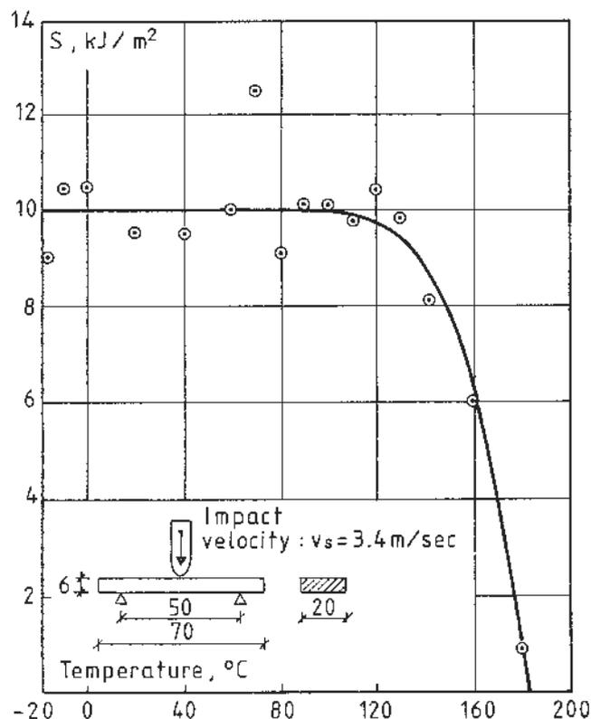
Fig. 3 Izod impact strength, S , for 6 mm polypropylene fibre reinforced plate material tested at different temperatures. (Dimensions in mm).
