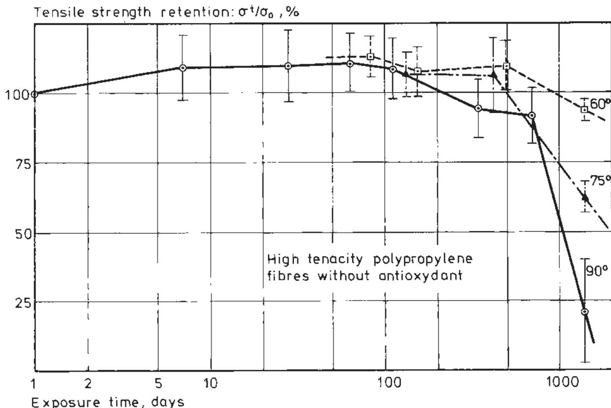
Fig. 7 Development of the tensile strength of plastic fibre rovings in accelerated tests at elevated temperatures (60°, 75° and 90° C). Fibre material: Polypropylene without antioxidant additive.
