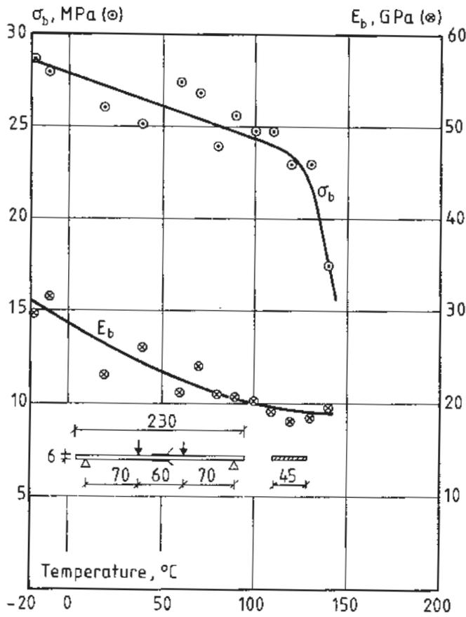
Fig. 2 Modulus of rupture,  $\sigma_b (= M/W)$ , and elastic modulus in bending,  $E_b$ , for 6 mm FRC-plate material tested at different temperatures. Polypropylene fibre reinforcement:  $V_F \sim 10$  vol-%. (Dimensions in mm).
