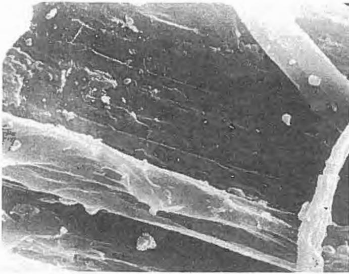
Fig. 8 SEM-photo of polypropylene fibres with antioxidant additive after 1400 days immersion at 90° C in concentrated Portland cement substrate saturated with oxygen, (1.430 x) . (Residual tensile strength:  $\sigma^t/\sigma_0 = 0.70$ ).
