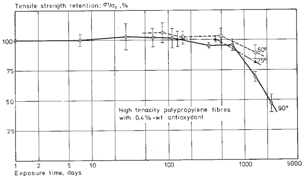
Fig. 6 Development of the tensile strength of plastic fibre rovings in accelerated tests at elevated temperatures ( $60^\circ$ ,  $75^\circ$  and  $90^\circ \text{C}$ ). Fibre material: Polypropylene containing 0.4% antioxidant additive.
