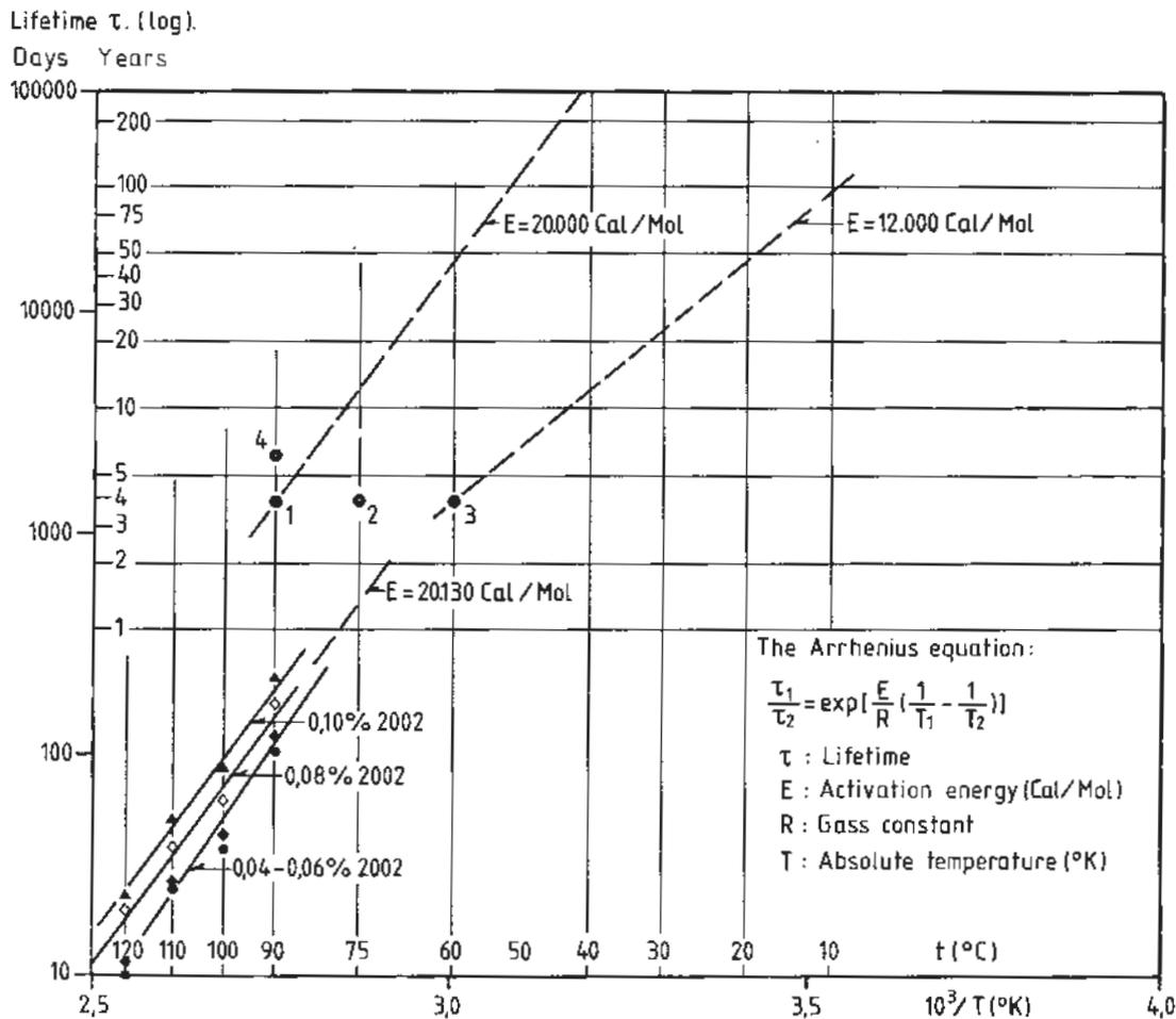
Fig. 4 Arrhenius diagram showing results from accelerated tests at elevated temperatures for estimating the durability of polypropylene fibres at ordinary ambient temperatures.
