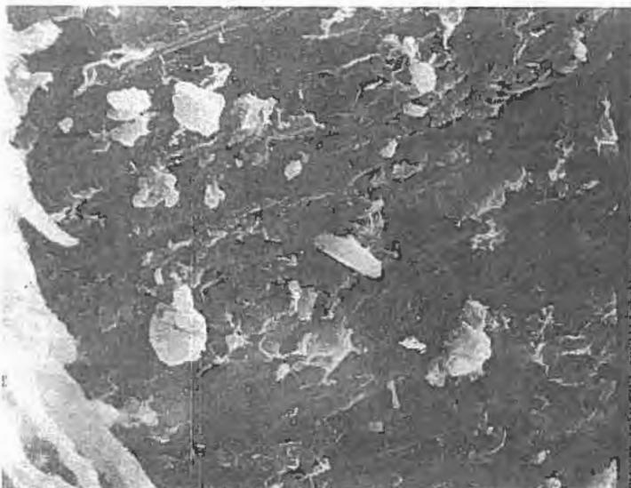
Fig. 9 SEM-photo of polypropylene fibres without antioxidant additive after 1400 days immersion at 90° C in concentrated Portland cement substrate saturated with oxygen, (1.430 x) . (Residual tensile strength:  $\sigma^t/\sigma_0 = 0.09$ ).
