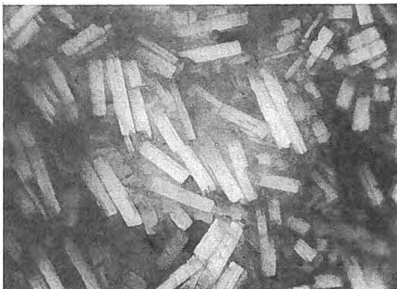
Fig. 5 Micro-photo of cross section in a fibre bundle of high tenacity polypropylene split fibres (100 x).
