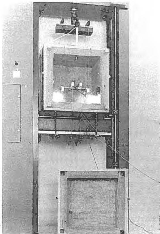
Fig. 1 10 tons Instron testing machine with cooling and heating equipment for making bending tests at constant temperatures in the range:  $\pm 20^{\circ}$  C to  $+140^{\circ}$  C.
