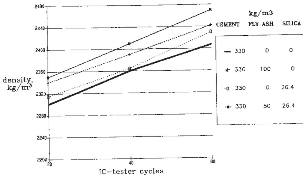
Figure 7. The effect of silica fume and fly ash on the workability of concrete.
