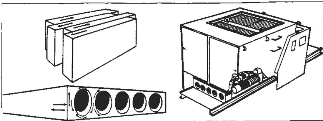
Figure 2. Shear compaction method.
