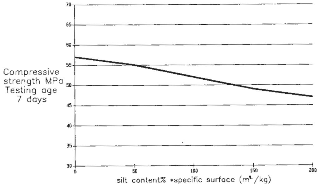
Figure 5. The effect of the silt included in aggregate on the compressive strength of concrete.
