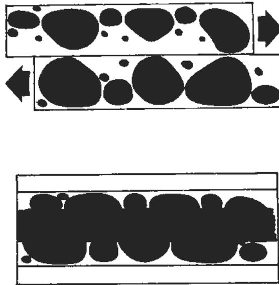
Figure 1. The aggregates are brought into the appropriate positions during shear compaction.
