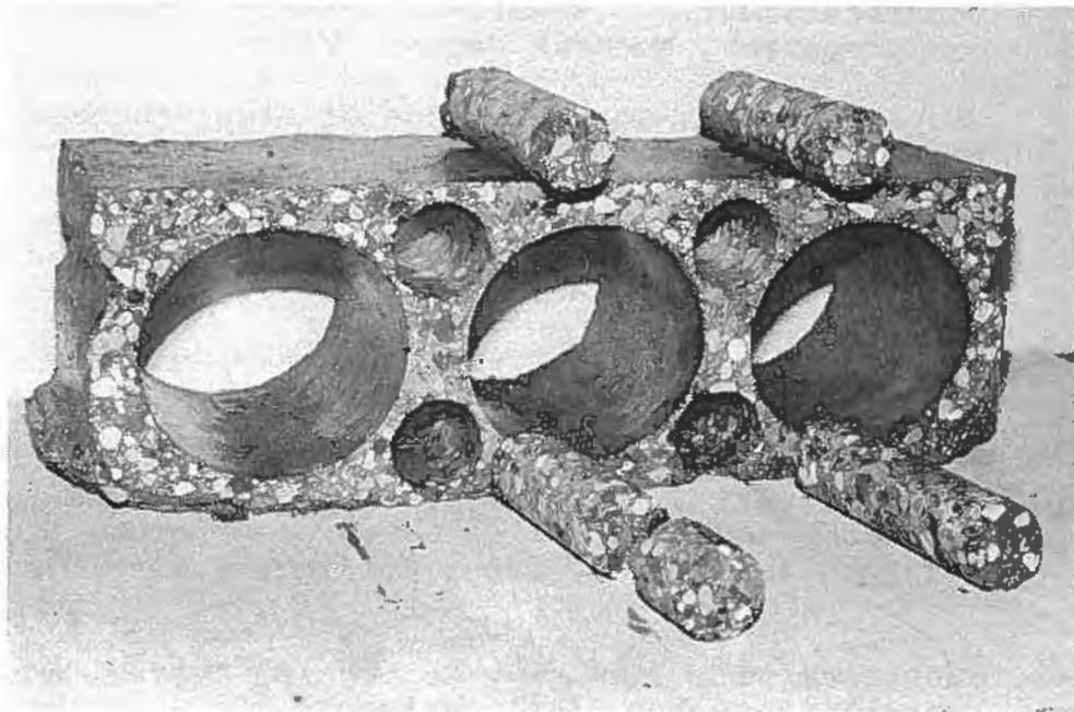
Photo 2. The cross-section of a hollow-core slab with drilled cores, manufactured in laboratory.
