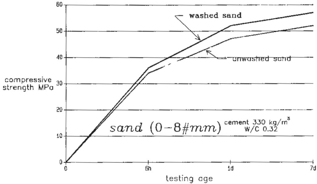
Figure 4. The effect of washed aggregate on the development of the strength of no-slump concrete.
