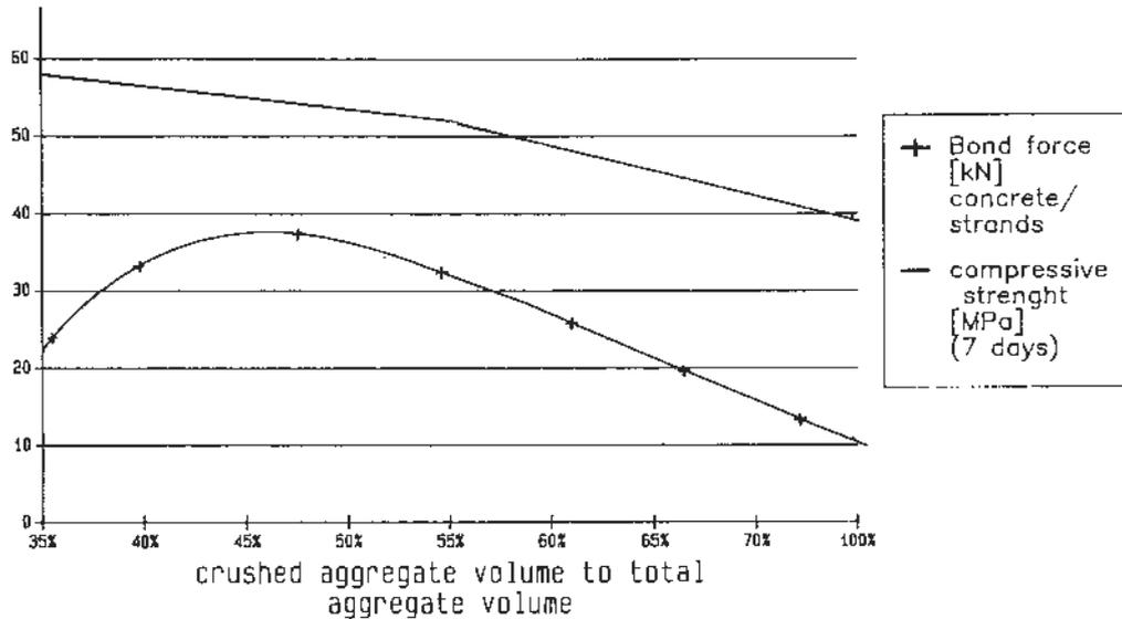
Figure 6. The effect of crushed aggregate on the compressive strength and the adhesion to prestressing strands.
