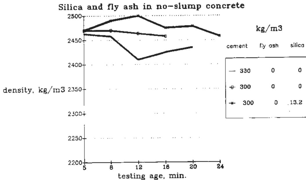
Figure 9. Stiffening of no-slump concrete with fly ash and silica fume.
