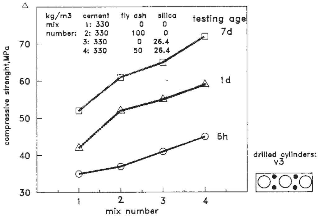
Figure 8. The effect of silica fume and fly ash on the compressive strength of no-slump concrete.
