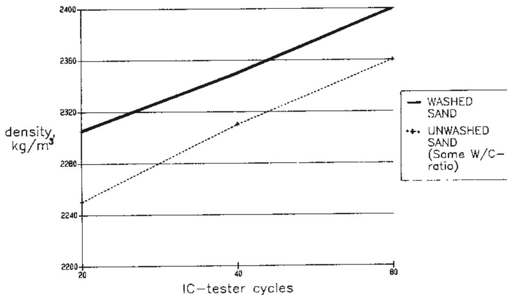
Figure 3. The effect of washed aggregate on the workability of no-s slump concrete, measured by IC tester.
