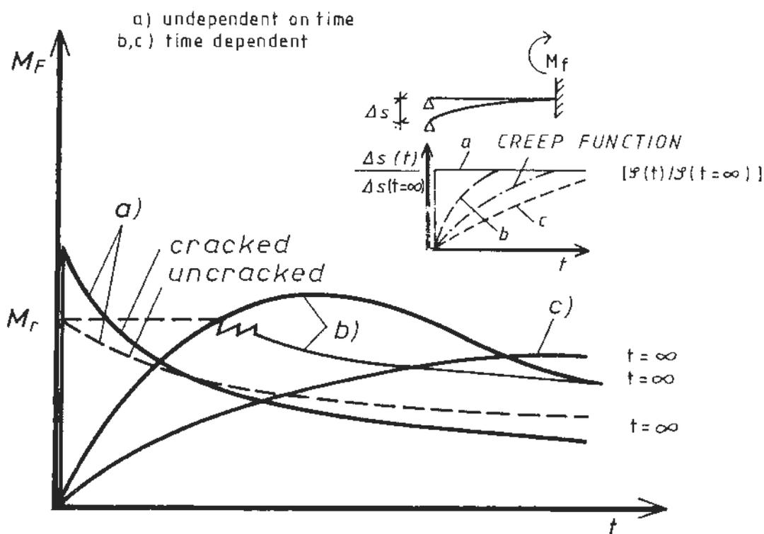
Fig. 1. Influence of the rate of restraint stress development on creep /8/.
