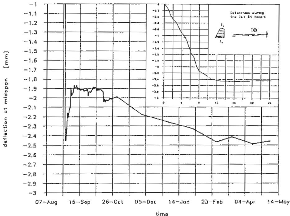
Fig. 5. Deflection at the midspan of the heated beam 1a.
