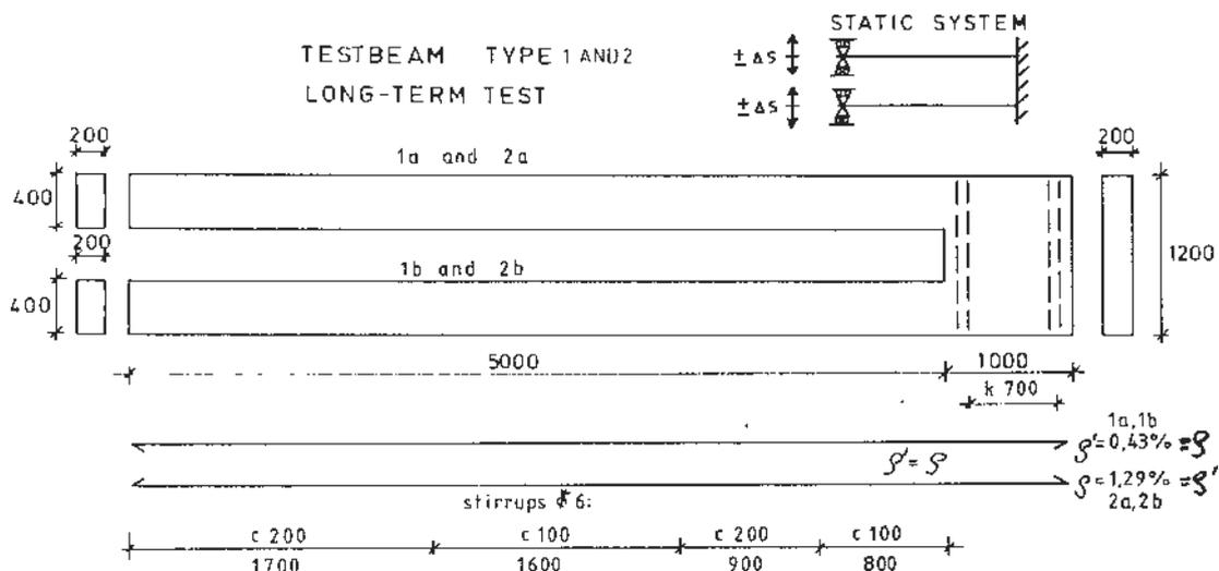
Fig 2. Dimensions and structure of the test beams.
