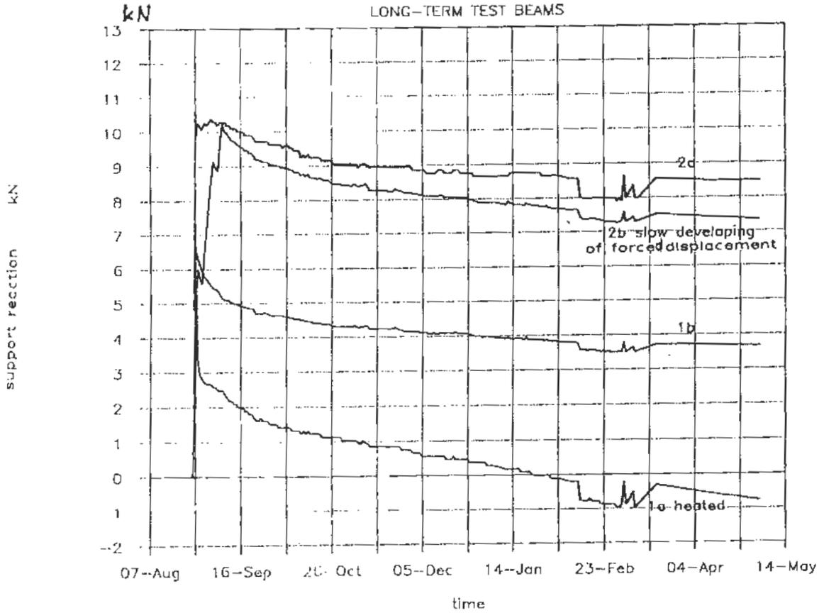
Fig. 6. Support reaction values (including own weight) in the free end of all beam during the first eight months.
