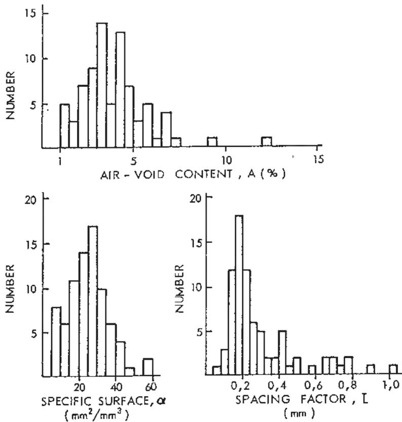
Fig 3. Air-void characteristics of specimens tested.
