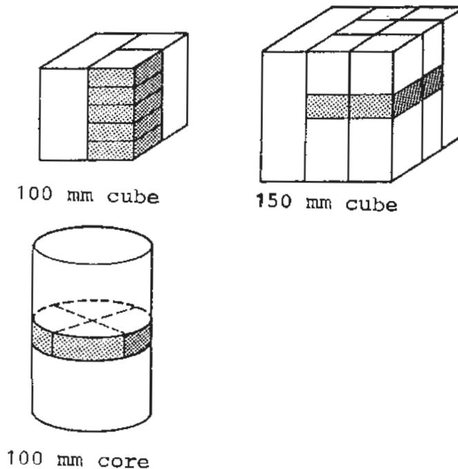
Fig 2. Cutting of specimens.
