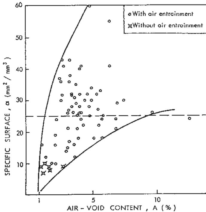
Fig 4. Specific surface versus air-void content.
