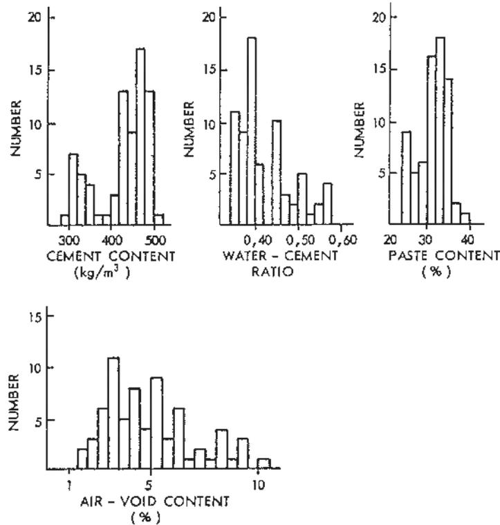
Fig 1. Data on fresh concrete for the specimens tested.
