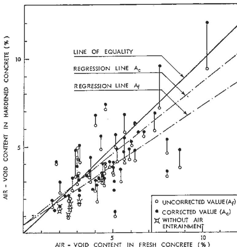
Fig 7. Air-void content in fresh versus hardened concrete.
