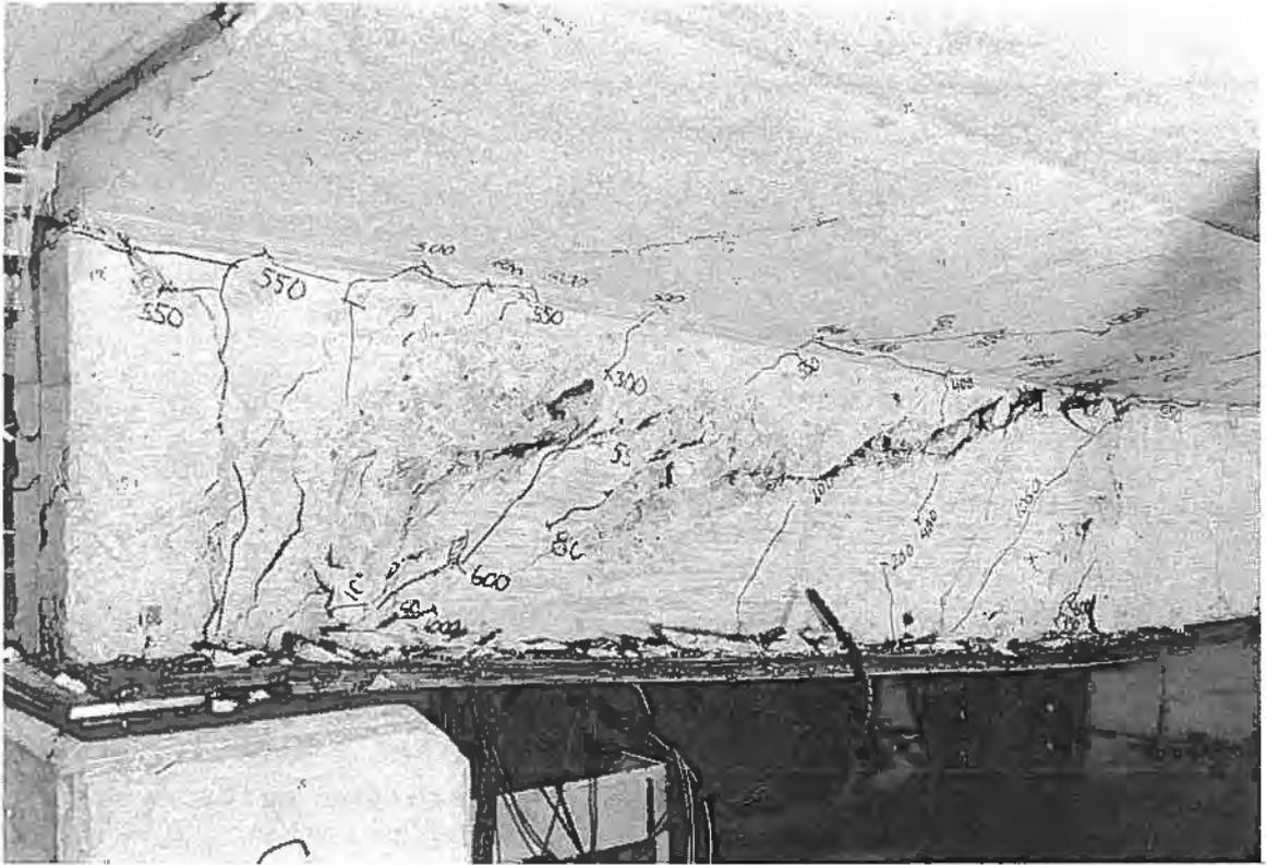
Fig. 8 Beam end C after failure.
