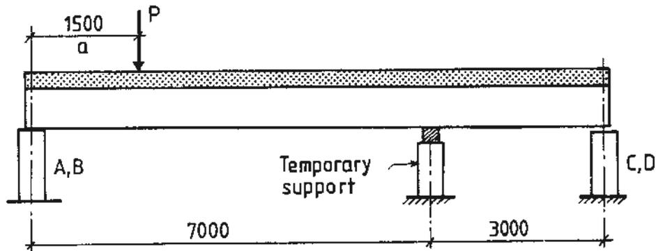
Fig. 3 Loading arrangements at shear tests.
