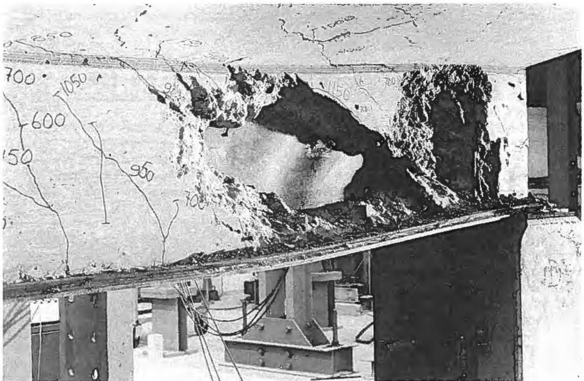
Fig. 9 Beam end D after failure.
