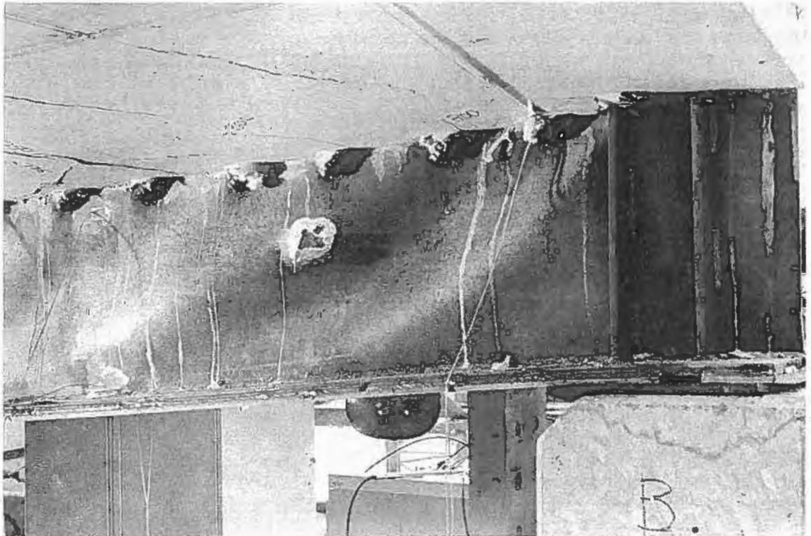
Fig. 7 Beam end B after failure.
