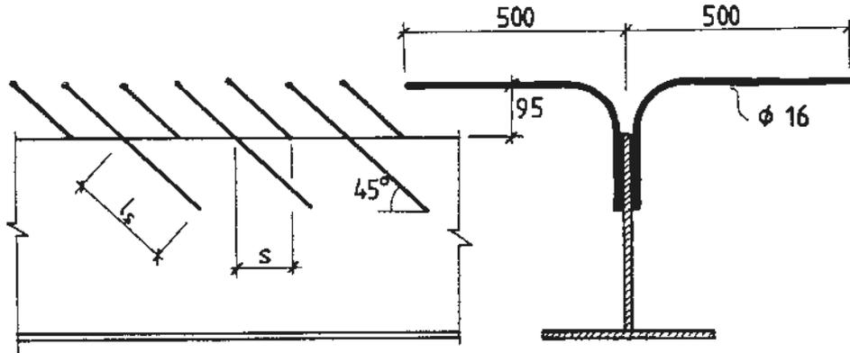
Fig. 2 The design of the shear transfer reinforcement.
