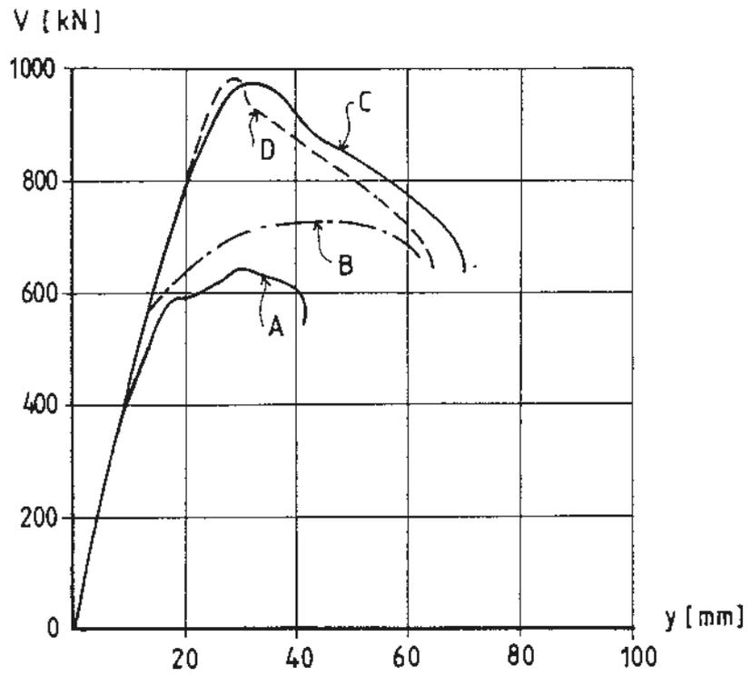
Fig. 4 Load deflection diagrams for the shear tests A, B, C and D.
