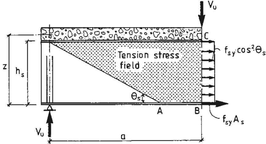
Fig. 10 Model for the ultimate shear capacity of the naked steel web.
