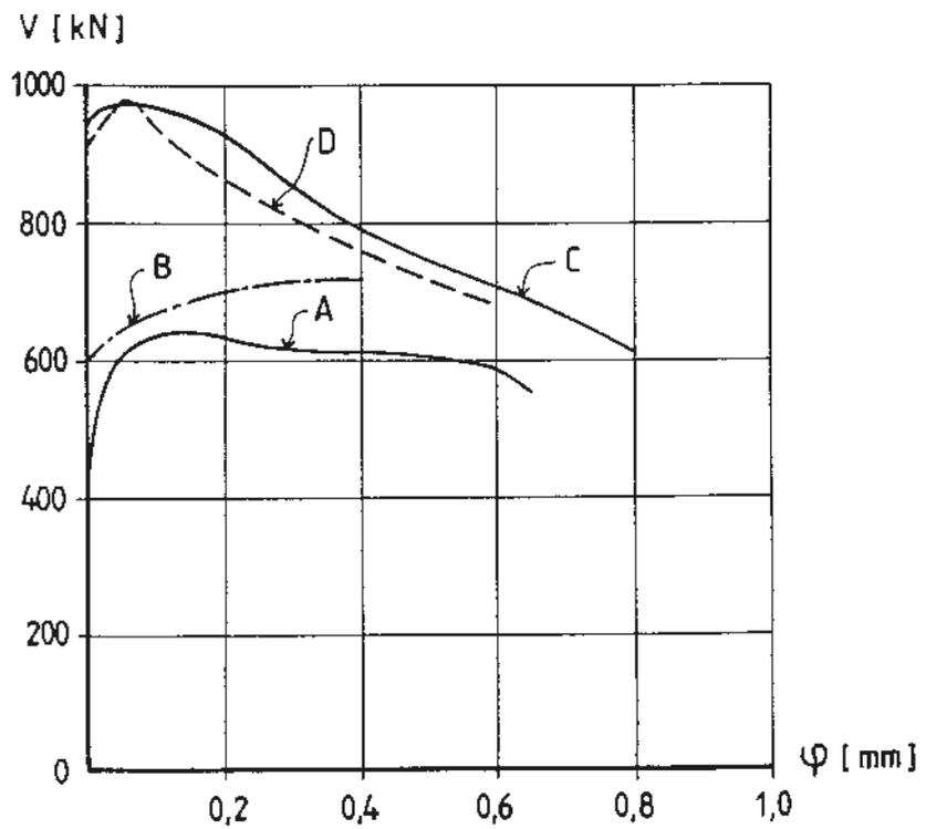
Fig. 5 Load slip relation for the shear tests A, B, C and D.
