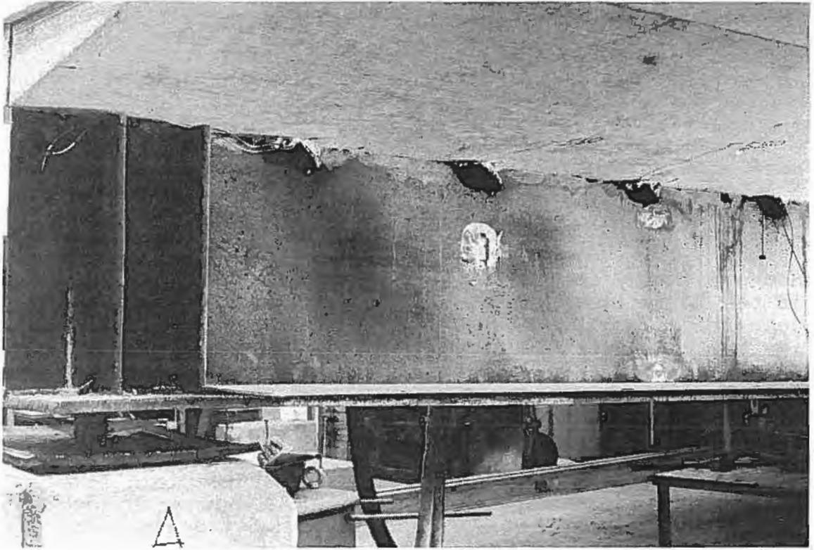
Fig. 6 Beam end A after failure.
