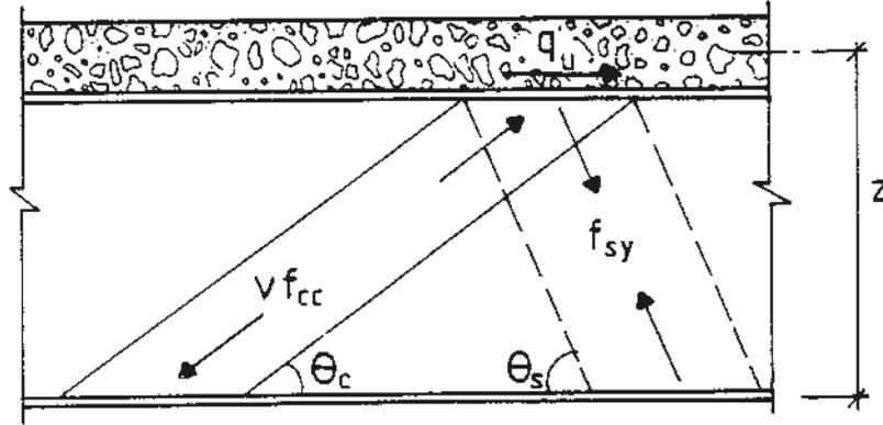
Fig. 11 Model for the shear capacity of the composite web.
