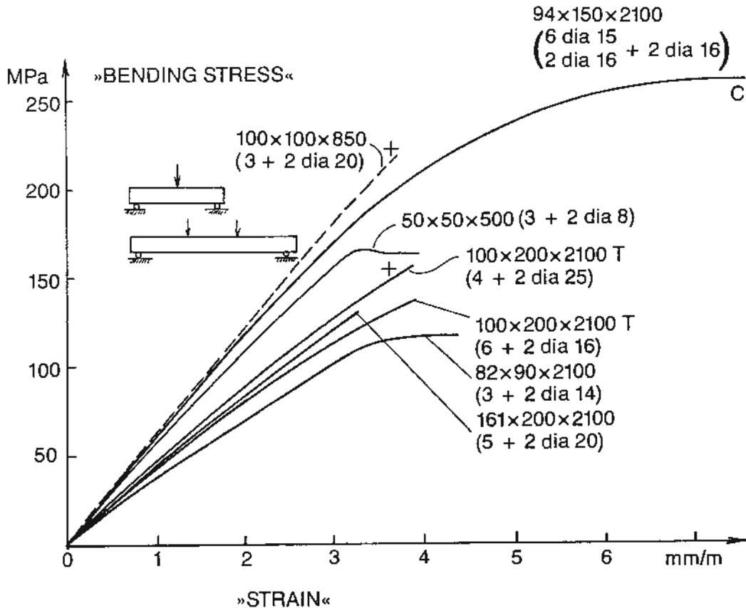
FIG. 8. Bending behaviour of six different types of CRC-beams, expressed by formal bending stresses and formal maximum tensile strains.
