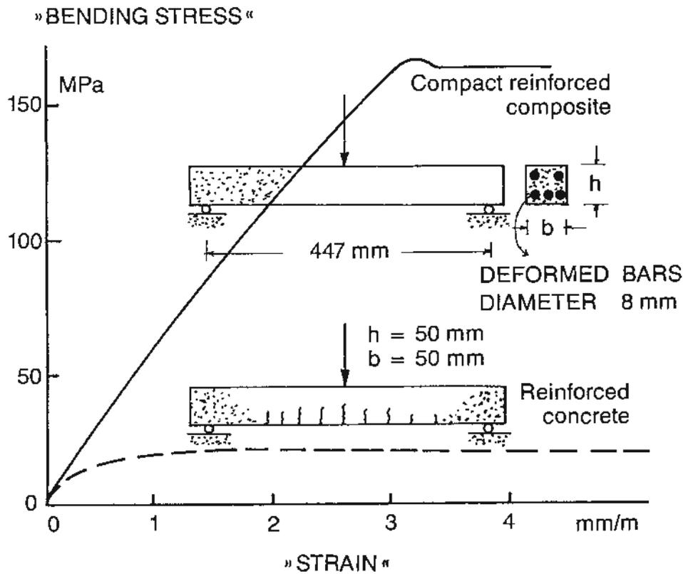
FIG. 3. Behaviour of CRC-beam (plate strip) in bending.
