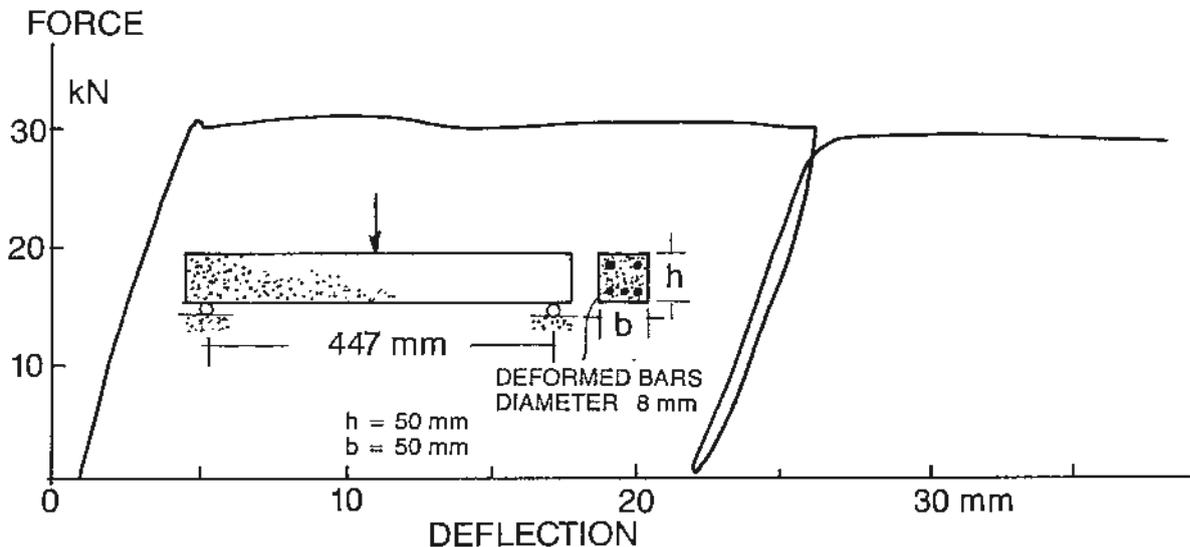
FIG. 7. Behaviour of a CRC beam (plate strip) in bending. After a pronounced yielding at a deflection of about 25 mm the load was released whereafter the beam was reloaded. The first part of the curve is shown in normalized form in FIG. 3.
