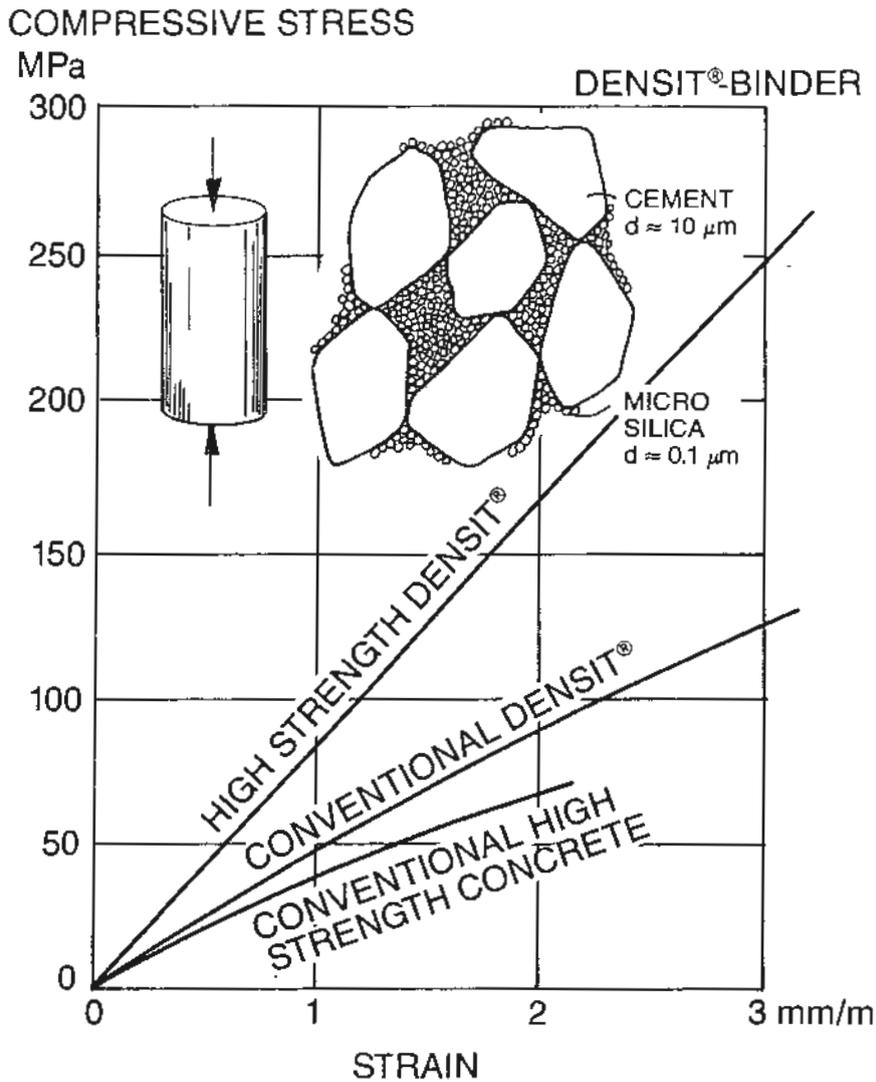
FIG. 1. Behaviour of Densit<sup>0</sup>-materials and conventional high-strength concrete under compression. The high-strength Densit<sup>0</sup>-materials are made with strong Al<sub>2</sub>O<sub>3</sub>-rich aggregates (calcinated bauxite). The Densit<sup>0</sup>-binder is formed from a structure built up of densely packed cement with microsilica placed in the spaces between the cement particles /1/.
