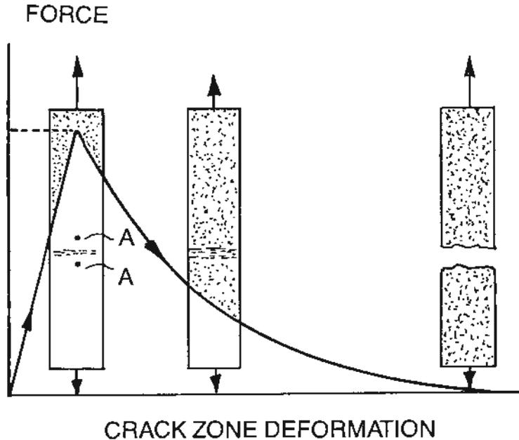
FIG. 4. Tensile failure in brittle materials occurs through the development of a single crack. The cracking is accompanied by a small deformation in the zone around the later separation face (A-A) after maximum loading has been reached. The magnitude of this "crack zone deformation" is about 20  $\mu\text{m}$  for concrete, 5  $\mu\text{m}$  for cement paste, 1  $\mu\text{m}$  for Densit<sup>0</sup>-paste, and 0.01  $\mu\text{m}$  for glass.
