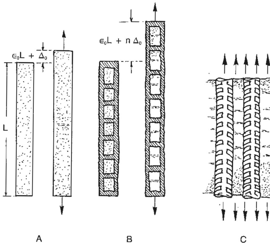
FIG. 6. Tensile deformation of a bar of a ceramic material (A) and an identical bar divided into small bodies fixed to a stiff frame that undergoes tensile deformation (B).
