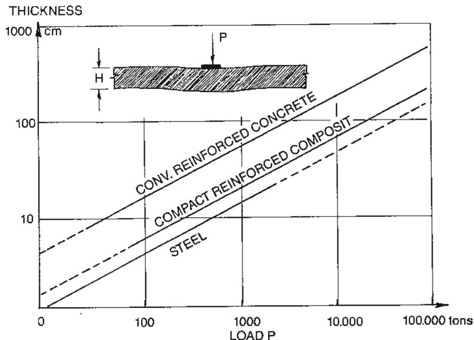
FIG. 10. Critical thickness of large plates loaded with a concentrated force.
