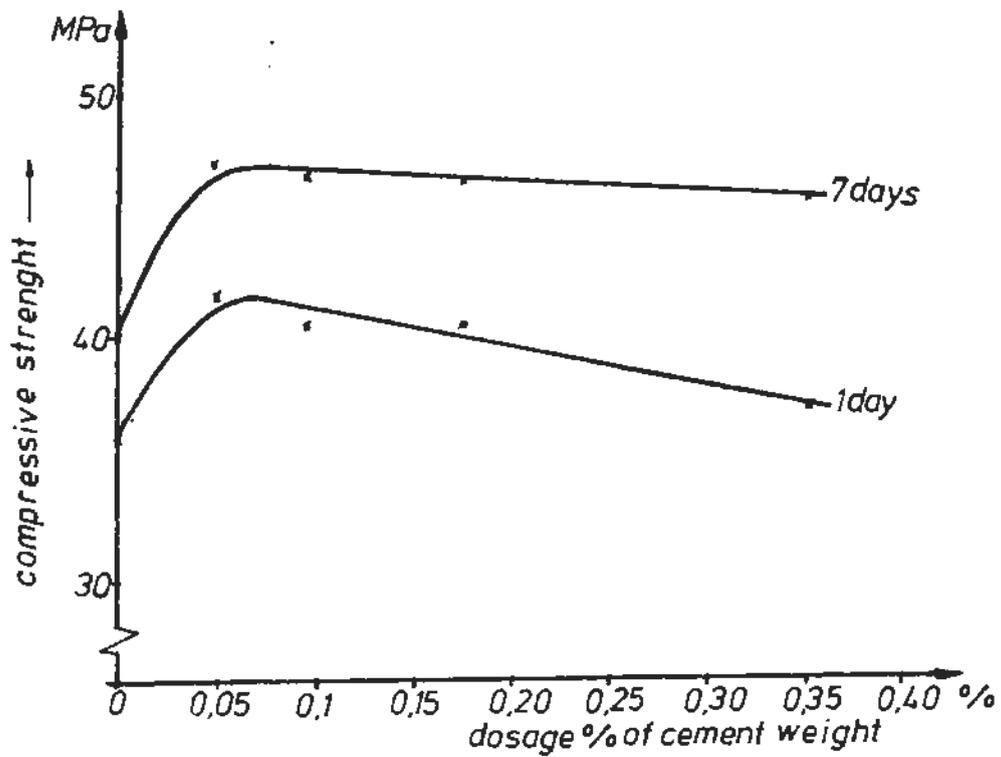
Fig. 4 Concrete strength depending on admixture dosage
