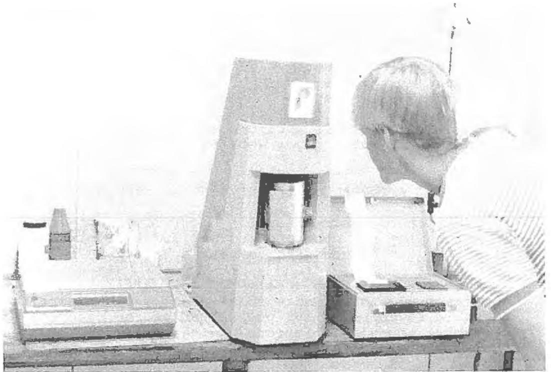
Photo 2 Device compacts concrete sample and simultaneously takes density readings. The control unit gives a print out of density readings.
