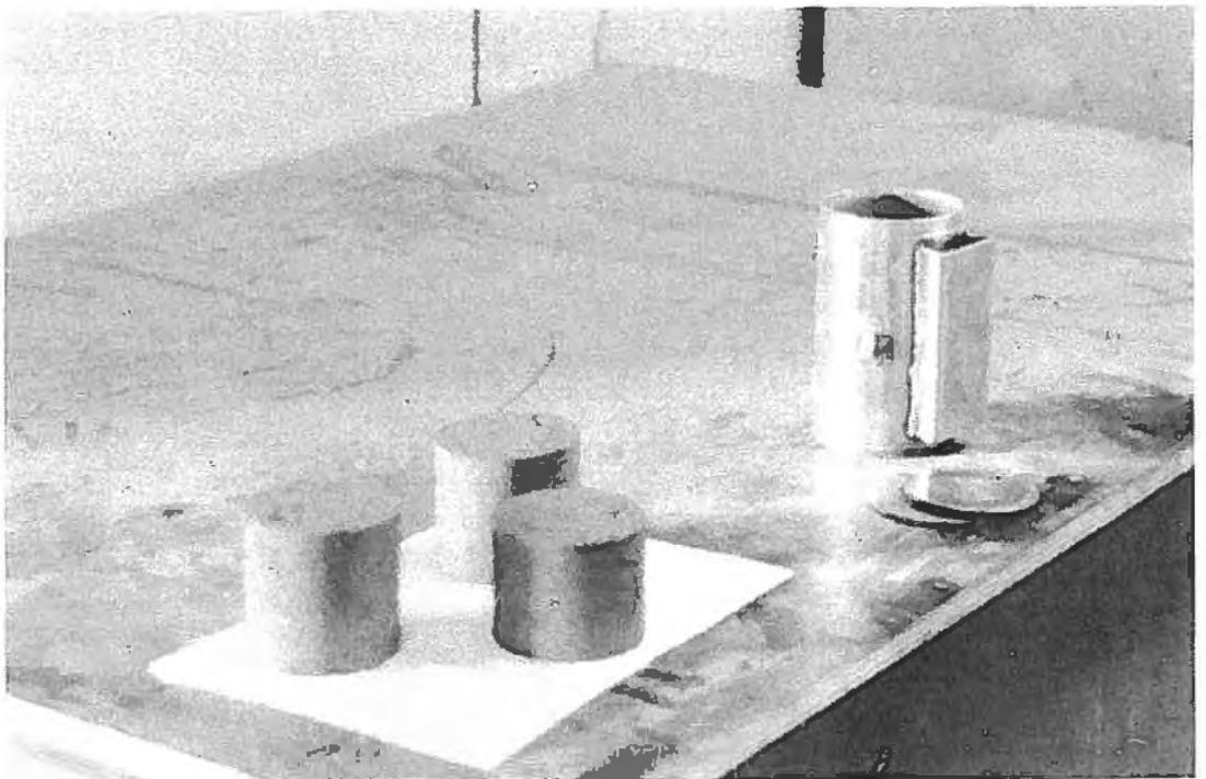
Photo 3 Compacted concrete samples and the work cylinder behind. If desired, the structure of test samples can be examined and they can be subjected to strength tests.
