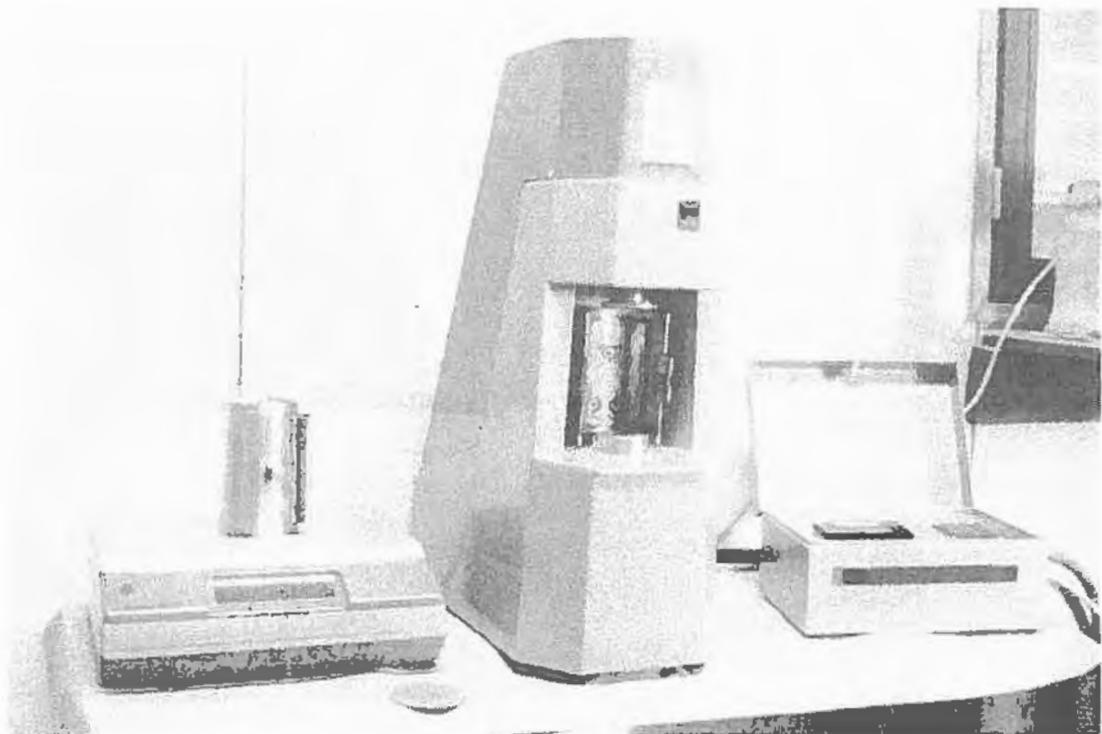
Photo 1 Testing device in centre, control and output unit on the right. The scale on the left can also be connected direct to the control unit. On top of the scale is the work cylinder in which the concrete sample is weighed.
