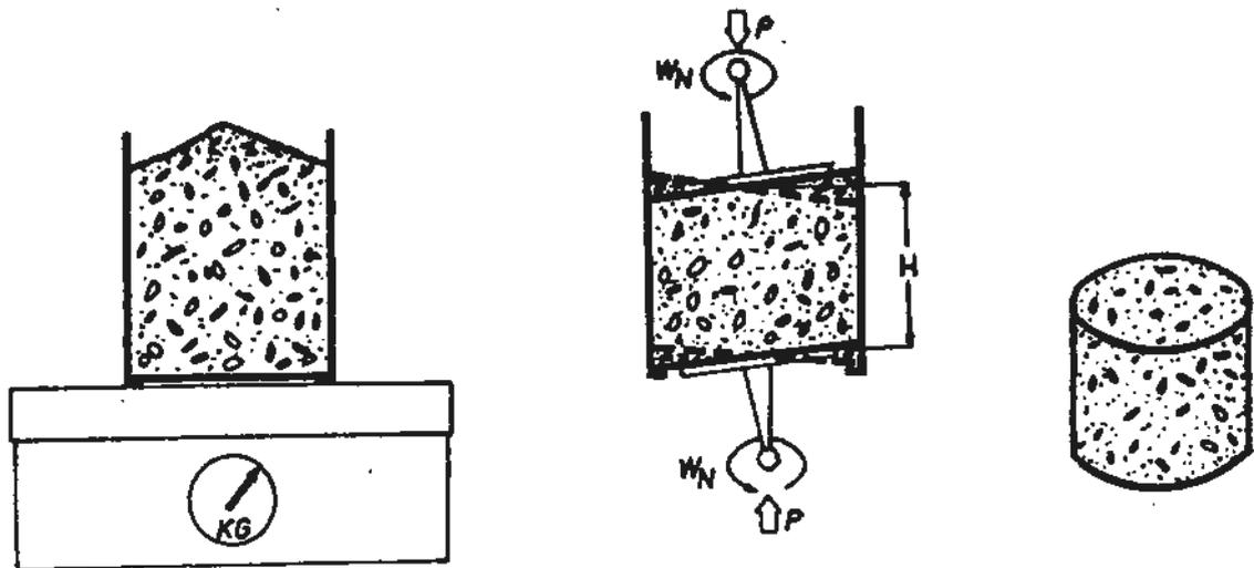
a) Weighing of the concrete sample in the work cylinder.
