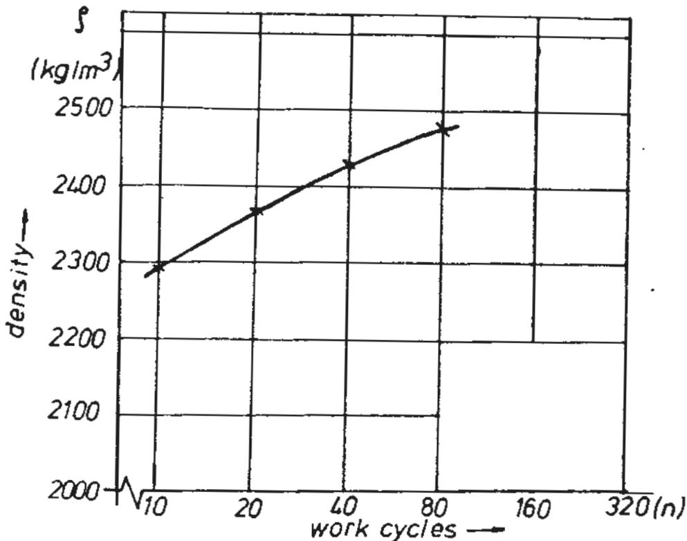
Fig. 2 Test report and compacting diagram
