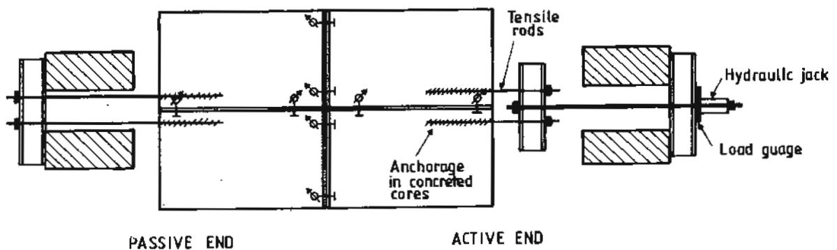
Fig. 3 Load arrangement and instrumentation
