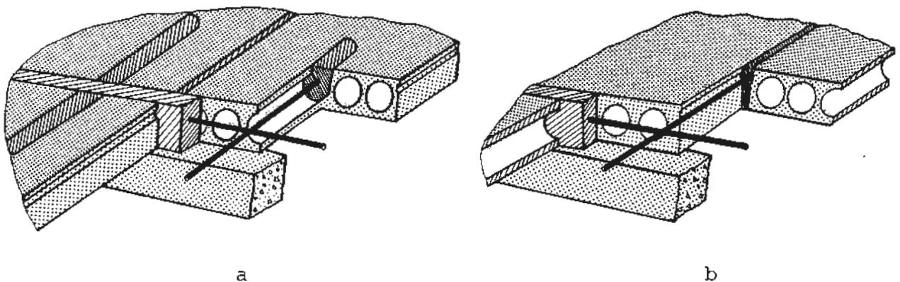
Fig. 1 Typical solutions for the connection at an internal support
