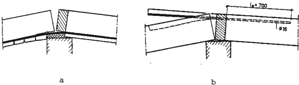
Fig. 10 Anchorage failures of the longitudinal tie bar
