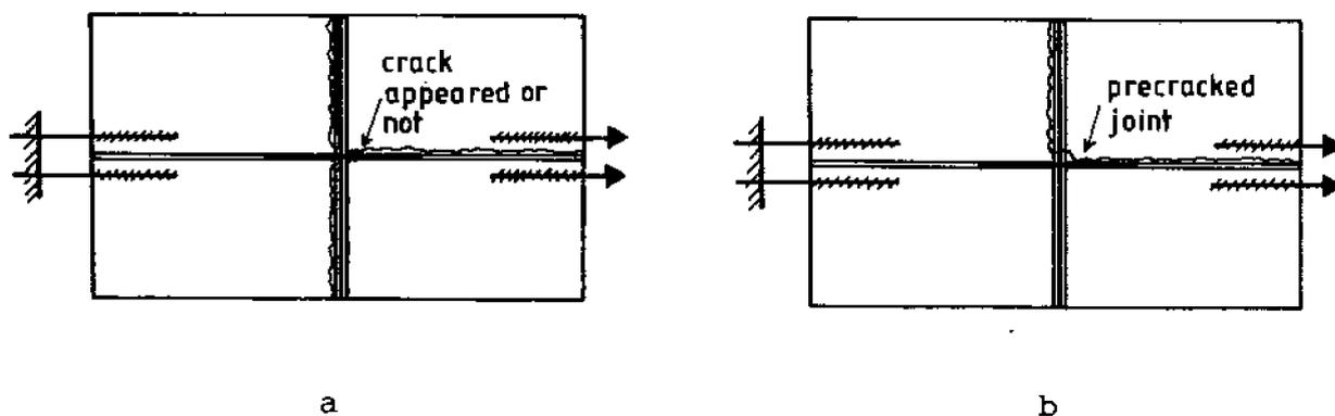
Fig. 5 Alternative ruptures in the transverse joint
