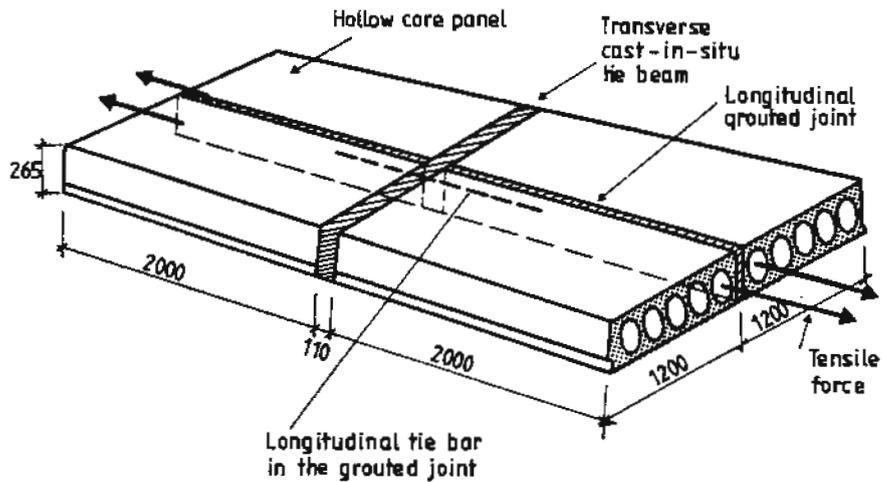
Fig. 2 Test specimen and load arrangement
