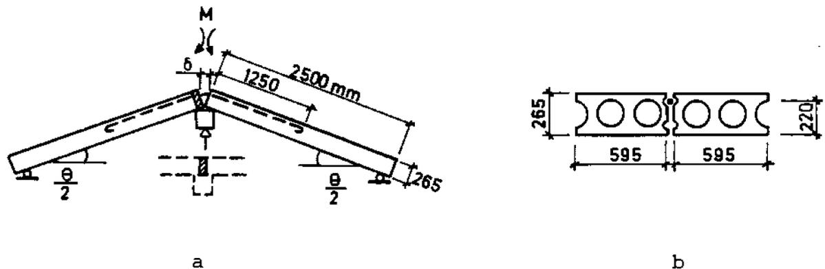
Fig. 9 The test specimen and load arrangement
