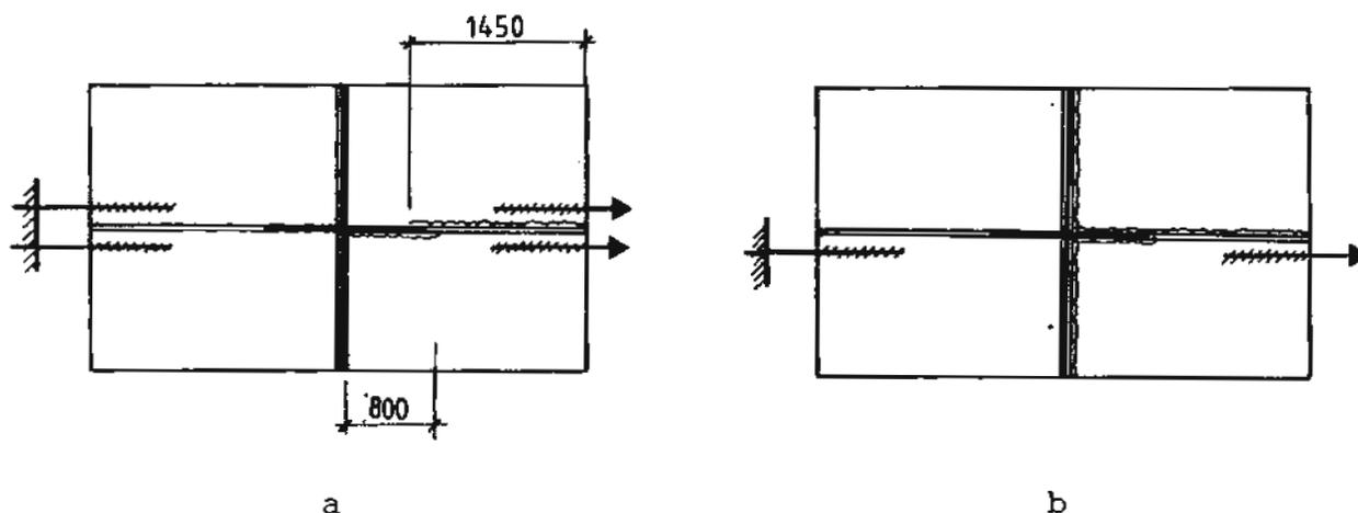
Fig. 8 Crack formation in test no. 8
