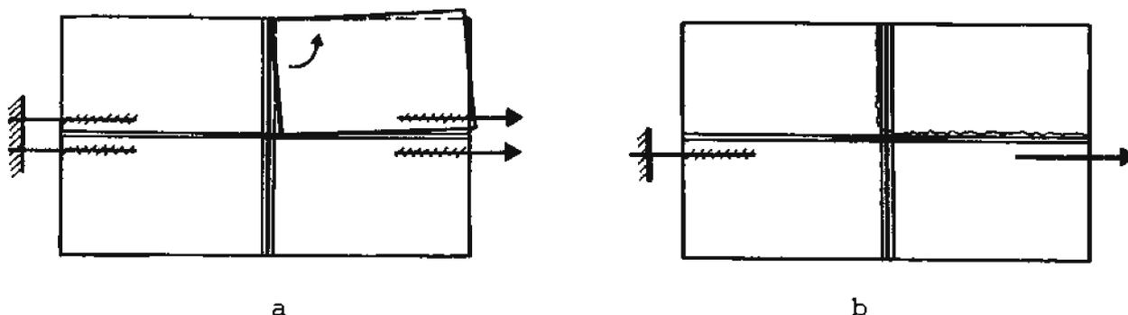
Fig. 6 Test specimen with precracked longitudinal joint
