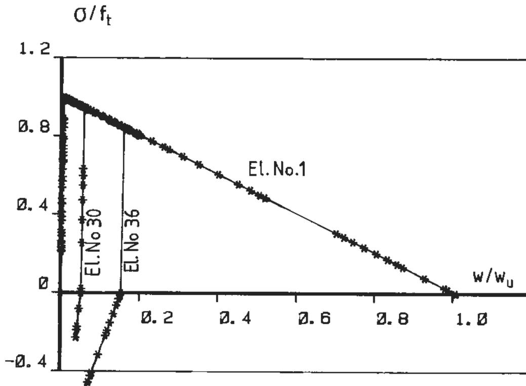
Fig. 5.6 Relative  $\sigma$ - $w$  curve from three different crack elements in the "large bar spacing" geometry
