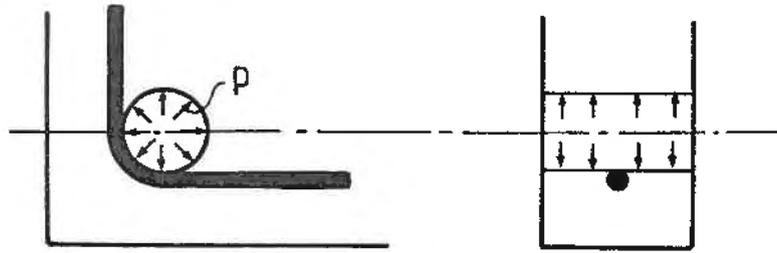
Fig. 4.1 Test specimen to study anchorage splitting
