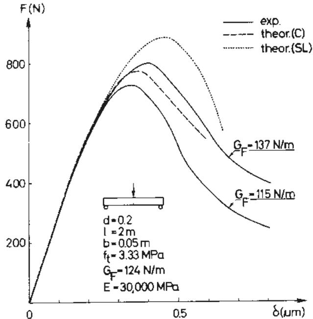
Fig. 2.5 Experimental and theoretical load-deflection curves for three-point bend tests on notched beams. (SL) is the straight line model. (C) is the bilinear model /5/
