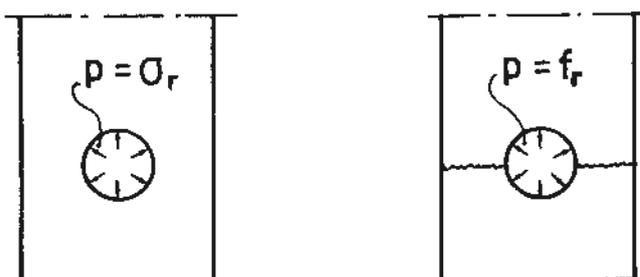
Fig. 2.1 Principle for splitting failure in a concrete cross section loaded with an internal pressure
