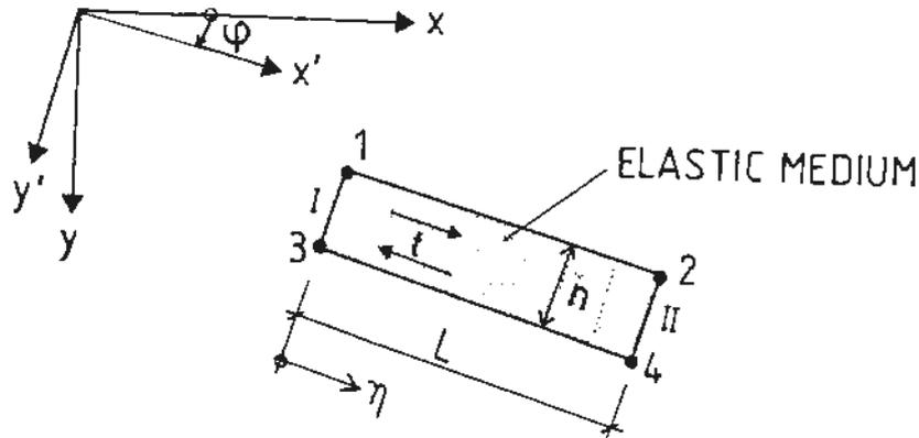
Fig. 3.1 Four node crack element
