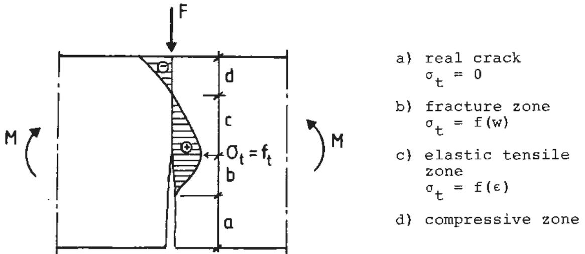
Fig. 2.2 Stress distribution at crack propagation according to FCM
