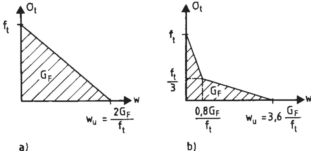
Fig. 2.4 Approximations of the  $\sigma$ - $w$  curve for plain concrete. b) is proposed by Pettersson, /5/ based on direct tensile tests .
