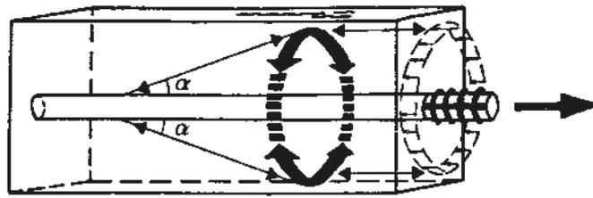
Fig. 1.2 "Schematic representation of how the radial components of the bond forces are balanced against tensile stress rings in the concrete in an anchorage zone", from /2/
