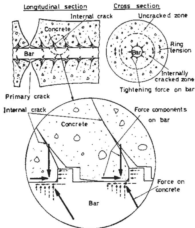
Fig. 1.1 Forces and internal cracking around a deformed bar, fig. from /1/
