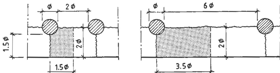
Fig. 5.1 The two geometries being analysed.  $\phi = 16$  mm. Due to symmetry, only the dotted part of the cover is modelled
