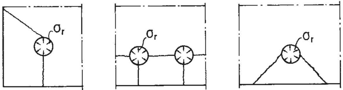
Fig. 1.3 Examples of different possible crack patterns at anchorage failure due to splitting (splitting failure)
