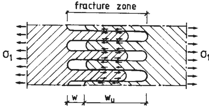
Fig. 2.6 Phenomenological, "slip friction" hypothesis to explain the strain softening in the fracture zone
