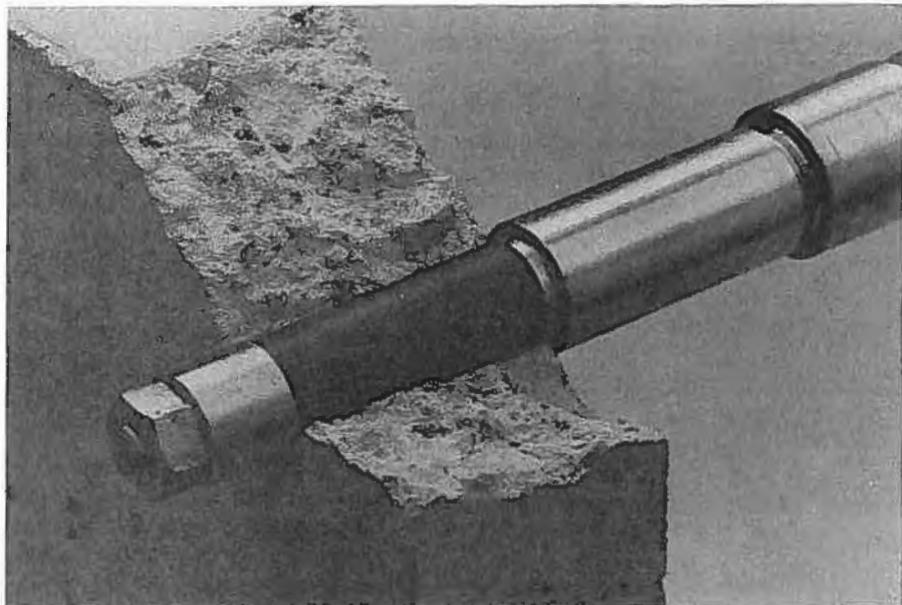
Fig. 4.2 A testing method to simulate anchorage splitting caused by a deformed bar
