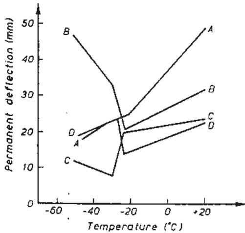
Fig. 5. Permanent deflections of reinforced beams prior to failure of the steels.
