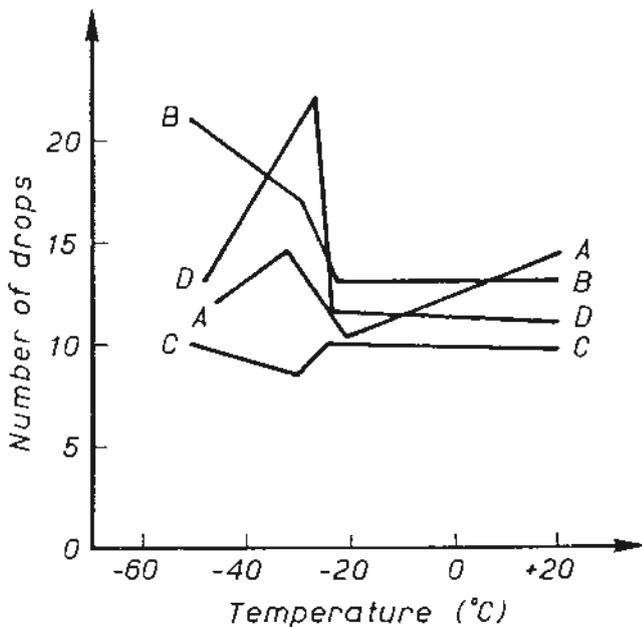
Fig. 2. Number of drops required to break the tension steel of beams.
