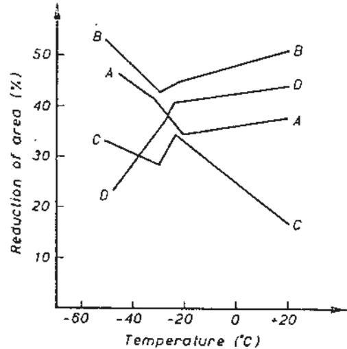
Fig. 6. Reduction in area of tension steels following their failure in the beams.
