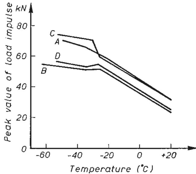
Fig. 4. Load required for occurrence of the first cracks in reinforced beams.
