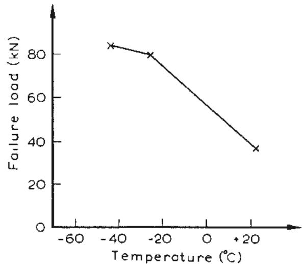
Fig. 3. Impact strength of unreinforced beams.
