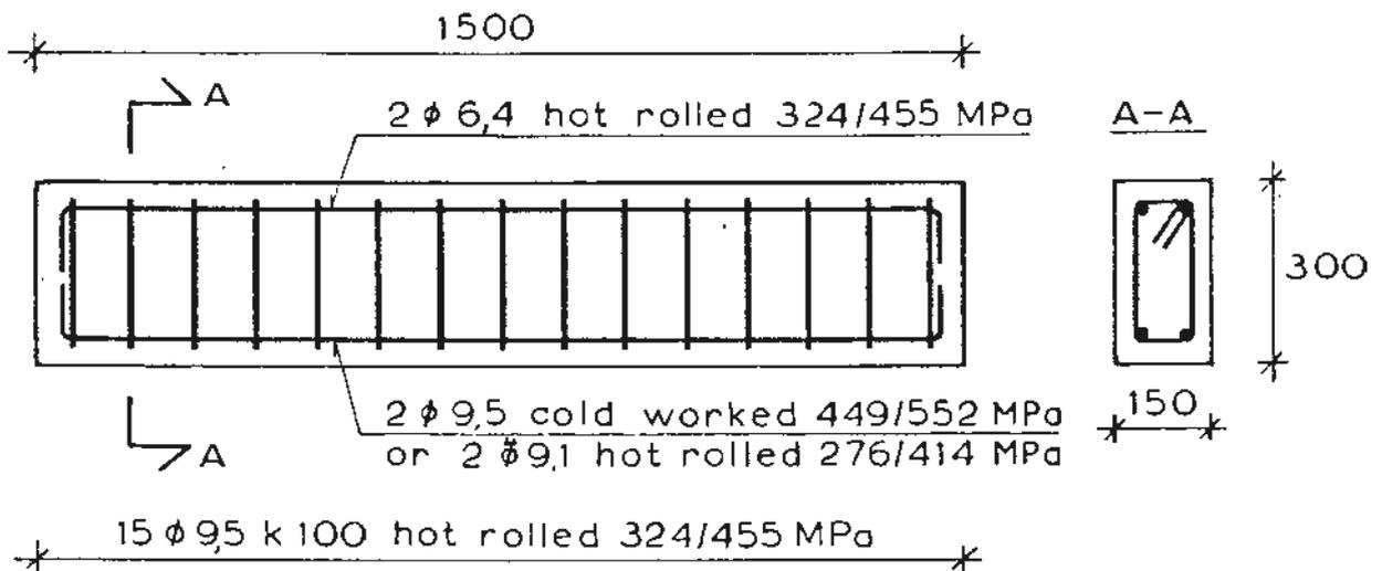
Fig. 1. Beam reinforcement pattern.
