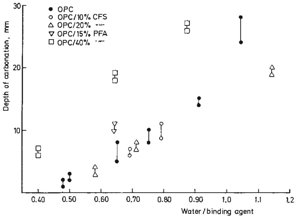
FIG 5. Measured minimum and maximum depth of carbonation for concrete stored for 2 1/2 years outdoors (sheltered from rain).
