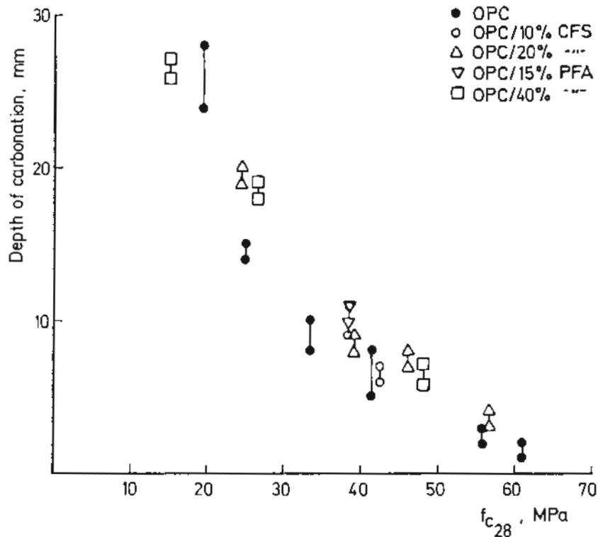
FIG 6. Measured minimum and maximum depth of carbonation for concrete stored 2 1/2 years outdoors (sheltered from rain) versus compressive strength after 28 days.
