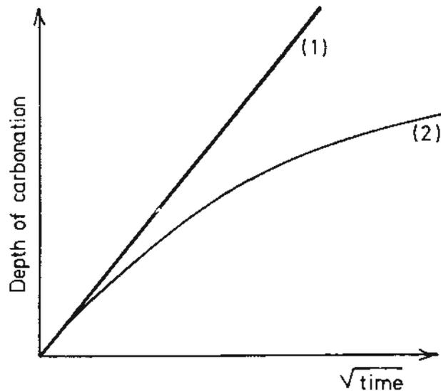
FIG 1. Two principles for describing the penetration of the carbonation front in concrete.
