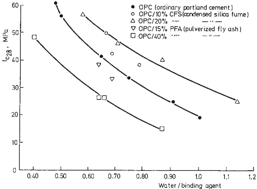
FIG 2. Compressive strength after 28 days. (7 days watercured) versus waterbindingagentratio for portland cement concrete, silica fume concrete and fly ash concrete.
