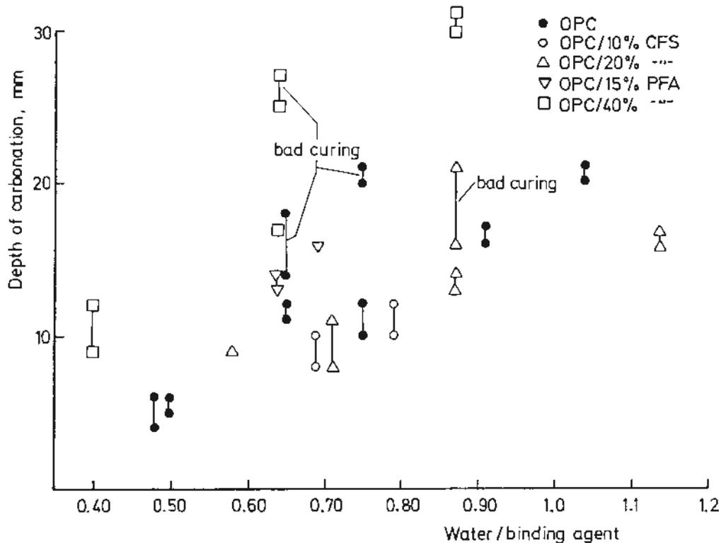
FIG 3. Measured minimum and maximum depth of carbonation for concrete stored for 2 1/2 years in 50% RH.
