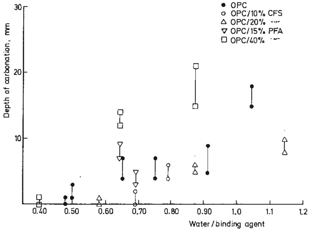
FIG 4. Measured minimum and maximum depth of carbonation for concrete stored for 2 1/2 years in 80% RH.
