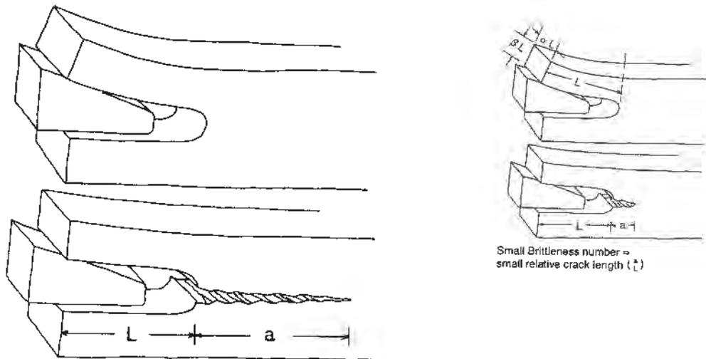
Fig. 10. Instability after crack initiation, illustrated by the size of the instantaneous crack.
