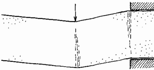
Fig. 4. Yield plane theory. In tensile yielding the body is displaced as rigid bodies separated by narrow yield zones.
