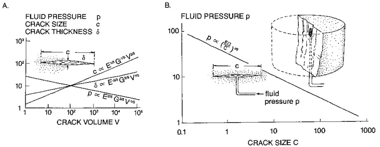
Fig. 9. Crack propagation in large objects caused by fluid expansion in the crack. The propagation is stable for strain-loaded systems, where the volume increases slowly (A), and unstable for stress-loaded systems, where the fluid pressure increases (B). The curves refer to systems with high Brittleness Numbers calculated according to LFEM.(1)(5)
