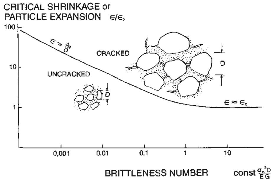
Fig. 7. Critical expansion of particles or shrinkage of matrix material in a composite with rigid particles as a function of the Brittleness Number.  $\epsilon$  is the strain, D the particle size,  $\sigma_0$  the tensile strength, E the modulus of elasticity, G the fracture energy, and  $\Delta_0$  the crack deformation, all referring to the matrix material.
