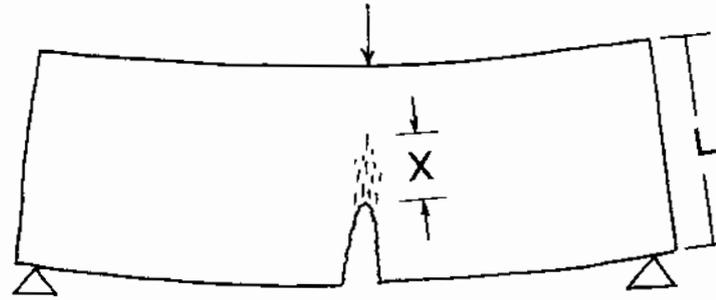
Fig. 5. Non-linear fracture mechanics is typically used when the length of the crack zone  $x$  is not small in relation to the size of the object  $L$ .
