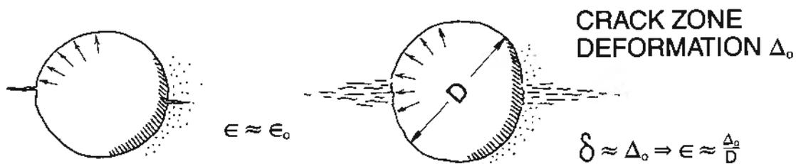
Fig. 6. Crack initiation by expansion of body in elastic solid.
