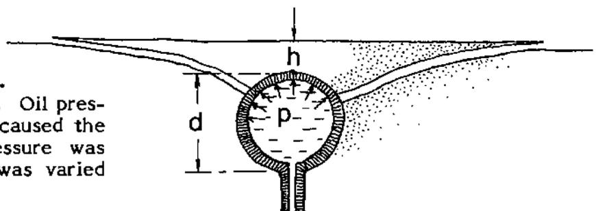
Fig. 11. Creation of pop-outs. Model test on cement mortar. Oil pressure in 30 mm rubber balls caused the pop-outs. The pop-out pressure was measured and the depth h was varied between 2.4 and 30 mm. (4)
