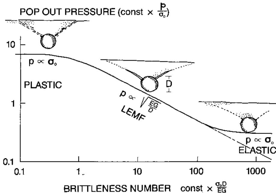
Fig. 12. Pop-out pressure as a function of the Brittleness Number. Master curve for geometrically similar systems (sketch). The sketches illustrate the situation just before rupture.
