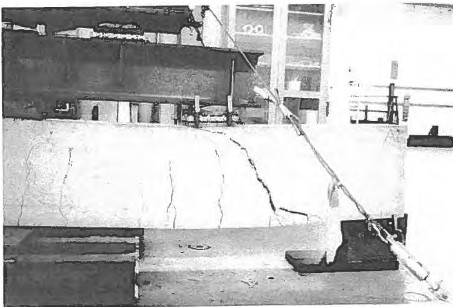
Photo 2. Shear failure in a non shear reinforced part of a beam.
