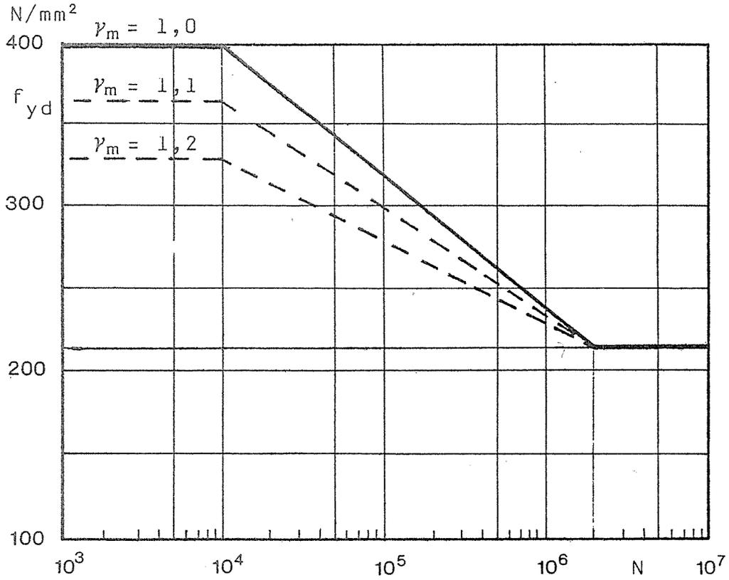
FIG 4 Simplified Wöhler diagram for the design fatigue strength of Finnish reinforcing steel
