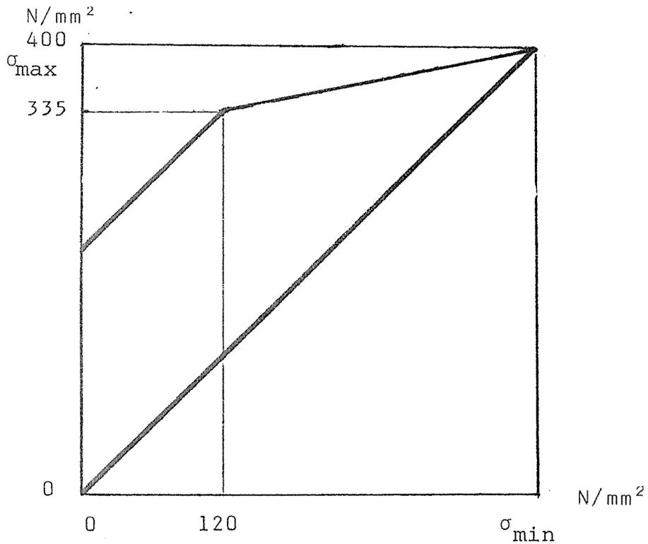
FIG 5 Simplified modified Goodman diagram for the design fatigue strength in figure 4
