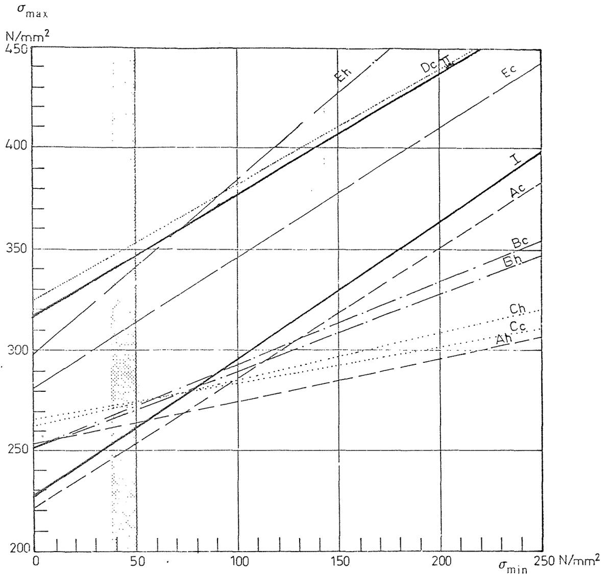
Symbols A, B, C, D, E, I and II are described in figure 1. Index h means hot-rolled and c cold-twisted bars.
