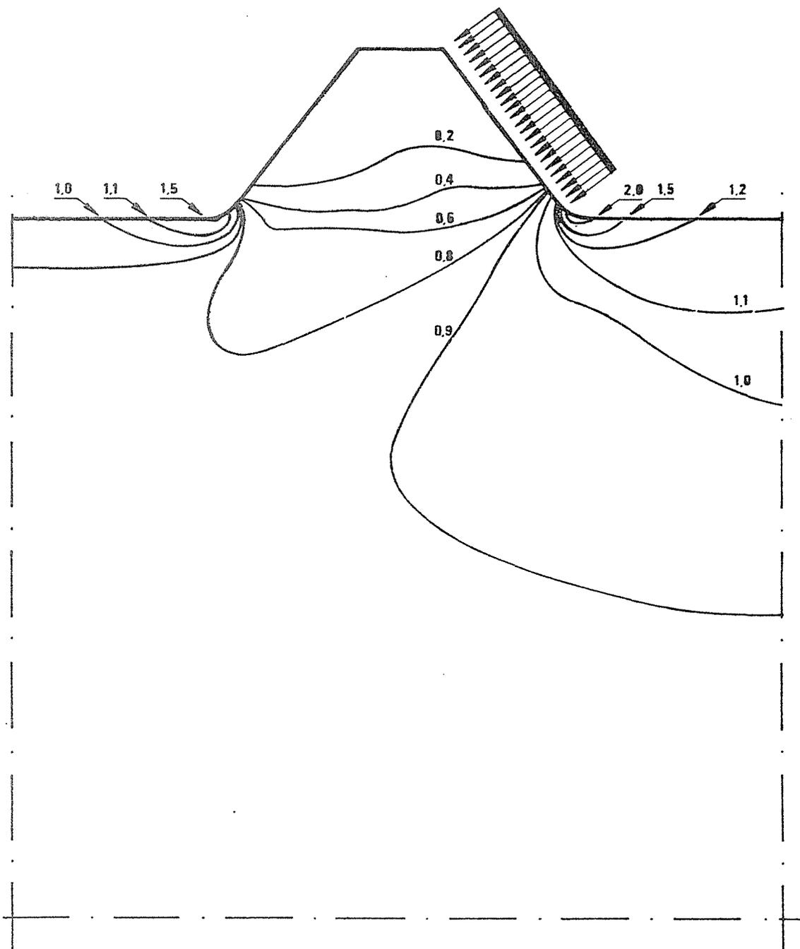
FIG 3 Contour map of ultimate stresses for an 8 mm bar embedded in concrete K 30. The average stress in steel bar is equal to unity.
